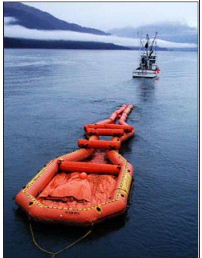
The fishing vessel Lady Sandra tows a CurrentBuster boom unit to Allison Point to practice oil-skimming operations. Photo by Stan Jones.
