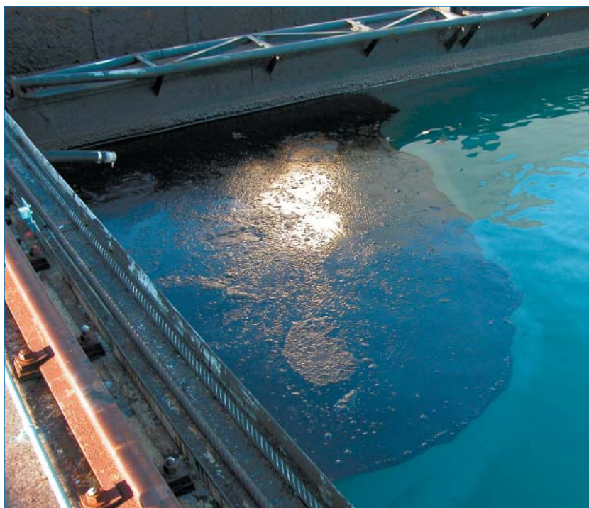
Test procedures at the OHMSETT facility fail to account properly for the resurfacing phenomenon, shown here, according to the council’s report. Photo courtesy of Merv Fingas.
