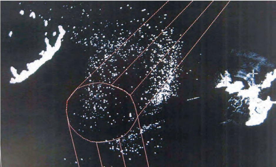
Above is an image of sea ice in tanker lanes created by the ice radar system. Dotted lines mark tanker lanes. The large white shapes indicate Bligh and Glacier Islands. Clusters of small white shapes indicate sea ice.
