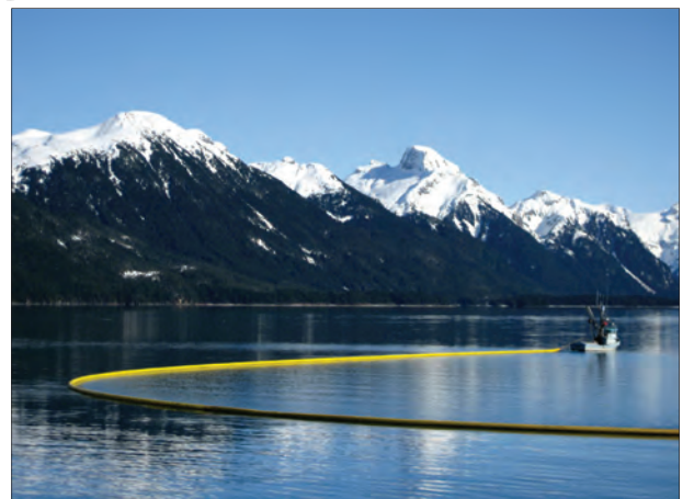
A Prince William Sound fishing vessel practices towing oil spill containment boom during a recent training session. Photo by Roy Robertson.
