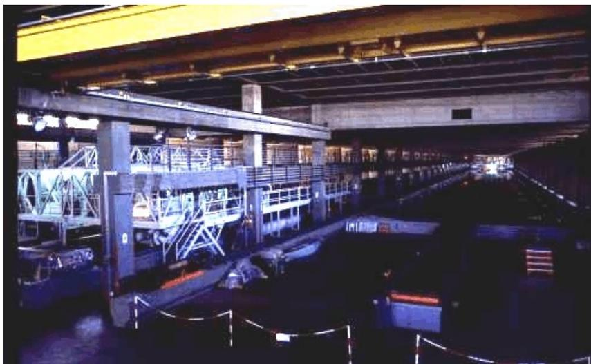
Figure 30 The tow tank at INSEAN, Italy. At 470 m, this is the longest tank of its type.
