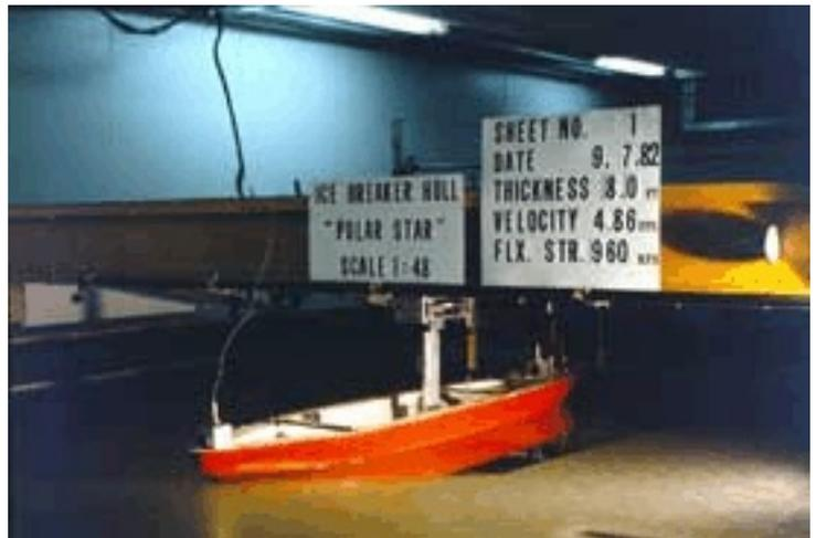
Figure 12 The Iowa ice basin and tow tank in operation
