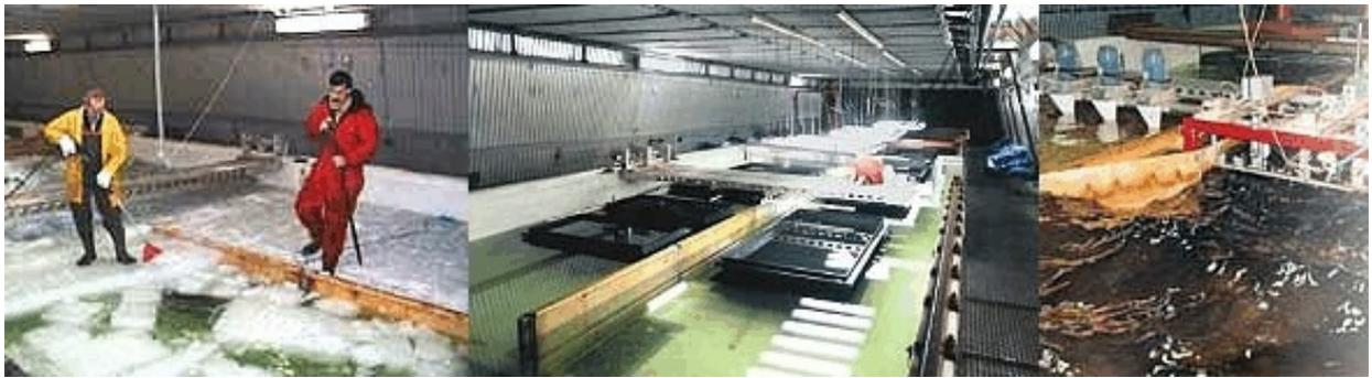
Figure 28 Montage of photographs of the Hamburg ice tank. The photo at right shows an oil skimmer being tested.
