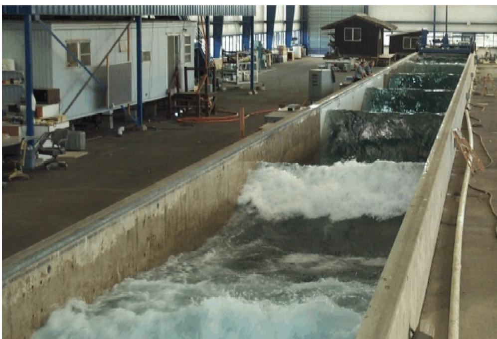
Figure 16 Oregon State large wave flume. This tank may be a candidate for dispersant testing.
