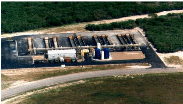
Figure 2 The SERF facility - The nine test tanks are visible at the top of the photo, the laboratory is the white building below the tanks, and the upright tanks are the oily water treatment vessels.
