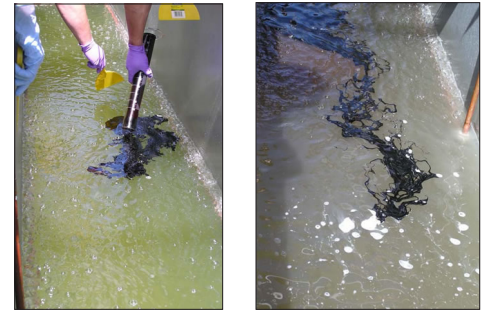
Testing the behavior of oil in water at a wave tank in Halifax.
