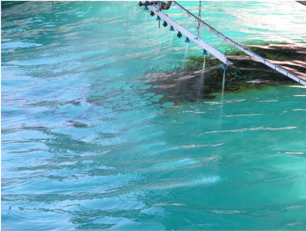
Figure 5 The Dispersant Spray System. Note that Some Herding is Occurring Here. The Width of the Spray System is about 10 Feet and the Current Oil Slick is about 5 Feet Wide
