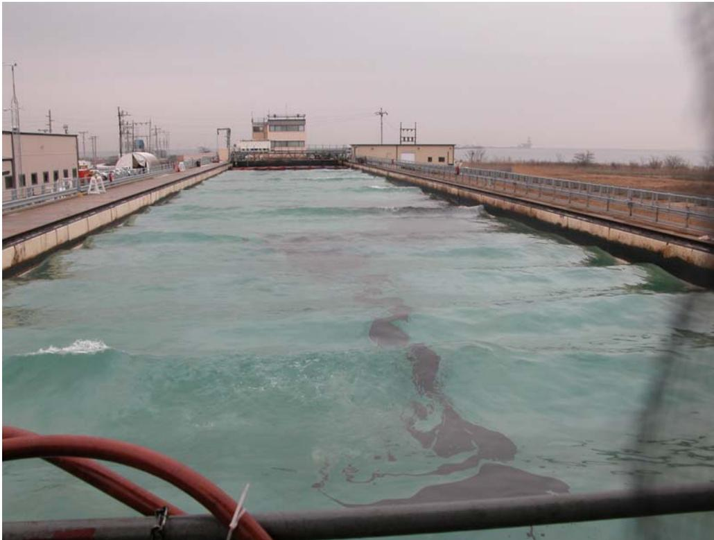
Figure 21 The Slick from Test 7 – Control Using 16% Weathered Endicott. This Photo is Right After The Slick Was Laid
