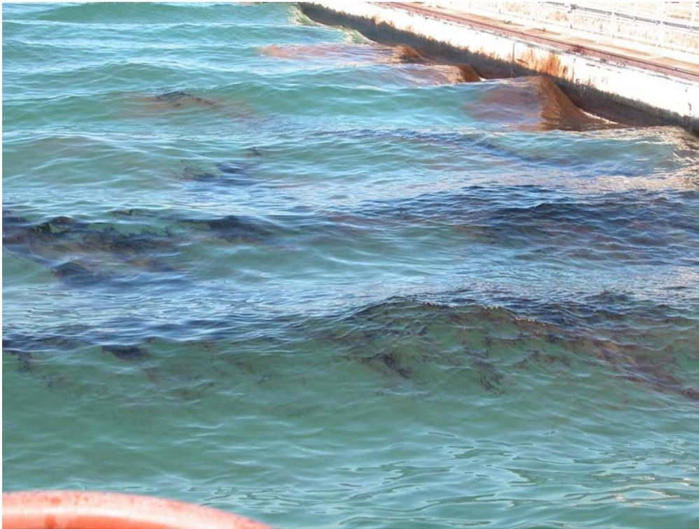
Figure 19 The Slick from Test 6 - Dispersion of 16% Weathered ANS – This is About 10 Minutes After Dispersion. Note Dispersion of Portions of the Slick and Others Which Are Not.
