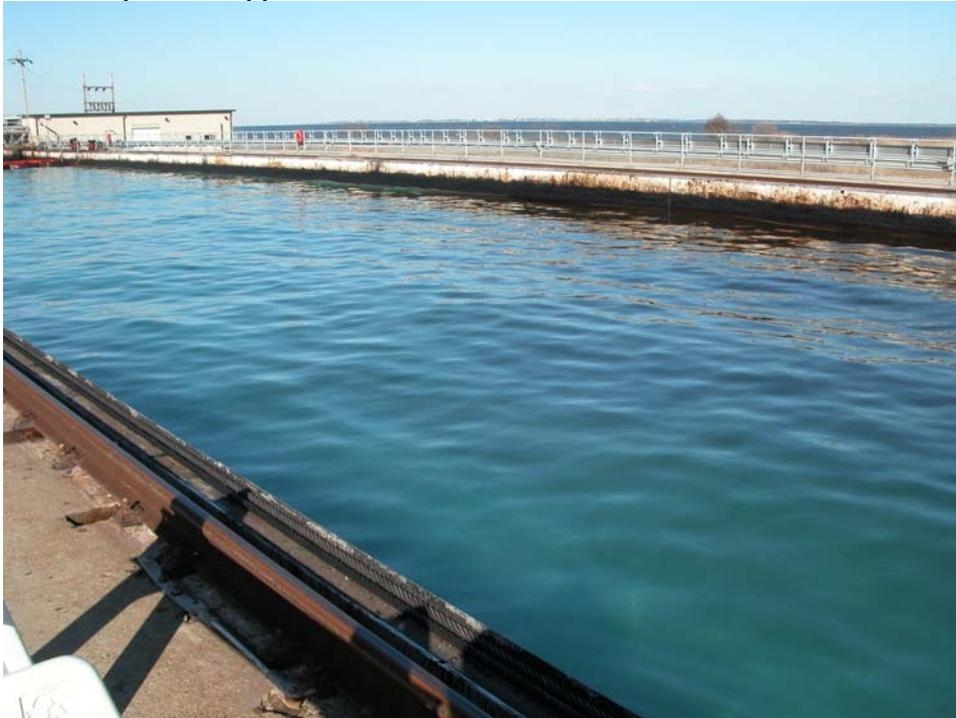
Figure 12 A View of the Tank After About 60 Minutes After Dispersant Application and About 35 Minutes After Waves Were Turned Off. Note the Thicker Black Oil Slick Resurfaced on the Opposite Wall and the Coverage of the Tank by Sheen
