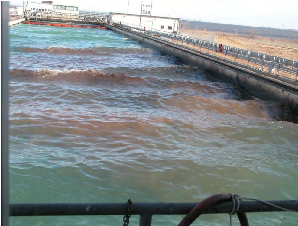
Figure 27 The Slick from Test 10 – Dispersed 15% On-Tank Weathered ANS – About 15 Minutes After Dispersion. Note that Dispersion is Relatively Wide Spread
