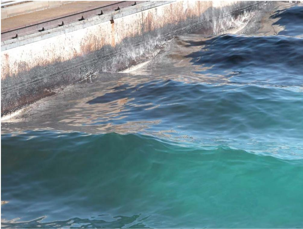
Figure 9 Test 3 – Dispersion of Fresh ANS Oil. This Picture was Taken about 8 Minutes After Dispersant Application. Dispersion is Occurring at the Edges of the Slick, Although Some Oil is Leaving as a Sheen
