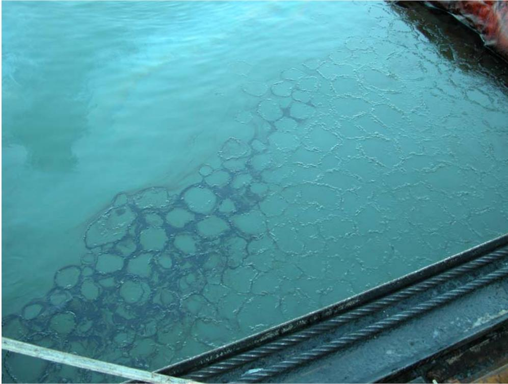
Figure 25 Resurfaced Oil From Test 9 – 15% Weather ANS – As Seen Next Morning
