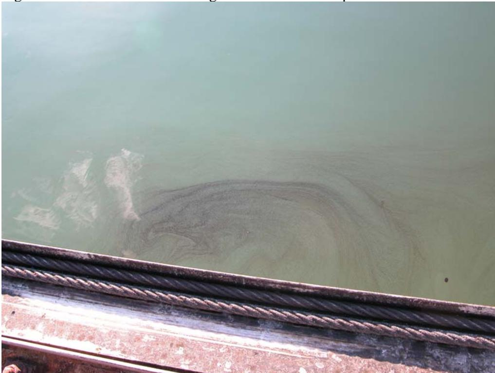
Figure 14 Oil Resurfaced Overnight from Test 3 – Dispersed Fresh ANS. Much of the Downwind Side of the Tank Was Covered with This Density of Slicks
