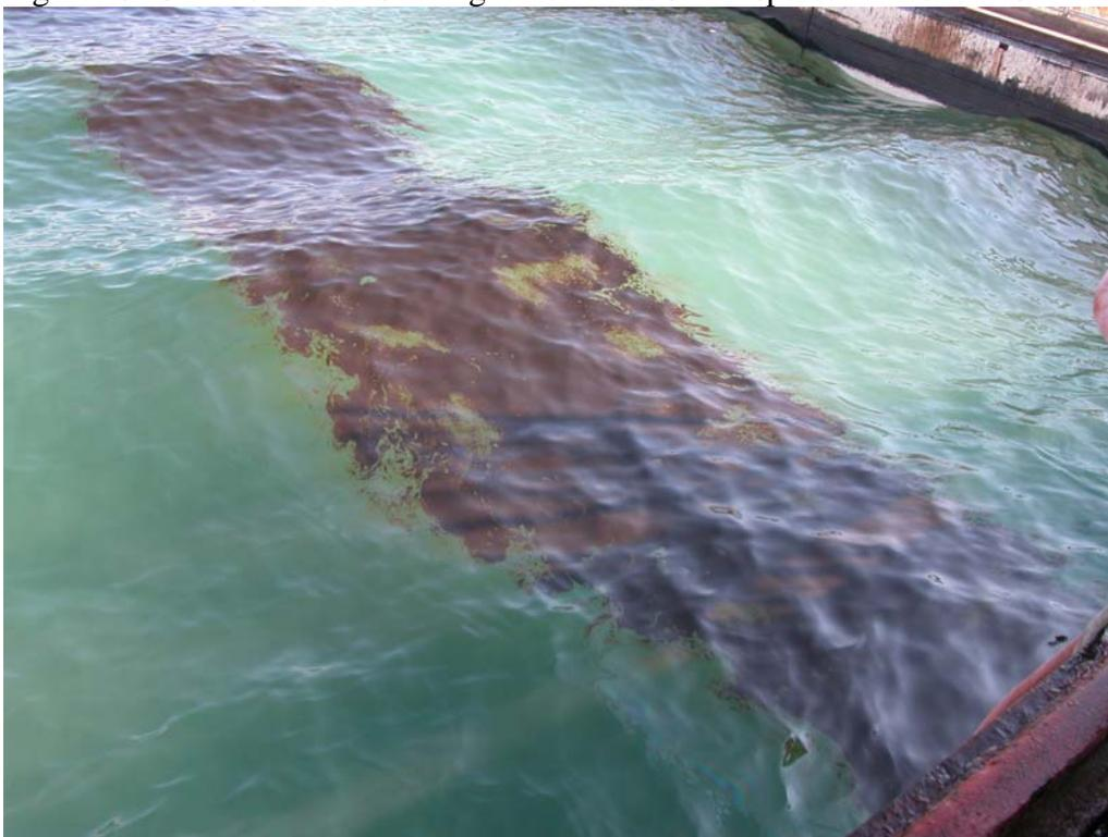
Figure 16 Slick from Test 4 – Control Slick, 10% Weathered Point McIntyre. This is Immediately After Deposition
