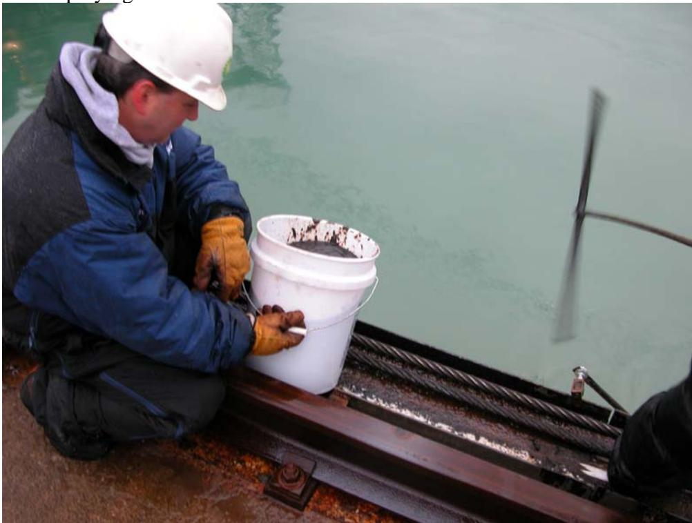
Figure 24 Oil Recovered from Test 9 – Dispersed 15% On Tank Weathered ANS. This is after the First Sweep About 50 Minutes after Dispersion
