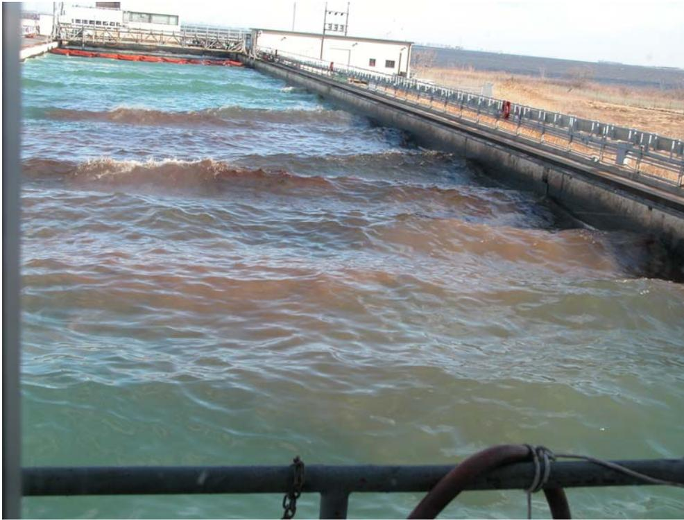
Figure 27 The Slick from Test 10 – Dispersed 15% On-Tank Weathered ANS – About 15 Minutes After Dispersion. Note that Dispersion is Relatively Wide Spread
