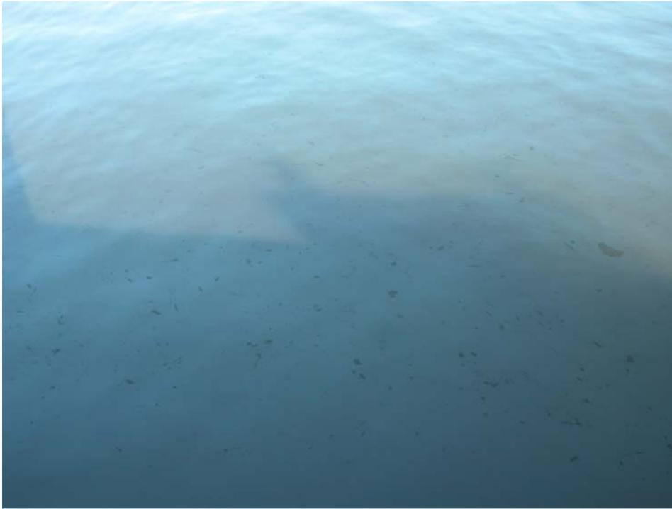
Figure 11 Resurfacing of Oil After Test 3, Fresh ANS Dispersed. This is About 55 Minutes After Dispersant Application and About 25 Minutes After Waves Were Turned Off.
