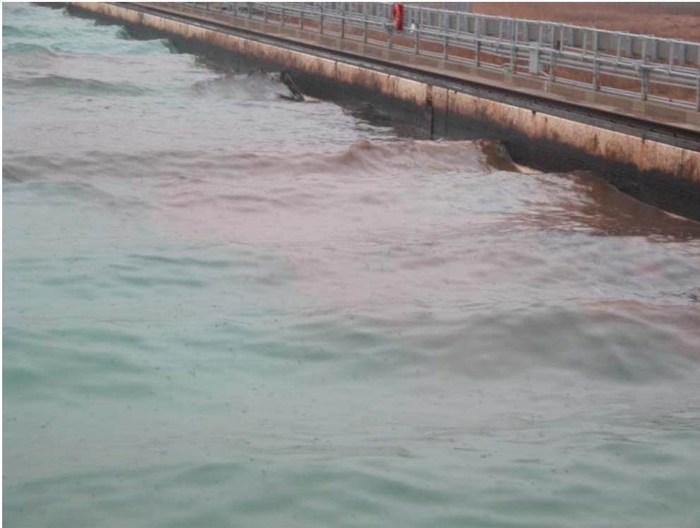
Figure 23 Dispersion from Test 9 – Dispersed 15% On-Tank Weathered ANS About 15 Minutes After Spraying
