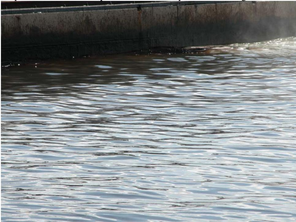
Figure 30 Resurfaced Oil From Test 11 – Dispersed 10% Weathered Endicott About 45 Minutes After Dispersion. Note that There Are Unmixed Dispersants in the Area
