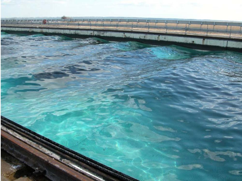
Figure 8 A View of the Second Test Involving Fresh ANS Oil. Note that this Oil Spread Readily Over much of the Tank. Significant Natural Dispersion Was Also Noted.
