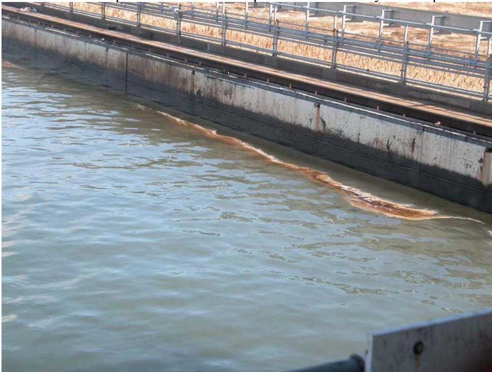
Figure 28 Resurfaced Oil From Test 10 – Dispersed 15% Weathered ANS About 45 Minutes After Dispersion. Note that There Still Are Unmixed Dispersants In the Area
