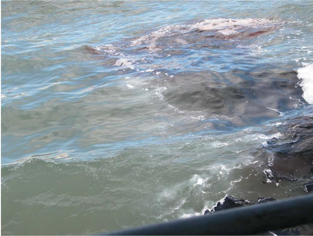
Figure 29 The Slick from Test 11 – Dispersed 10 Weathered Endicott – About 5 Minutes After Dispersion. Note that Dispersion is Some Dispersant Streaking
