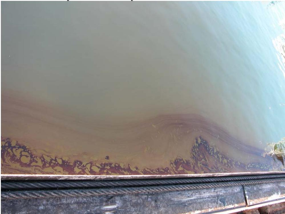
Figure 20 Resurfaced Oil From Test 6 - 16% Weathered ANS – Photo Taken About 50 Minutes After Dispersion. The Downwind Wall had Oil of This Density Along Most of Its Length
