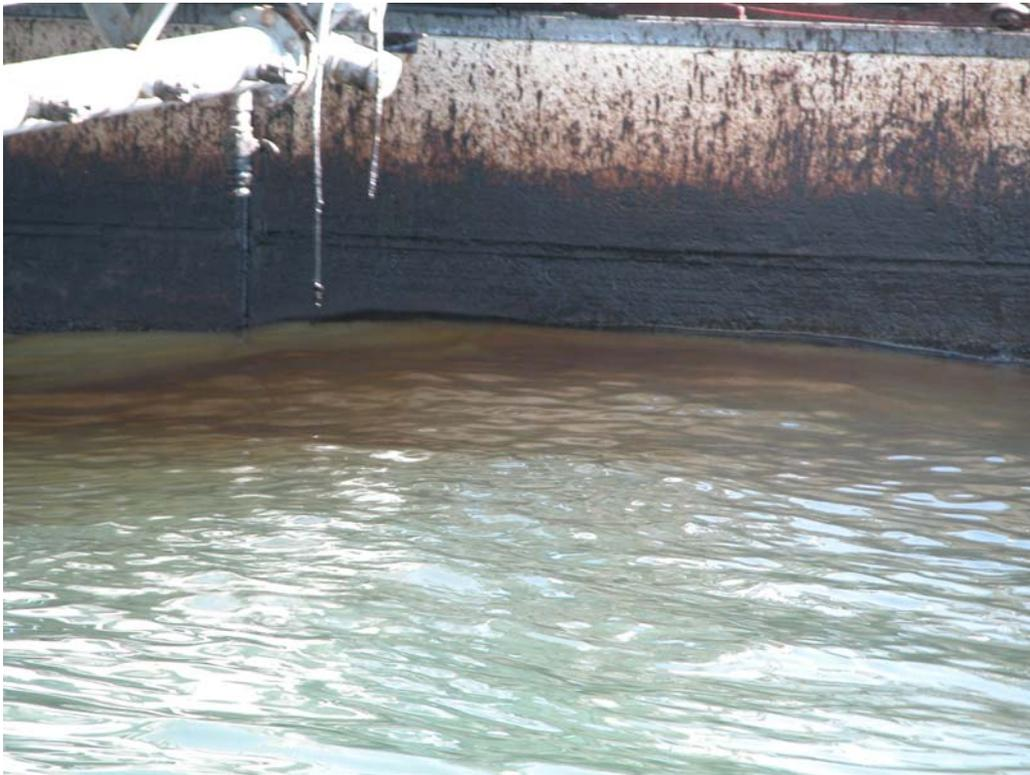
Figure 17 The Slick from Test 5 – 16% Weathered ANS – About 10 minutes After Slick Laid.
