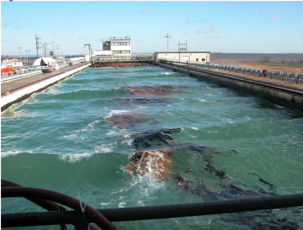
Figure 26 The Slick from Test 10 – Dispersed 15% On-Tank Weathered ANS – About 5 Minutes After Dispersion. Note that Dispersion is Just Beginning (Brown Areas) and That There is Some Dispersant Streaking
