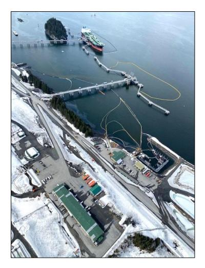
**Figure 2.** Containment booms placed around the spill site and in adjacent waters. Saw Island in upper left background adjacent Berth 5 tanker. Image from Alyeska Pipeline Service Company.
