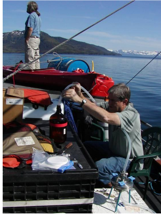
Figure 55 Vacuum filtration of a sediment/seawater sample after four days of mixing.
