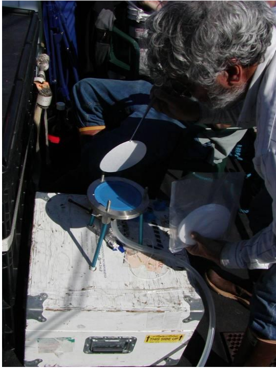
Figure 54 Placing a clean 0.7 \mu\text{m} glass fiber filter into the PLVWSS before sediment/ seawater sample processing.
