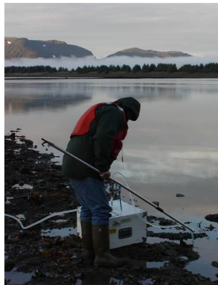
Figure 51 Wand and vacuum tubing used to collect a near-shore surface water sample.
