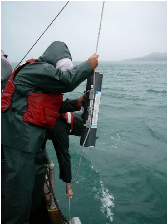
Figure 48 Seawater collection from the M/V Auklet using a 4-L GoFlo Bottle®.
