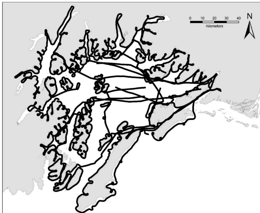
Figure 1. The 2019 survey flight tracks, which were essentially the same as the 2021 tracks. The apparent gaps in the survey flight tracks from 2019 are due to issues with the GPS recording device, but they were flown and recorded on the backup paper logs.
