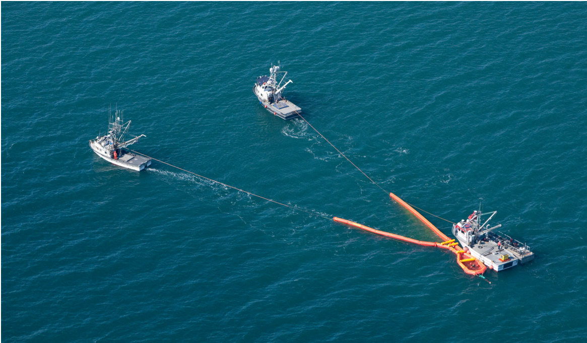
Figure 3-10. Example nearshore recovery system using Current Buster® containment deployed by three fishing vessels (Nuka Research photo)
