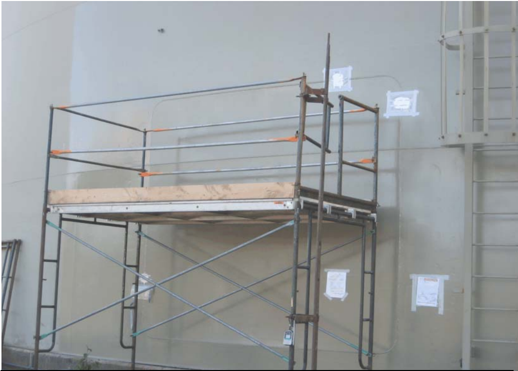
figure 3 - The taped areas represent where hardness measurements were taken on the door sheet.
