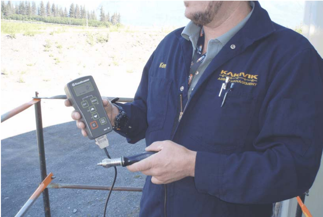
figure 5 - Krautkramer Model KB-MIC 10 hardness tester used to take the hardness measurements (SN#4633).
