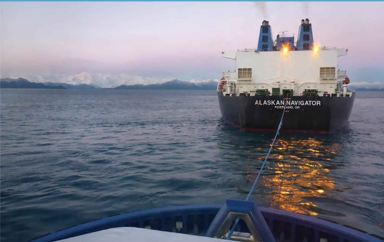
*Starting around 2003, a series of towlines broke during training exercises. Crowley Marine Services, which operated the tugs for Alyeska at that time, worked with the towline manufacturer to understand and address the problem. These failures underscored the importance of exercises and showed the need for continued close monitoring of the system.*
