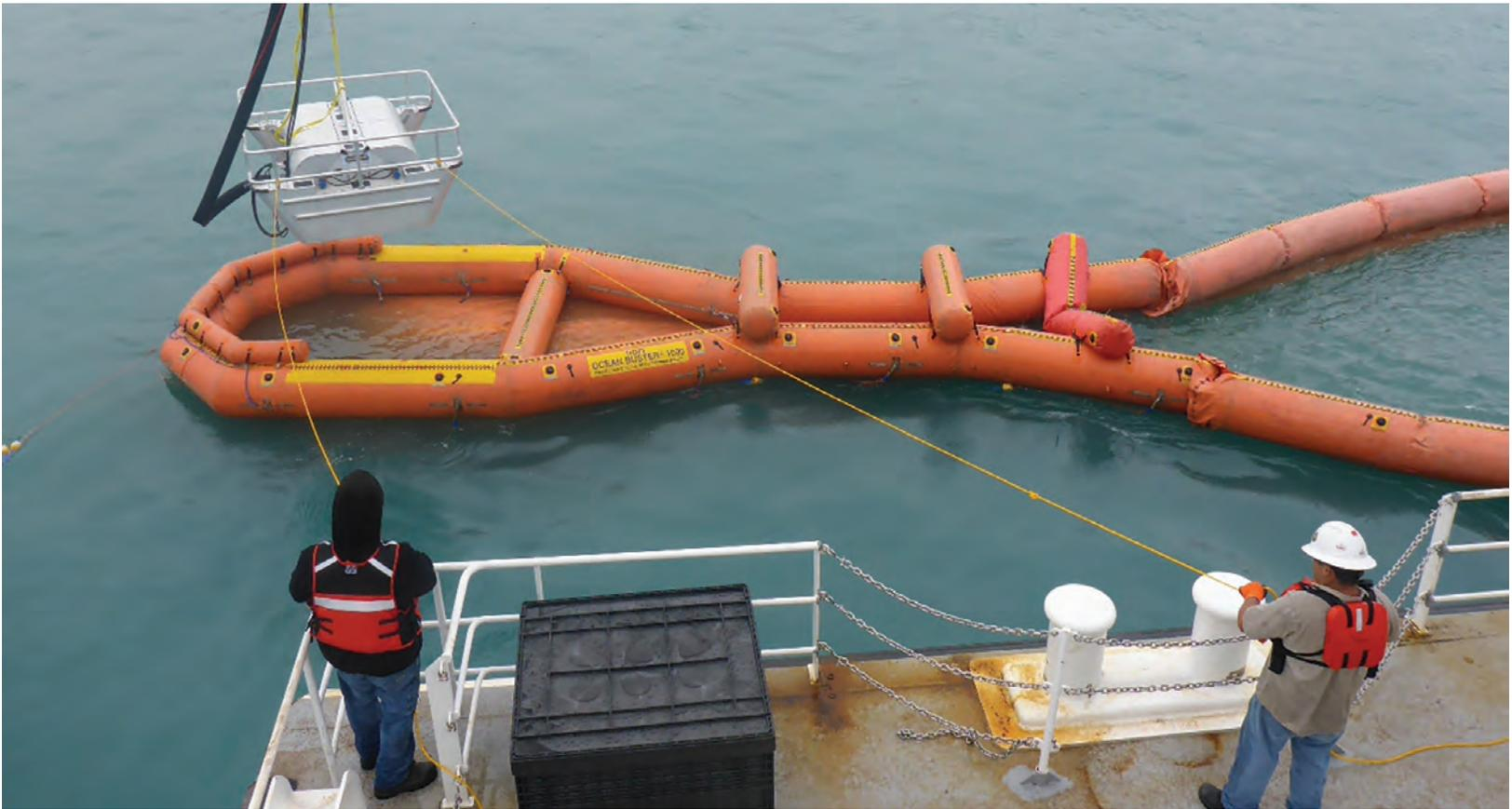
*The combination of the new Crucial skimmers with Buster boom systems have increased oil skimming efficiency since 1989.*
