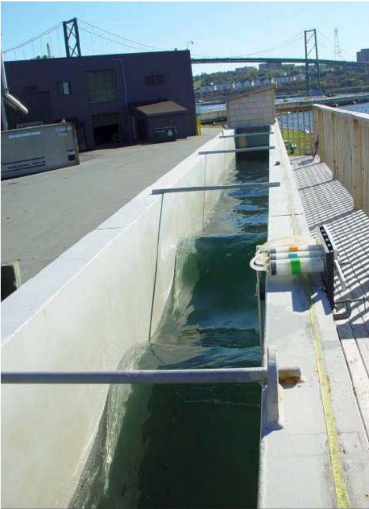
Figure 13: Wave tank located at BIO in Dartmouth, NS, Canada. This tank is collaboratively administered by DFO-COGER in Canada and the U.S. EPA. It is 60 m long by 0.5 m wide and 2 m deep. The normal operating depth is 1.5 m.
