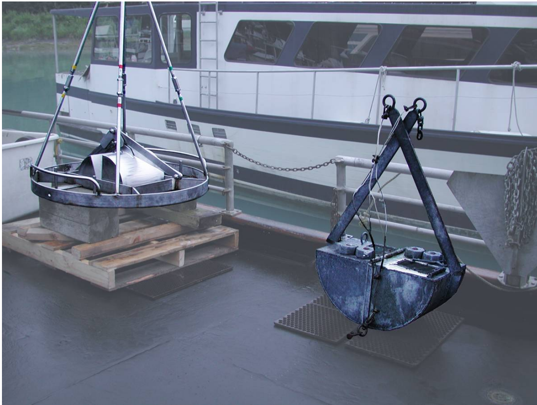
Figure 6. Modified (left) and unmodified (right) models of Van Veen grabs used in sampling method comparisons. The clam-shell buckets are cocked open on the left model and closed on the right.
