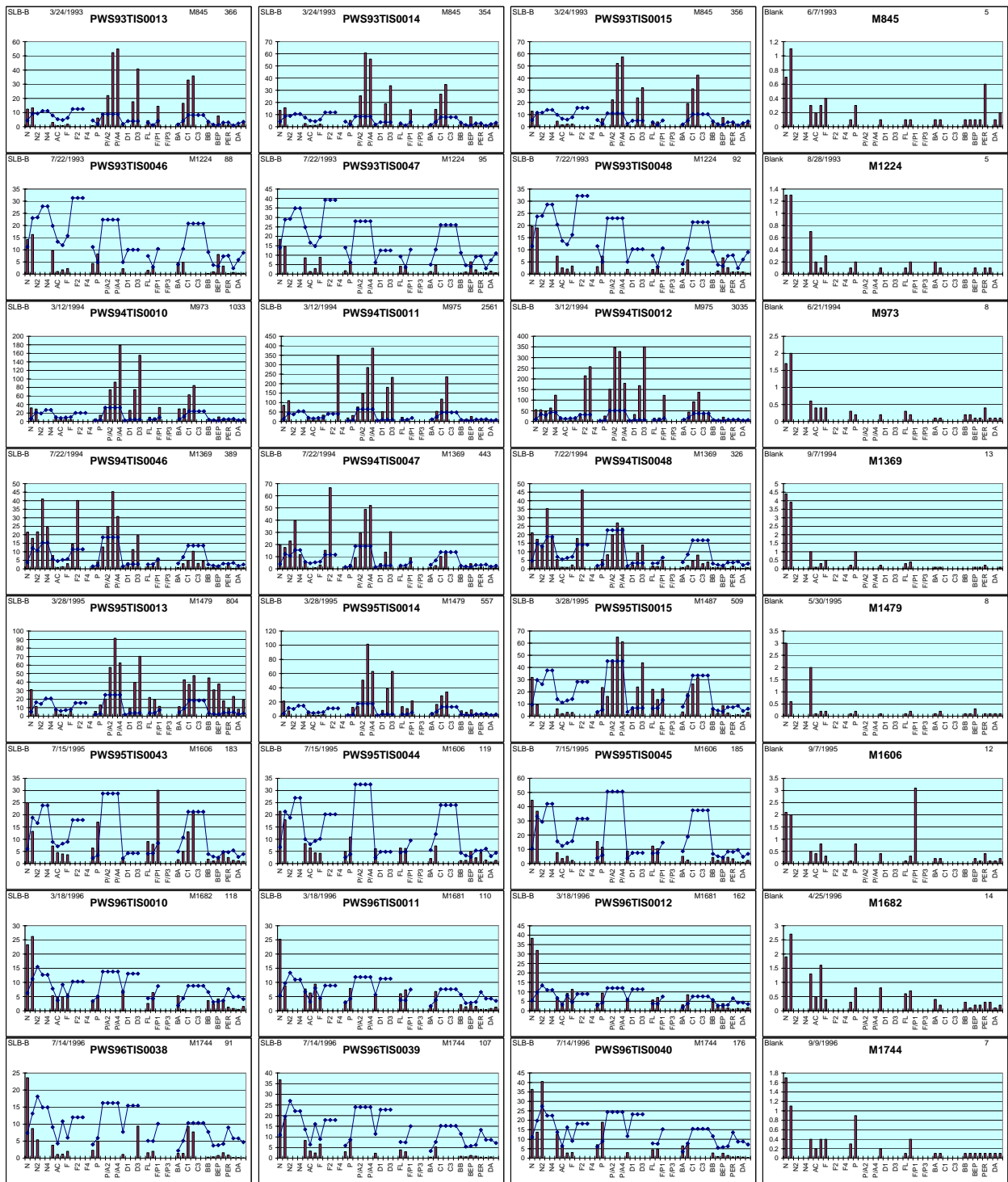
Figure 57. Compiled PAH histograms from Sleepy Bay (SLB) showing the presence of particulate/oil-phase PAH in March 1993, March 1994, July 1994, and March 1995 and the absence of oil-phase contamination reflected only by laboratory procedural artifacts in July 1993 and July 1995 through July 1996.
