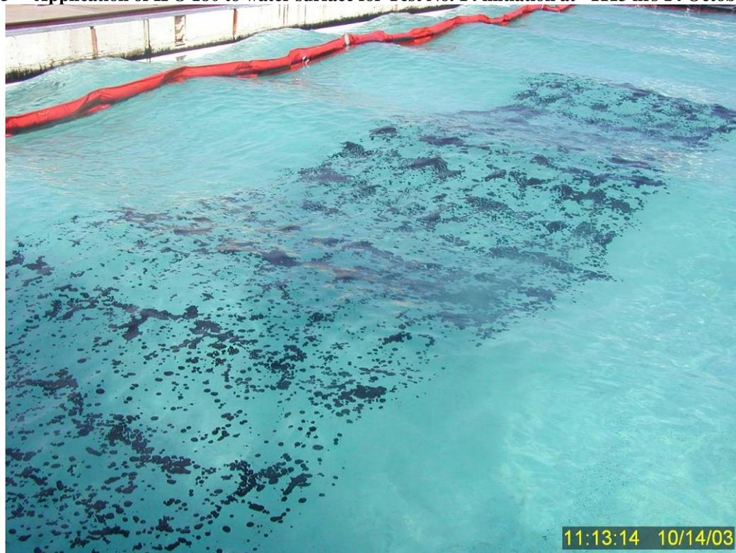
Figure 76 Quarter-sized oil patches and initial IFO 180 fuel oil spreading during the first 20 seconds of Test 14 (~ 12 seconds after dispersant application). Note: patchy oil distribution causes much of the dispersant to land directly on the water surface resulting in under dosing of the oil.
