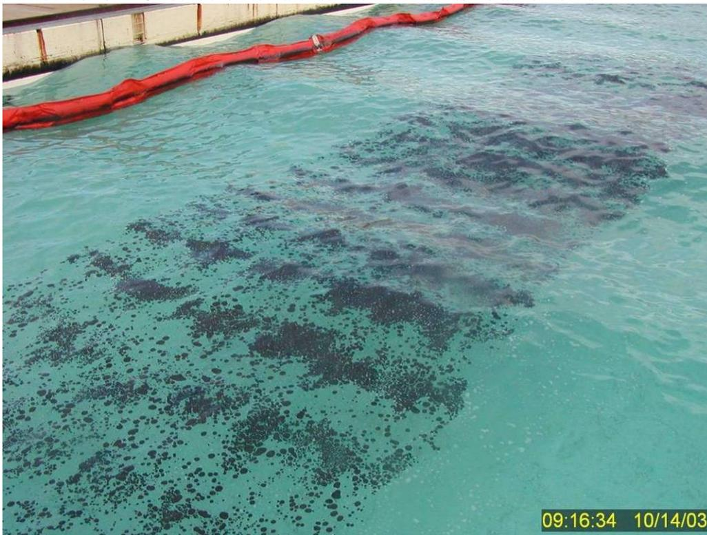
**Figure 64** Appearance of IFO 180 fuel oil ~20 seconds after SD25 dispersant application in Test No. 13. Note the uneven (patchy) distribution (lower left-hand corner) before the oil had a chance to spread. This caused much of the dispersant to actually land on the water resulting in under dosing the slick.
