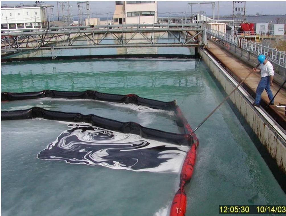
**Figure 90** Pulling the boom to the edge of the tank to facilitate collection of the remaining surface oil that had been herded by the fire monitors into the northeast corner of the experimental boom at the termination of Test No. 14.
