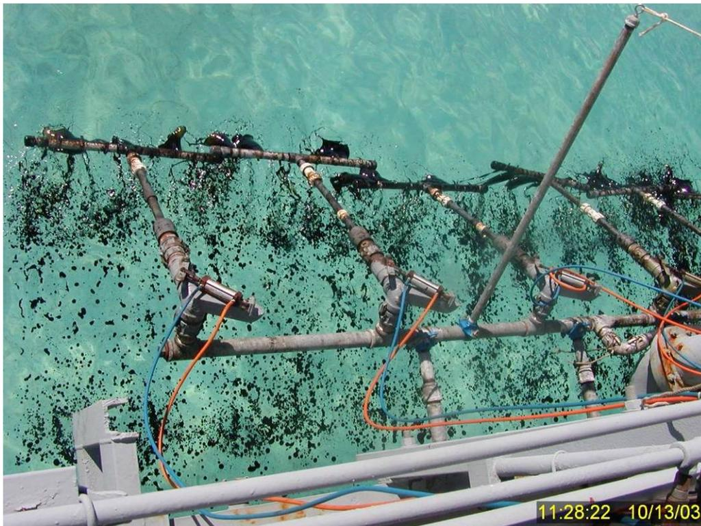
Figure 24 IFO 180 fuel oil addition to tank for Test No. 11 at 11:28:22 hrs, October 13, 2003.
