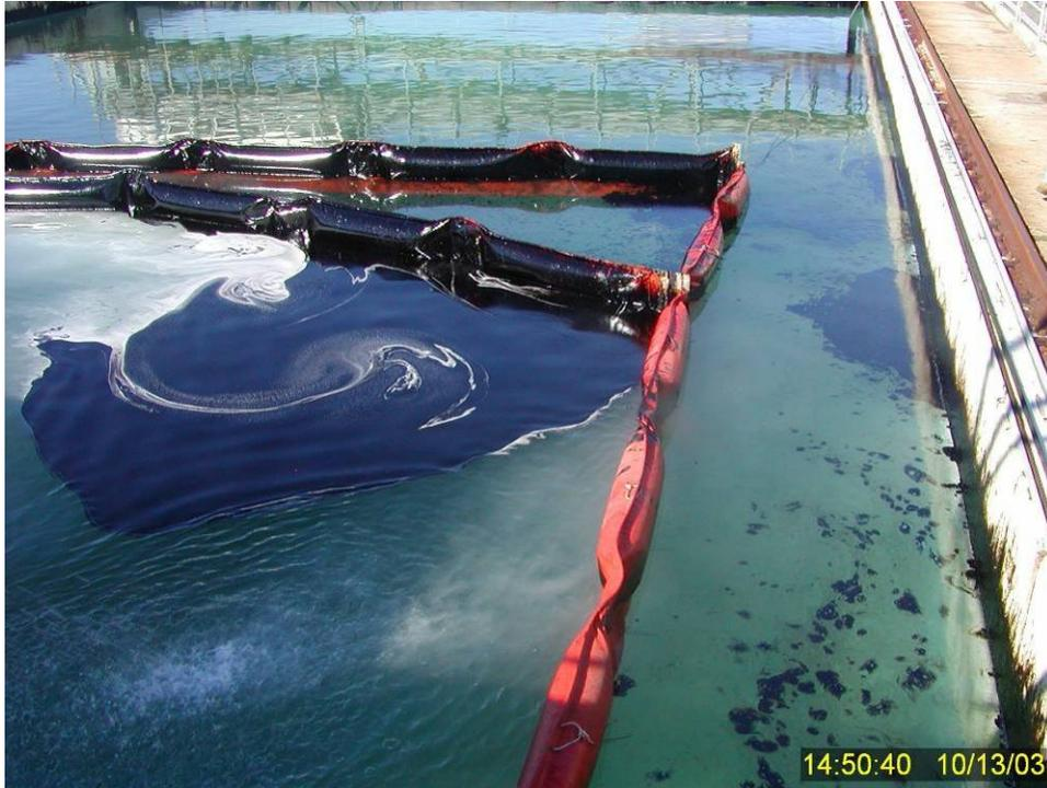
**Figure 55** Non-dispersed surface oil being herded into the north-east corner of the primary containment boom for collection. Note the surface oil between the containment boom and tank wall that apparently escaped during the test or resurfaced very soon after it was terminated.
