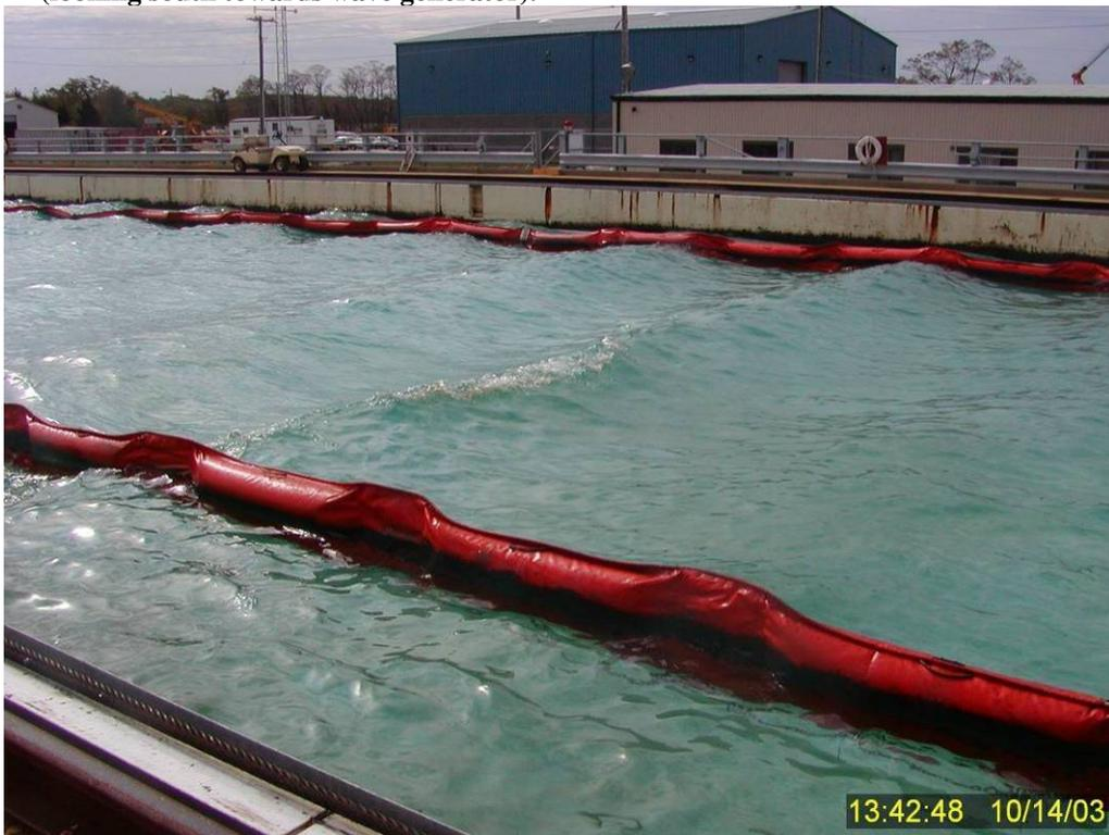
**Figure 95** Example of cresting wave turbulence at 33.3 cpm before Test No. 15. Usually there are no more than one to three such “breaking” waves within the experimental zone at this frequency setting.
