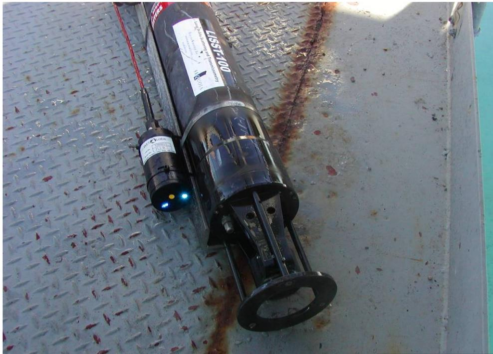
**Figure 4** LISST – 100 Particle Size Analyzer with WET Labs Fluorometer attached.
