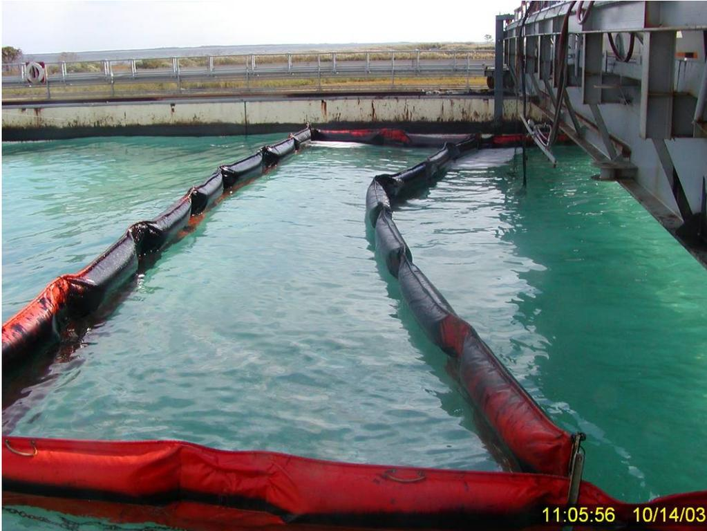
Figure 71 Secondary containment zone at the north end of the test tank showing no oil splash-over during Test 13.
