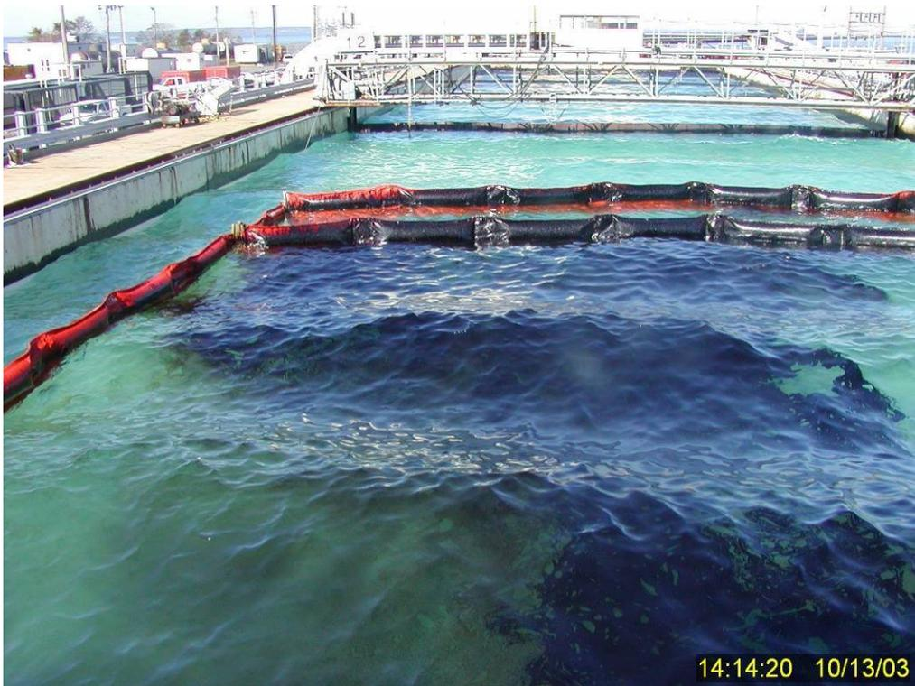
**Figure 46** Mixture of surface and some subsurface (dispersed) oil ten minutes into Test No. 12. This dispersant was only marginally successful under these conditions, but with time there was more evidence of oil entrainment into the water column.
