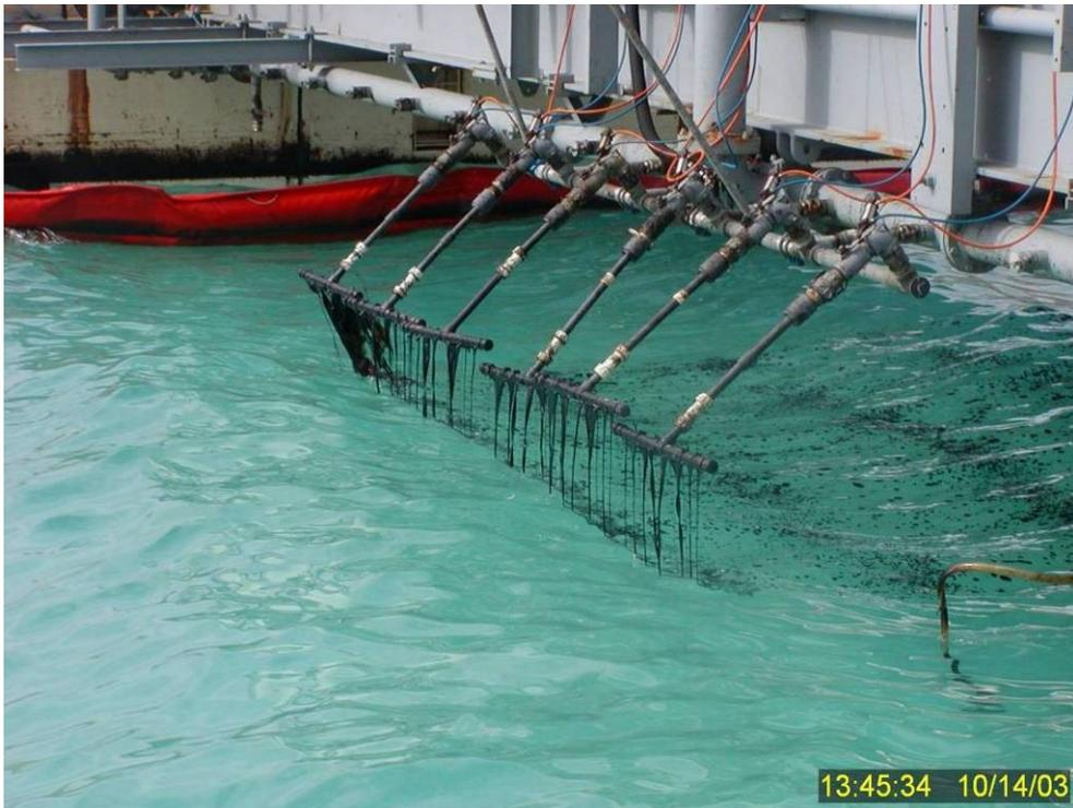
**Figure 96** Addition of IFO 180 fuel oil to the water surface at initiation of Test No. 15. For this operation, the bridge is moved at  $\frac{1}{2}$  knot to the south (from the right to the left) so that the oil on the water surface can be treated from a dispersant spray bar mounted on the other side of the bridge (see Figure 97).
