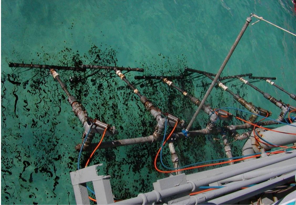
**Figure 15** Introduction of IFO 180 fuel oil from oil manifolds beneath movable bridge at initiation of Test No. 10.
