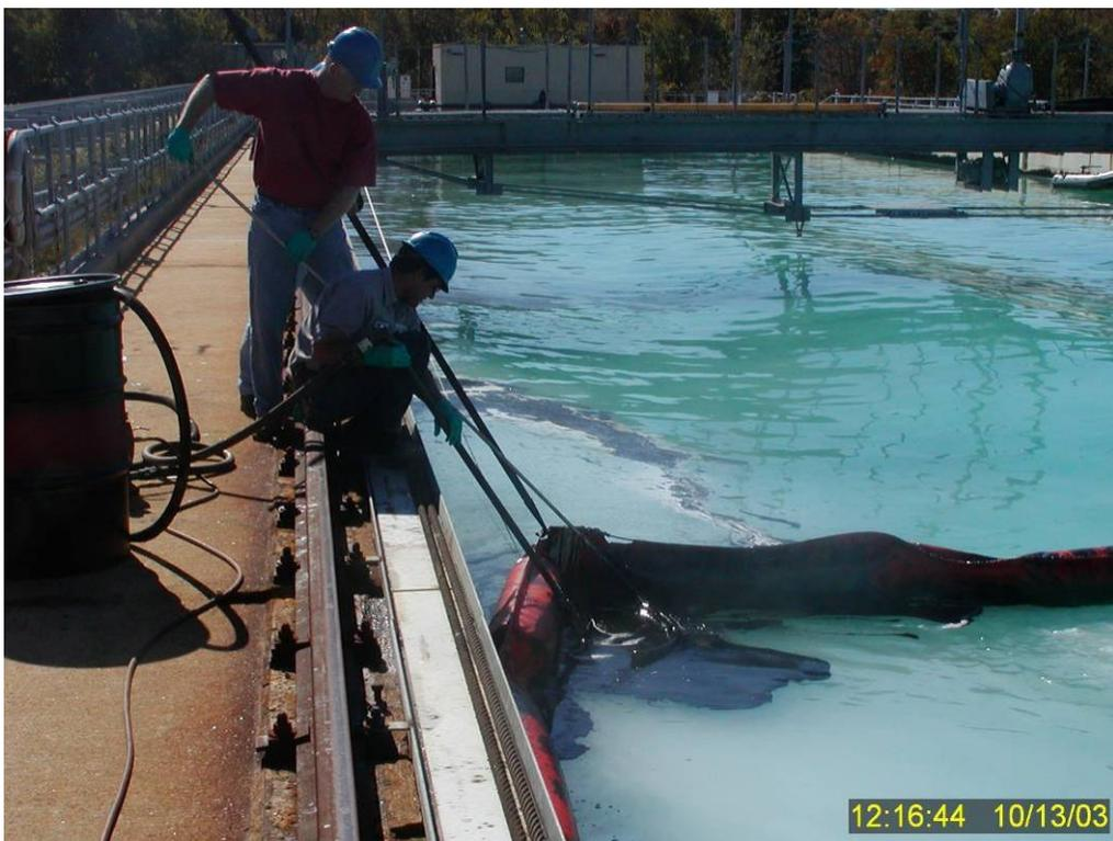
**Figure 40** Test No. 11: Vacuum recovery of non-dispersed surface oil at conclusion of test. A separate oil drum (on left) is used to contain the oil from each test to allow later quantification of recovered oil after allowing for oil/water separation. Collected oil is analyzed for water content by the lab at OHMSETT.
