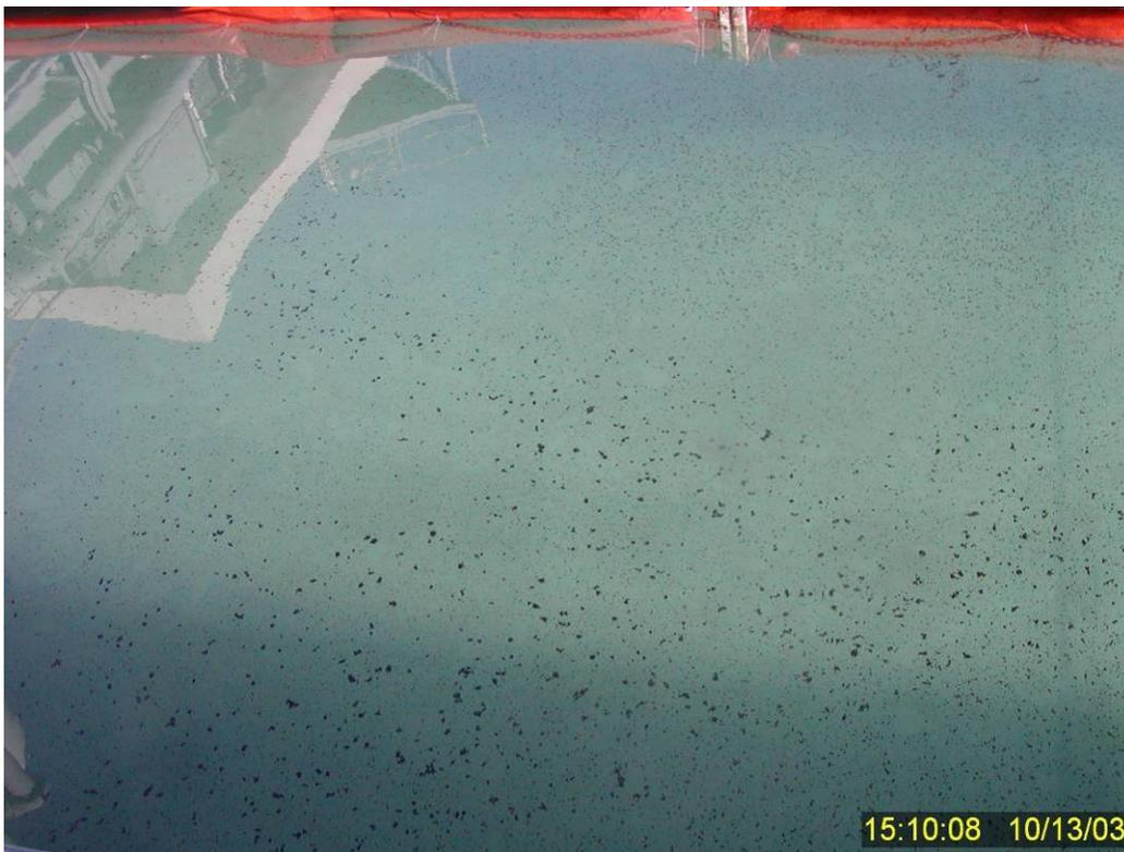
**Figure 59** Close-up photograph of agglomerating oil droplets resurfacing between the western tank wall and containment boom ~ 36 minutes after turbulence was terminated at the end of Test 12.
