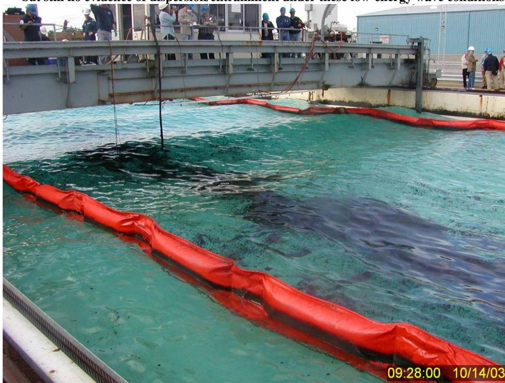
**Figure 66** Movable bridge positioned over the slick 12 minutes after dispersant application. Note the fluorometer cables passing directly through the slick to provide data from 1- and 2-m directly beneath the oil.
