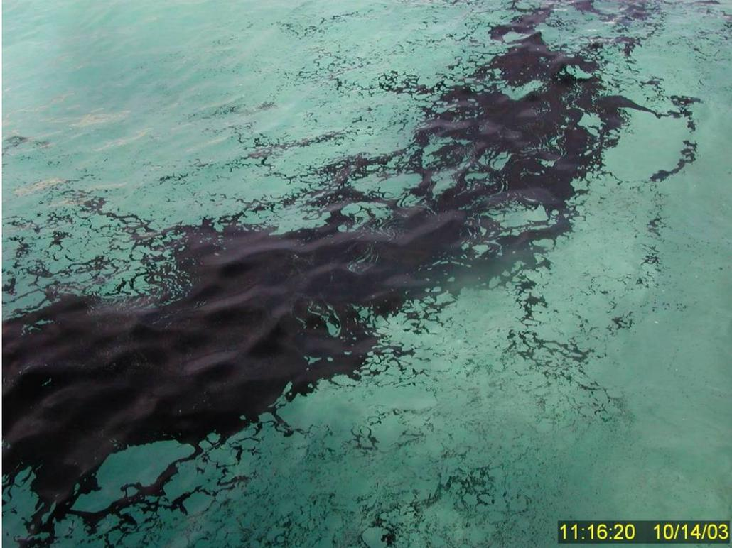
**Figure 79** Close up of surface slick three minutes after Test No. 14 dispersant application showing no dispersion/entrainment.
