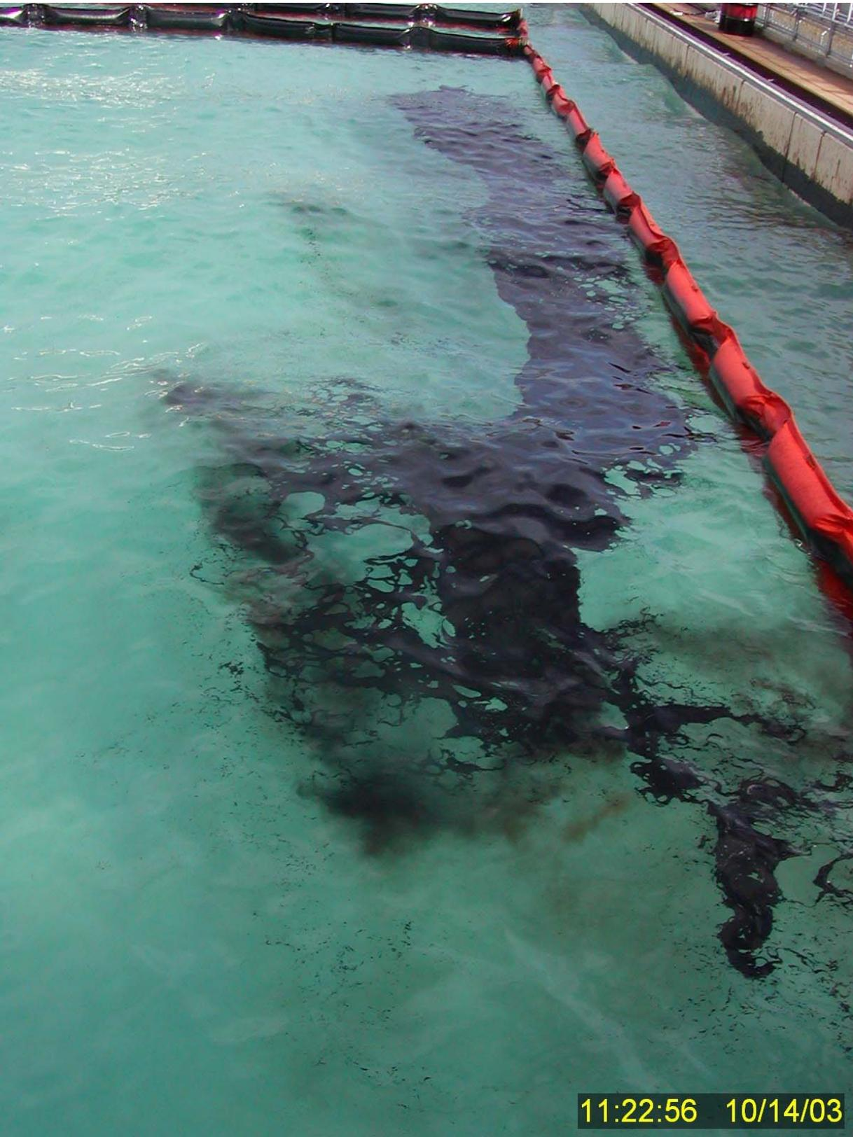
**Figure 84** Localized dispersion caused by dragging fluorometer cables and submersible pump lines through the surface slick.
