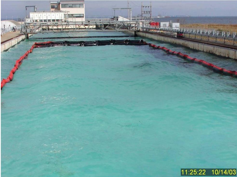
**Figure 86** Unusual standing wave pattern (both along and across the tank) that developed approximately 12 minutes into Test No. 14. Note, this was still not a high enough energy regime to facilitate chemical dispersion, and at this time most of the oil had migrated to the east side and north-east corner of the experimental zone.
