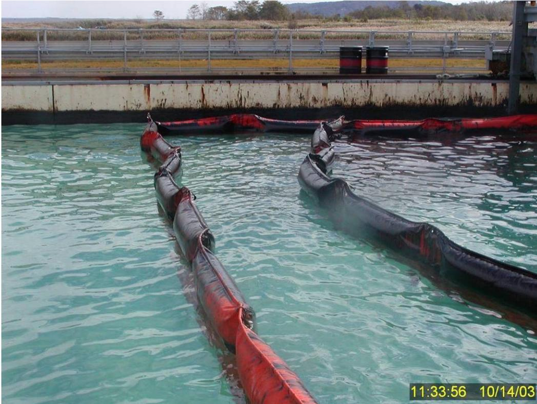
Figure 88 Secondary containment boom showing no splash over or dispersed oil plume at the termination of Test No. 14.
