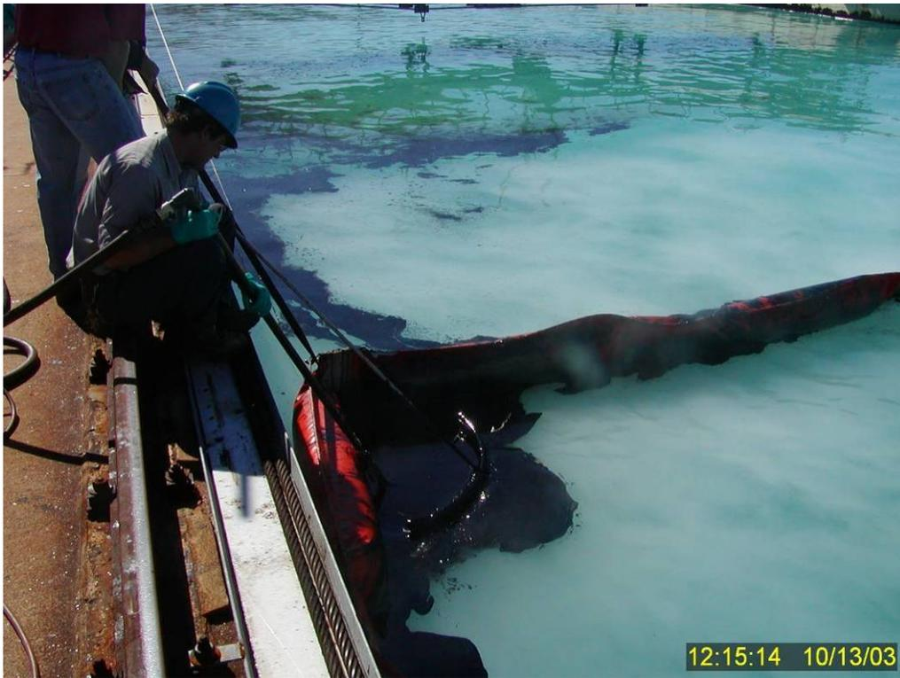
**Figure 39** Test No. 11: Squeegee and vacuum hose recovery of surface oil at termination of test.
