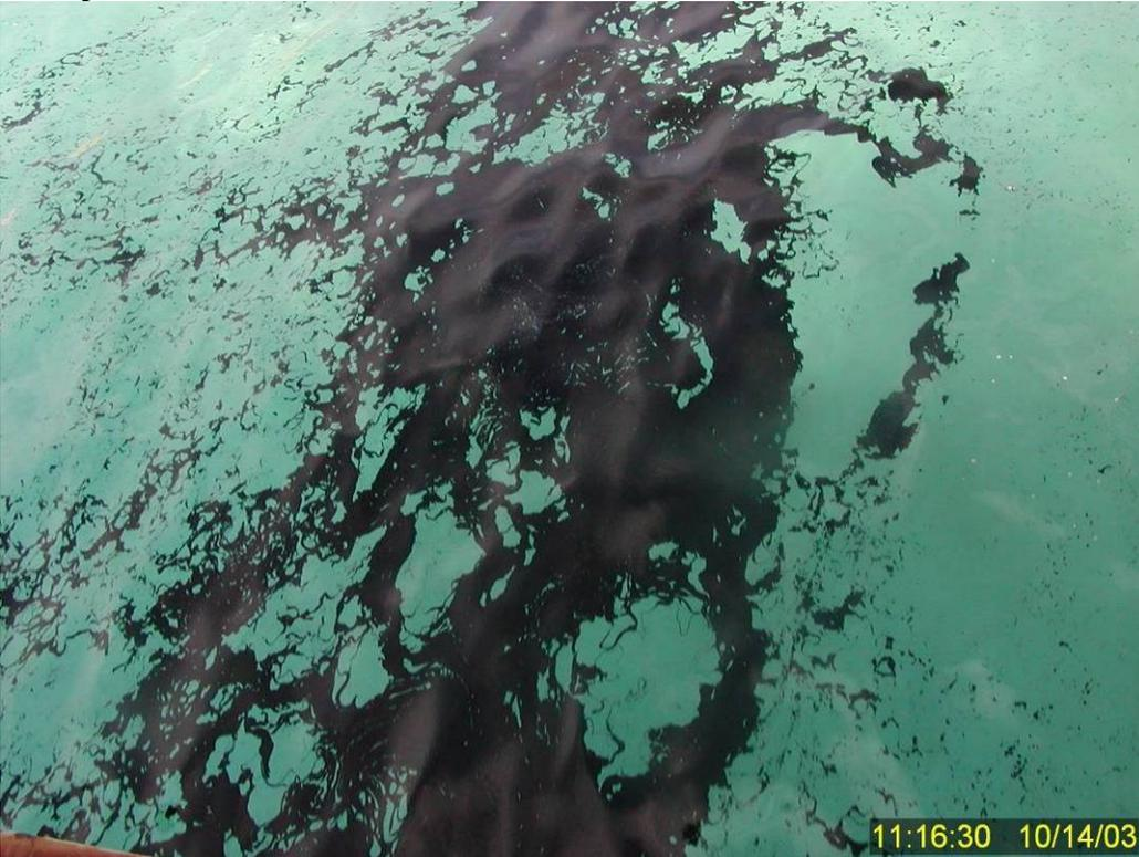
**Figure 80** Surface oil slick showing no significant dispersion/entrainment three minutes after treatment.
