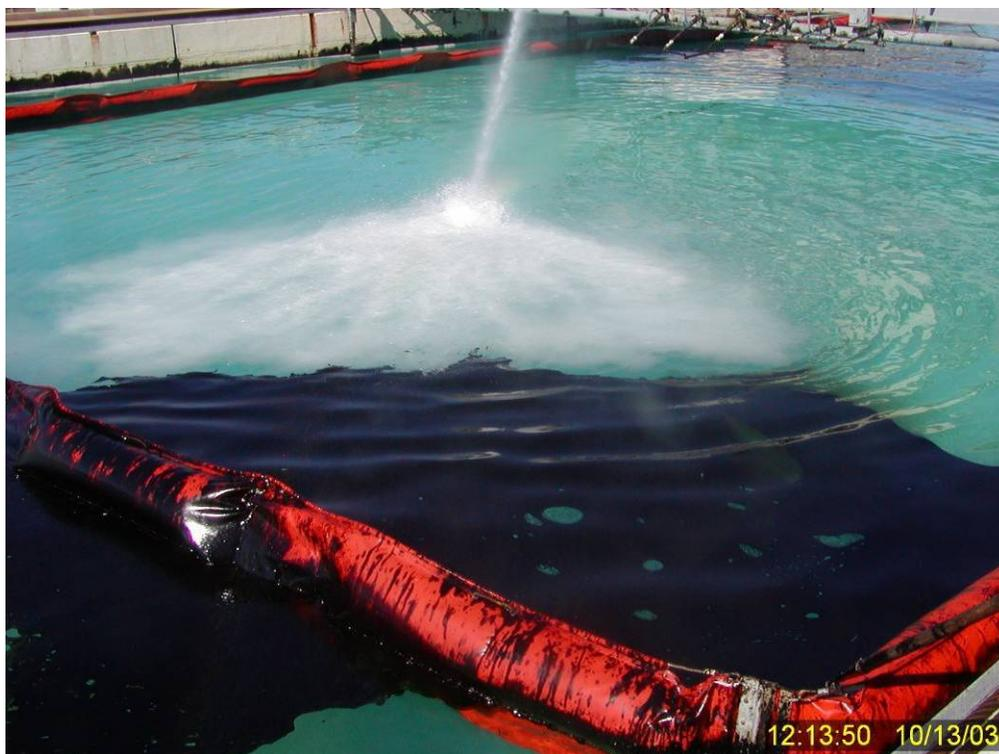
**Figure 37** Test No. 11: Use of fire monitor spray to herd surface oil into corner of boom to facilitate recovery by vacuum. Note the spray is directed to water surface 10-15 feet from oil to avoid accidental entrainment.
