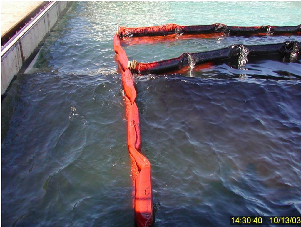
**Figure 53** Discoloration of subsurface water by lateral diffusion of dispersed oil outside the containment boom 26 minutes into Test No. 12 (just before the wave turbulence was discontinued at 1434 hrs).
