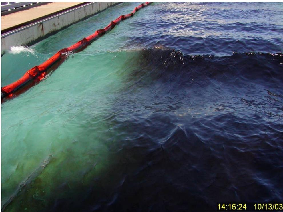
**Figure 48** Lateral spread of subsurface (dispersed) oil twelve minutes after dispersant treatment. Note 2-4 inch breaking wave in upper third of photograph and rough texture of water surface showing lack of coherent oil slick.
