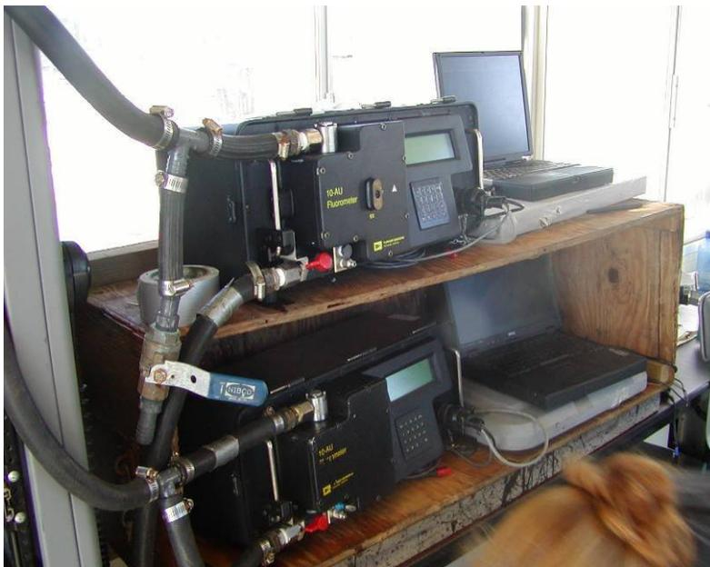
Figure 1 Parallel Turner 10 AU fluorometers (with intakes at 1 and 2-m) used for OHMSETT heavy fuel oil studies.
