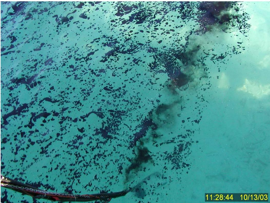
Figure 26 Test No. 11: Minor (and anomalous) dispersion/entrainment of IFO 180 fuel oil due to turbulence introduced by dragging fluorometer cable through dispersant-treated surface oil.
