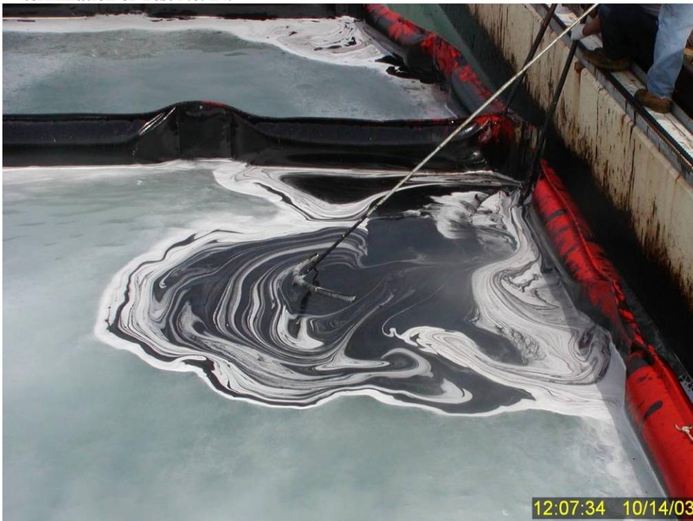
**Figure 91** Squeegee and vacuum recovery of the last remnants of non-dispersed surface oil from Test No. 14. The white foam is believed to be dispersant that was emulsified by the fire monitor spray during surface oil recovery.
