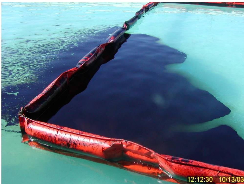
**Figure 35** Test 11: Non-dispersed IFO 180 fuel oil within containment boom ~30 minutes after the conclusion of the test. By this time some residual IFO 380 oil from earlier tests had drifted against the outside of the containment boom used for the test.
