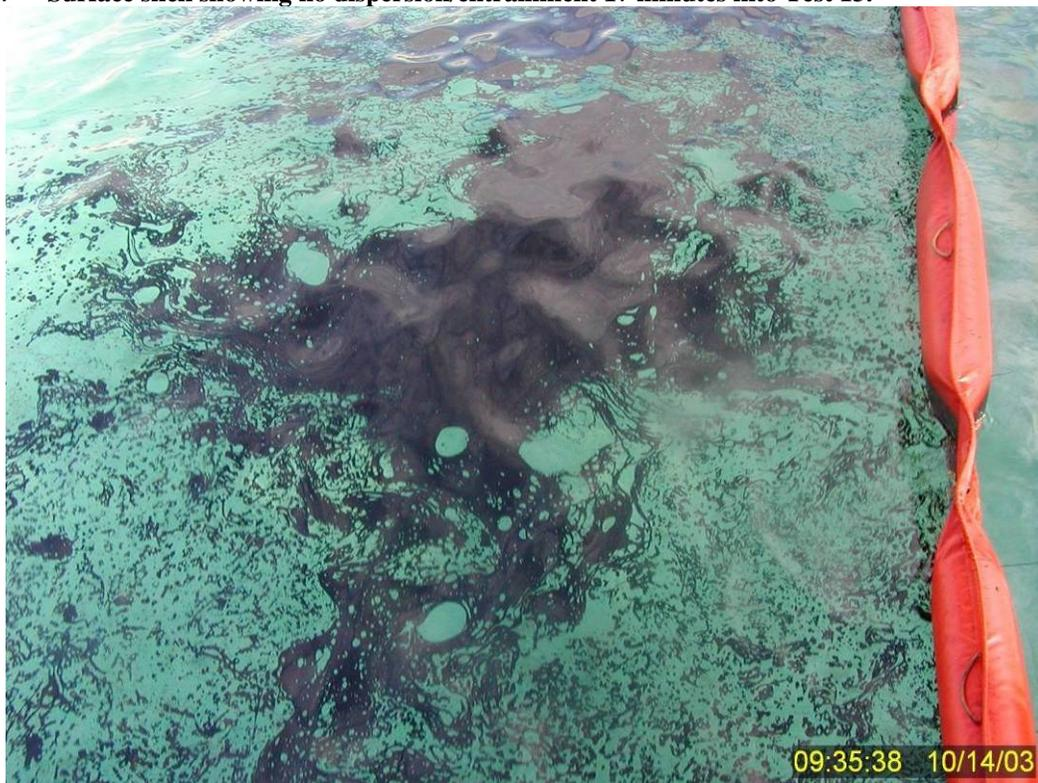
**Figure 68** Close up of surface slick from the bridge positioned directly over a larger patch of nondispersed surface oil 19 minutes into Test 13. There was no evidence of any chemically enhanced or natural dispersion noted.
