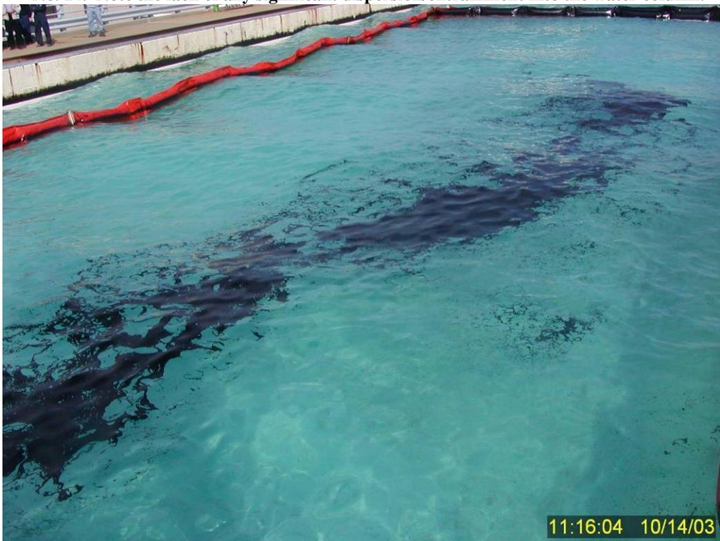
**Figure 78** Overhead view of IFO 180 fuel oil three minutes after Test No. 14 treatment with Corexit 9500 under light energy (low wave turbulence) regime.
