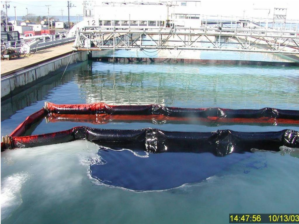
**Figure 54** Herding of non-dispersed surface oil at the termination of Test 12. Note the fire-monitor spray is directed to the water surface not the oil to avoid unwanted entrainment during collection.
