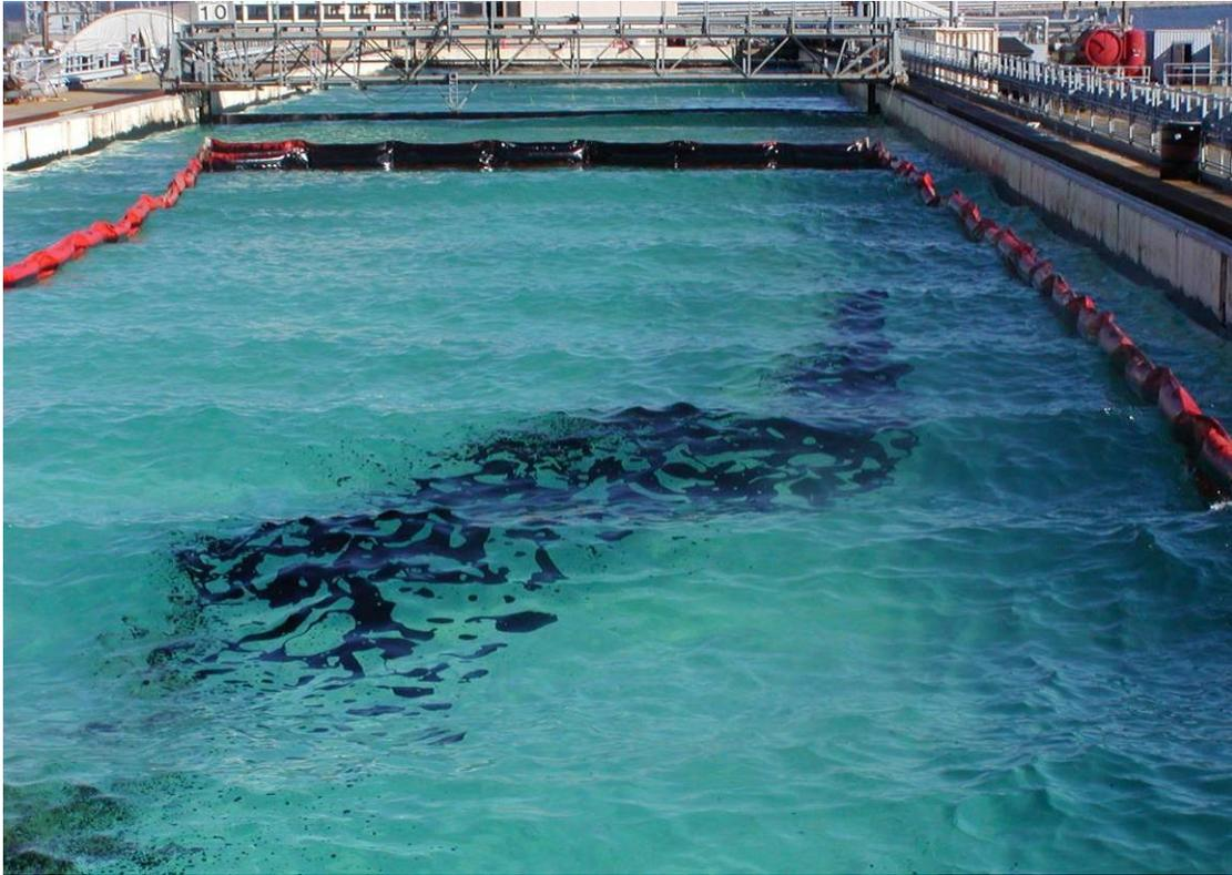
**Figure 19** IFO 180 control slick approximately 15 minutes after initiation of Test No. 10 (looking north). The darker water on the right is due to the shadow from the edge of the tank.
