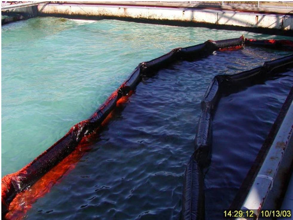
**Figure 52** Overhead photograph of smooth nondispersed surface oil within primary containment boom (on right) and subsurface dispersed oil visible within secondary containment boom. Note there is also some non-dispersed surface oil along the upper edge of the secondary boom but not outside of it.
