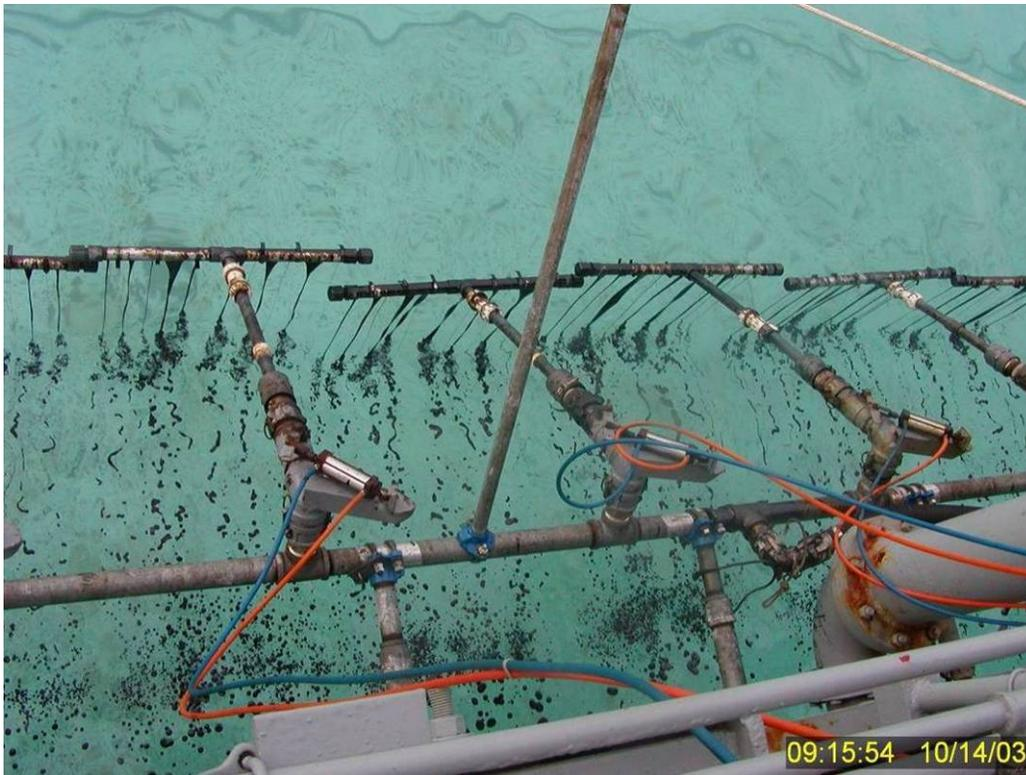
**Figure 63** Addition of IFO 180 fuel oil to water surface for Test No. 13 at ~0916 hrs.
