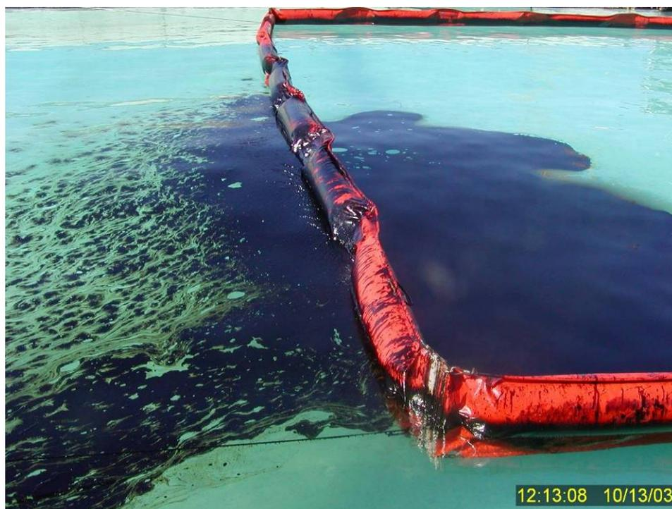
**Figure 36** Test 11: Close-up of southeast corner of containment boom showing the different appearance of the residual IFO 380 from earlier tests with the non-dispersed IFO 180 from Test 11 before recovery.
