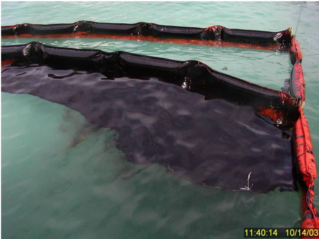
Figure 89 Non-dispersed surface oil that had been driven by the wind and waves into the northeast corner of the experimental zone during Test No. 14. Note the lack of any significant oil in the secondary containment boom at the top of the figure.
