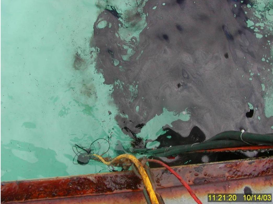
**Figure 81** Fluorometer and submersible pump cables dangling from movable bridge into surface oil slick seven minutes after Test No. 14 Corexit 9500 treatment under low-energy wave regime.
