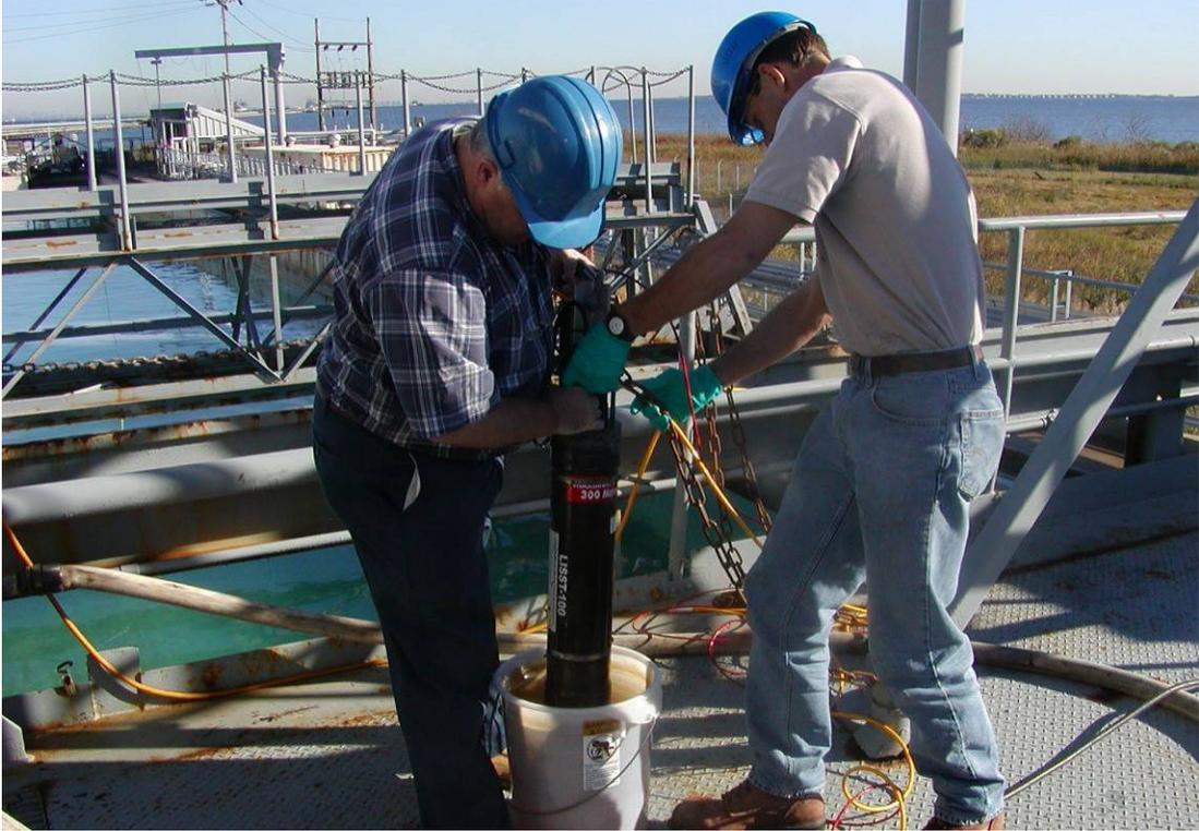
**Figure 7** Calibration of LISST particle size analyzer and WET Labs fluorometer.
