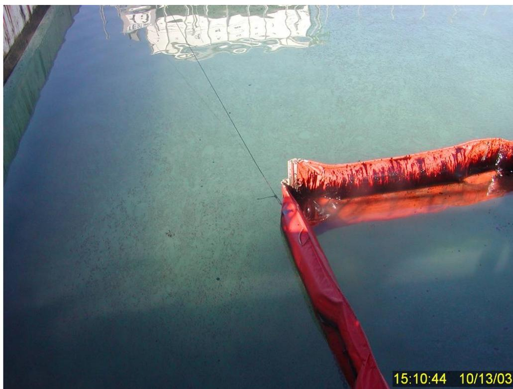
**Figure 60** Resurfacing dispersed oil droplets outside the secondary containment boom ~36 minutes after turbulence was terminated at the end of Test 12.
