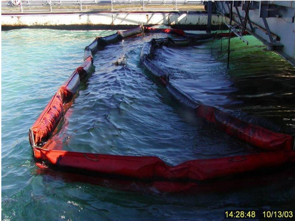
**Figure 51** Wave induced strain on primary containment boom and minor surface oil in secondary containment boom 24 minutes into Test No. 12. Note the discoloration of the water from subsurface dispersed oil droplets both within and outside the secondary containment boom.
