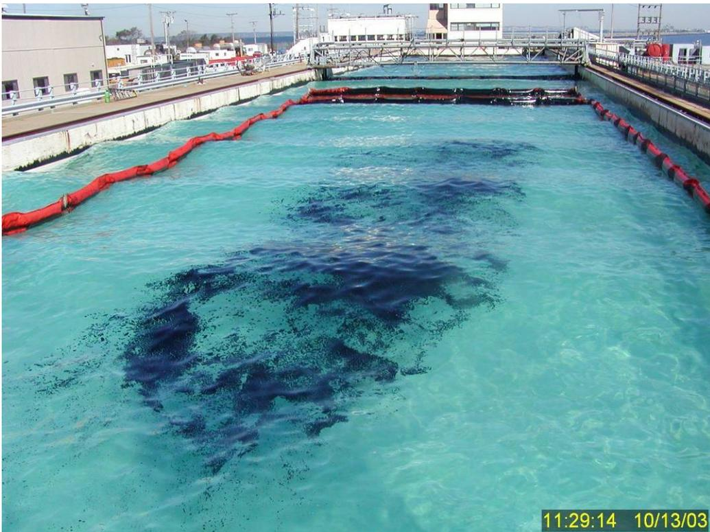
**Figure 28** Test 11: Dispersant-treated IFO 180 ~50 seconds into experiment. Still no significant oil entrainment with this dispersant under these test conditions.
