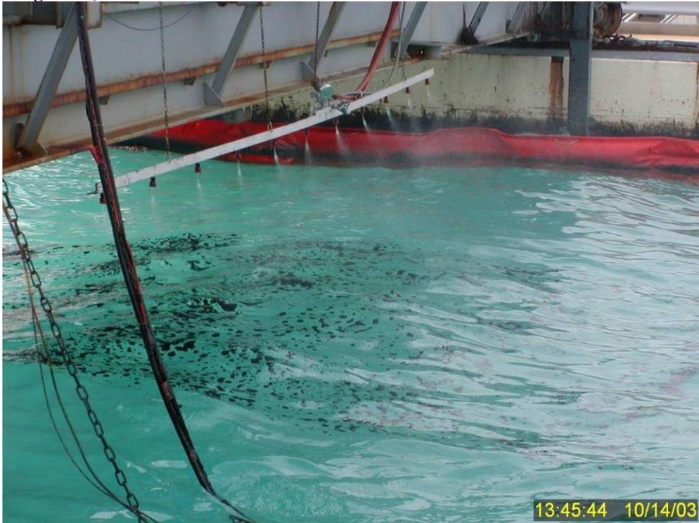
**Figure 97** Application of Superdispersant 25 to surface oil as the bridge is advanced at  $\frac{1}{2}$  knot to the south (left). The oil is on the water surface for only 8-10 seconds before dispersant application. Note the fluorometer cables and submersible pump are off to the side of the treated oil.
