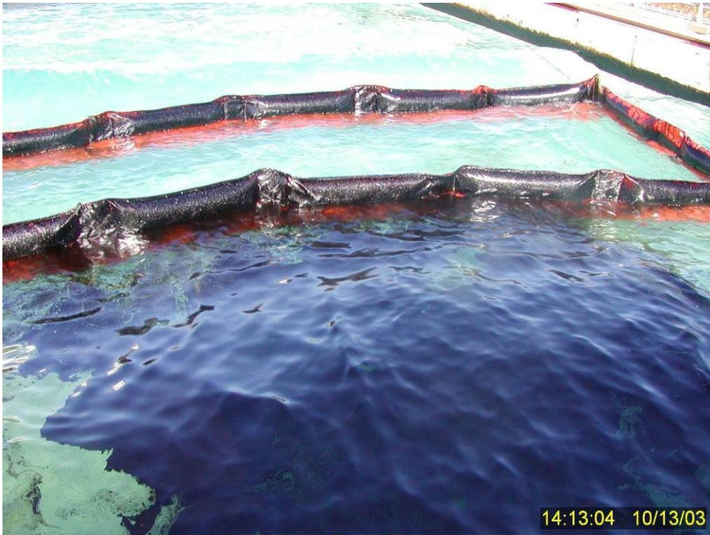
**Figure 45** Surface (non-dispersed) oil contained within experimental zone (note the clean water within the secondary containment boom) nine minutes after initiation of Test No. 12.
