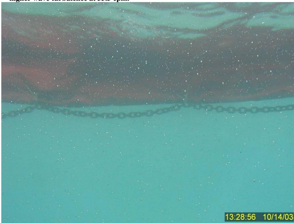
Figure 93 Containment boom from northern-most underwater window showing water clarity before Test No. 15.
