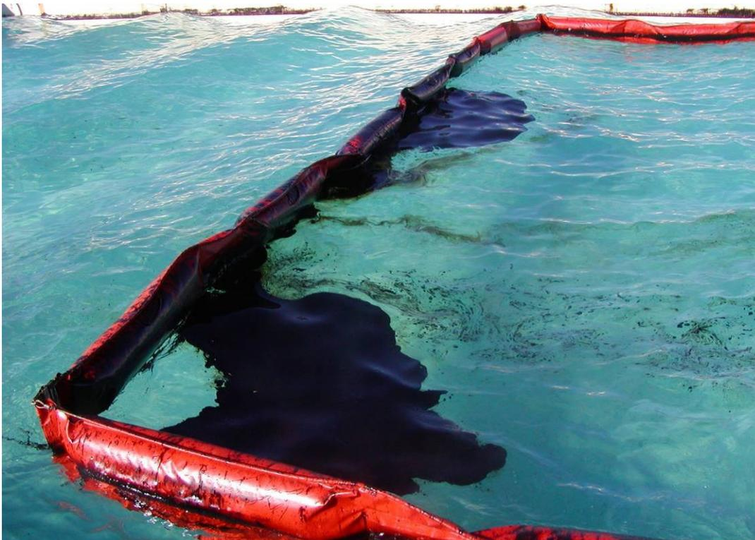
**Figure 21** Captured oil at south end of test enclosure boom at termination of IFO 180 control Test No. 10.
