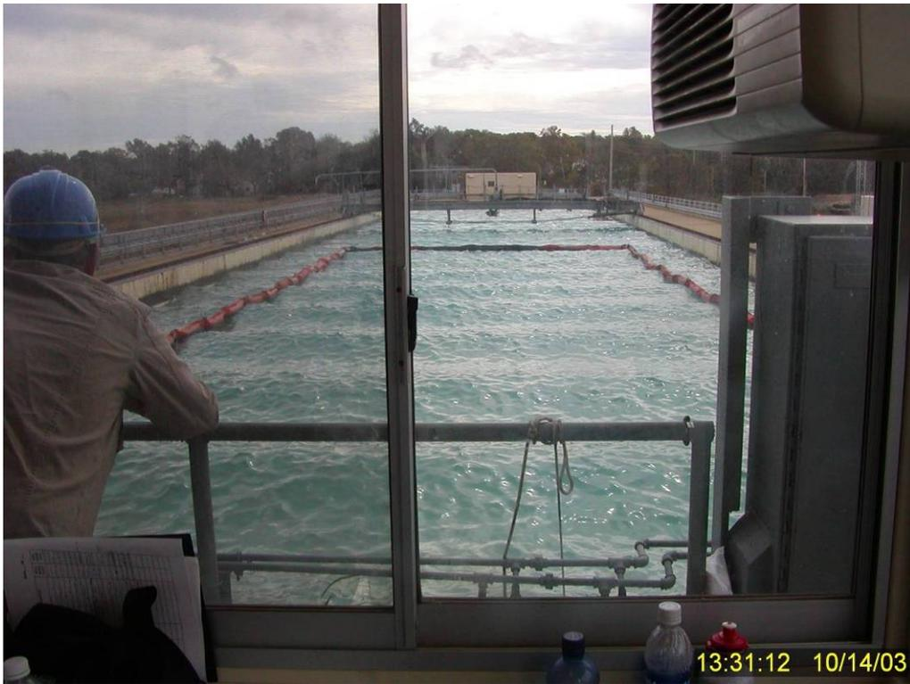
**Figure 94** Wave train viewed from the control room on movable bridge before Test No. 15 initiation (looking south towards wave generator).
