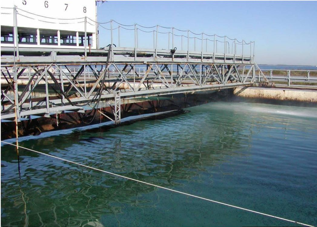
**Figure 61** Final 13 October 2003 cleaning/polishing the wave tank by using the fire monitors to drive any remaining surface oil beneath the permanent curtain at the extreme north end of the tank.
