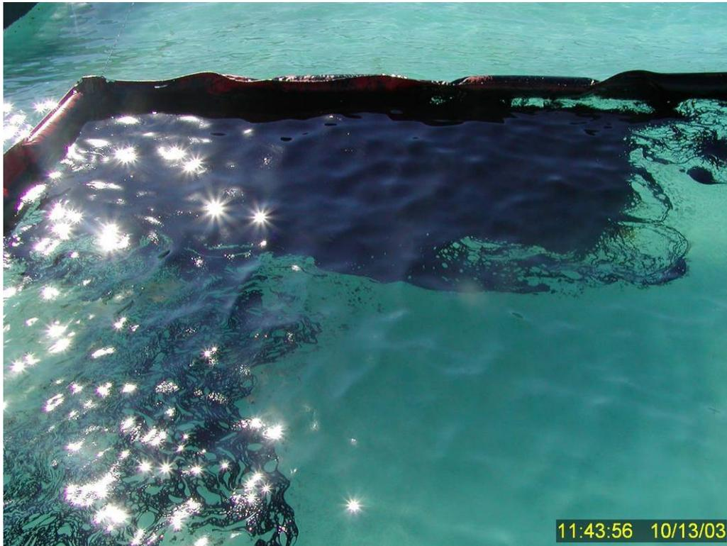
Figure 34 Test No. 11: Close up of non-dispersed surface oil in south-east corner of test boom ~ 22 minutes after initiation of the test. Note the lack of any oil outside the boom.
