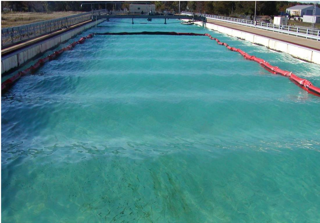
**Figure 14** Wave train before initiation of control test (No. 10) IFO 180 fuel oil, no dispersant, and wave generator set at 33 cycles per minute (cpm). Note trace of oil that was washed off/dripped from oil application manifold before test was started. Photographed looking south toward wave generator.
