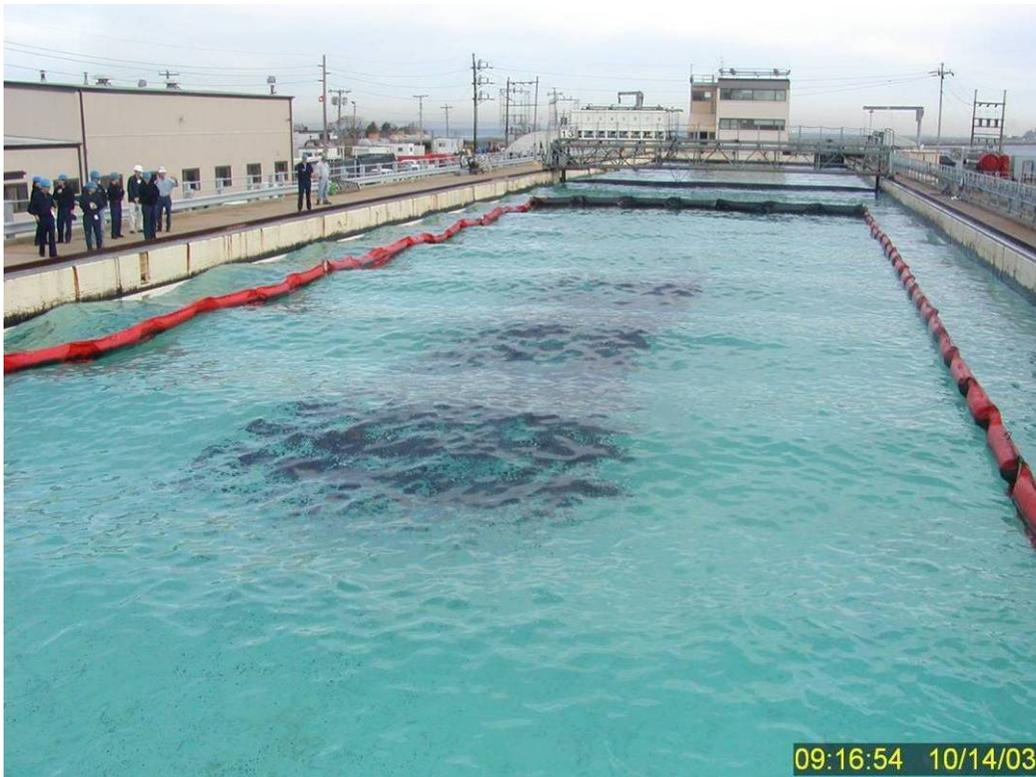
**Figure 65** Slightly better spreading 60 seconds after the oil was applied to the water surface in Test No. 13, but still no evidence of dispersion/entrainment under these low-energy wave conditions.
