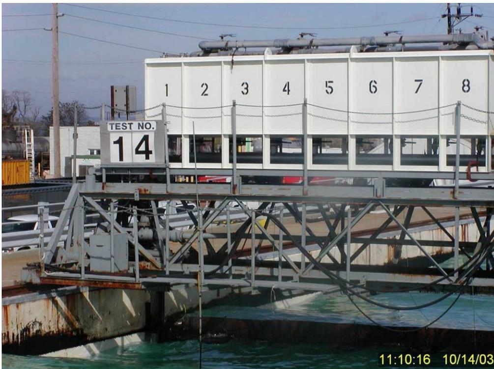
Figure 72 Set up for Test 14: IFO 180 fuel oil, Corexit 9500 at a nominal DOR of 1:50, and low-energy waves at 30 cpm.
