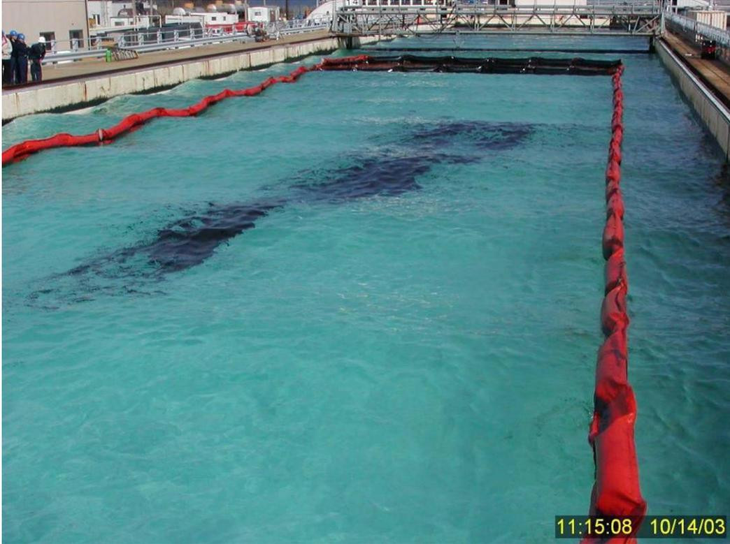
**Figure 77** Appearance of the surface IFO 180 oil slick two minutes after dispersant 9500 application in Test No. 14. Note the lack of any significant dispersion/entrainment into the water column.
