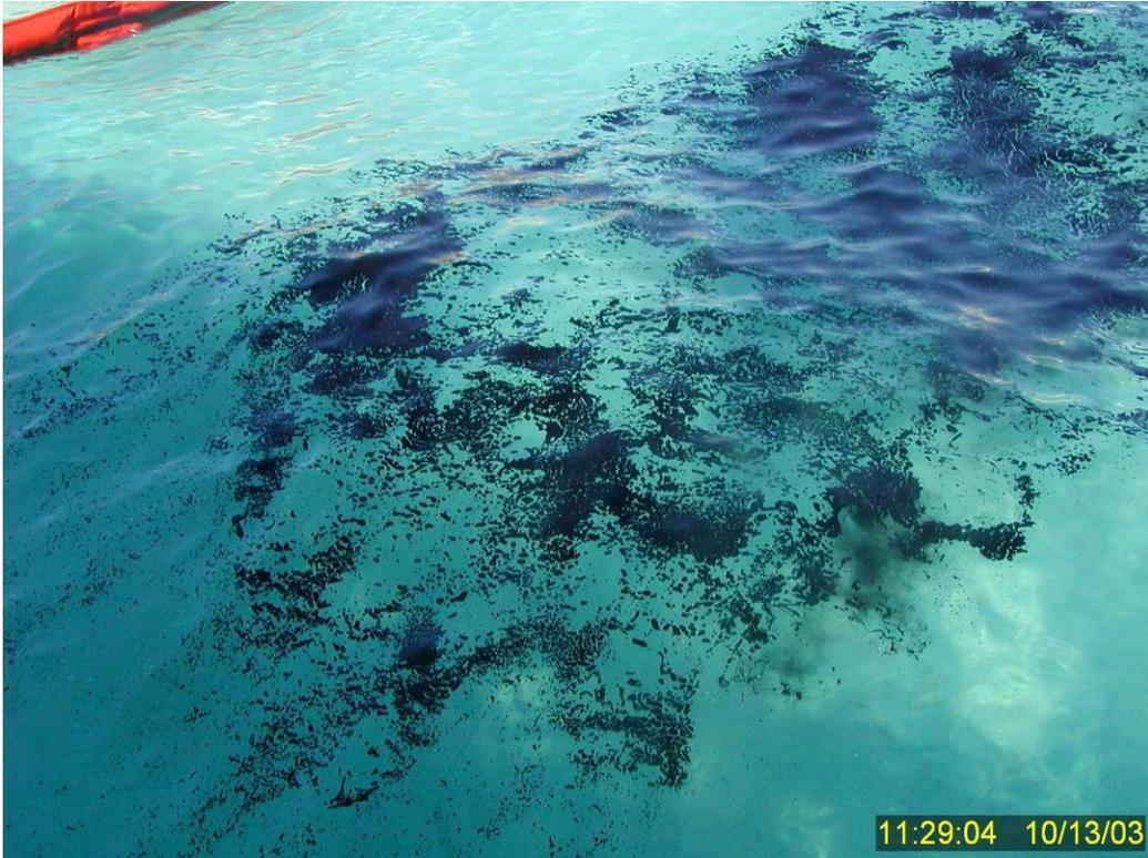
**Figure 27** Test 11: Dispersant-treated IFO 180 ~ 40 seconds into experiment. Note lack of any significant oil entrainment into the water column.
