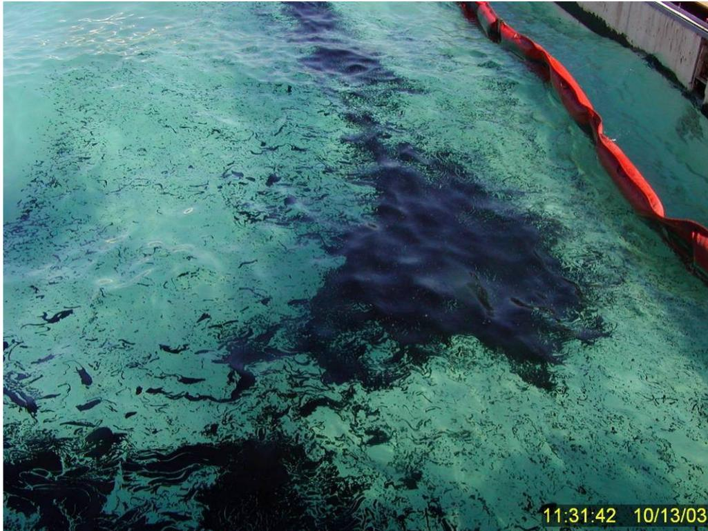
**Figure 31** Test No. 11: Drift of non-dispersing IFO 180 ~ 3.25 minutes after treatment.
