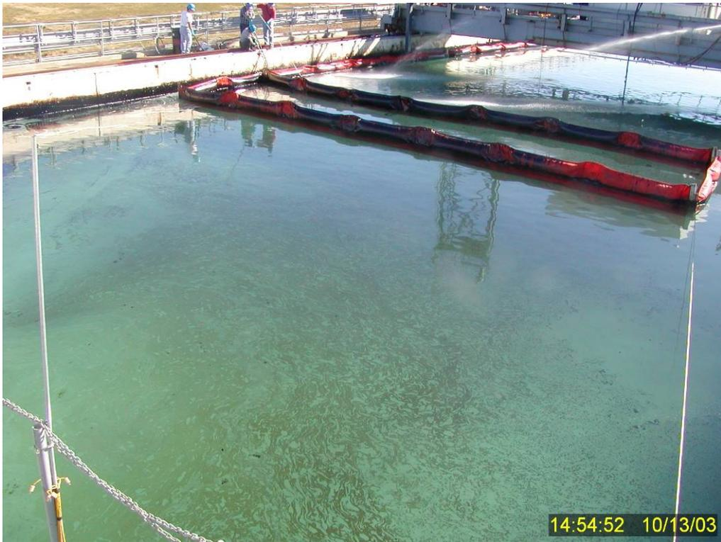
**Figure 57** Splashed-over oil and/or resurfacing dispersed oil outside the containment boom ~ 20 minutes after the termination of wave turbulence at the end of Test No. 12.
