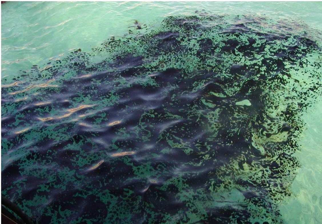
**Figure 16** Untreated IFO 180 control slick (~15-20 seconds after application to the water surface).
