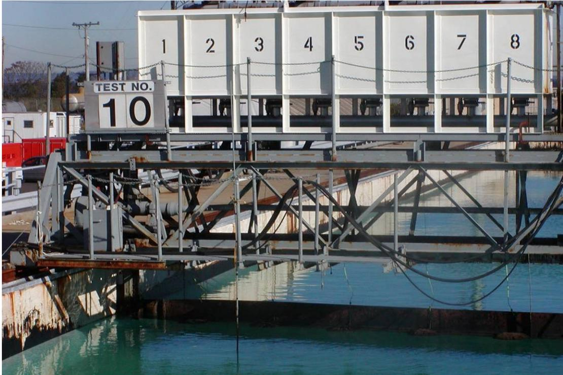
**Figure 13** Test tank before initiation of control test with IFO 180 fuel oil and no dispersant, October 13, 2006. The wave generator had not yet been turned on. Photographed looking north.
