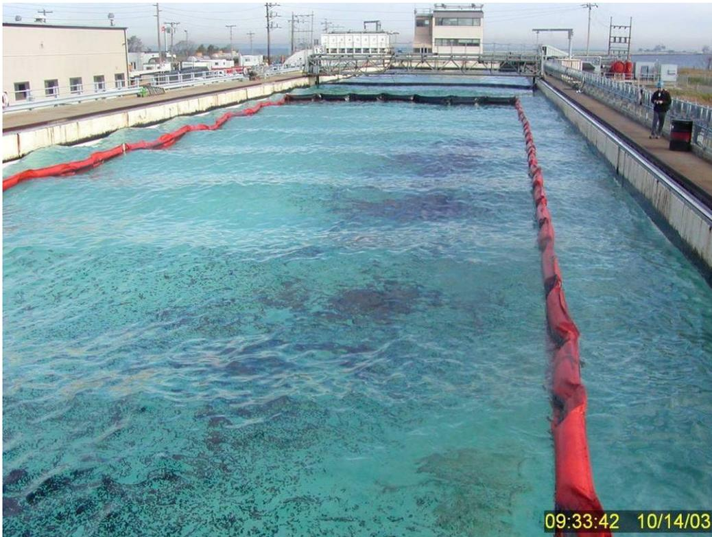
**Figure 67** Surface slick showing no dispersion/entrainment 17 minutes into Test 13.
