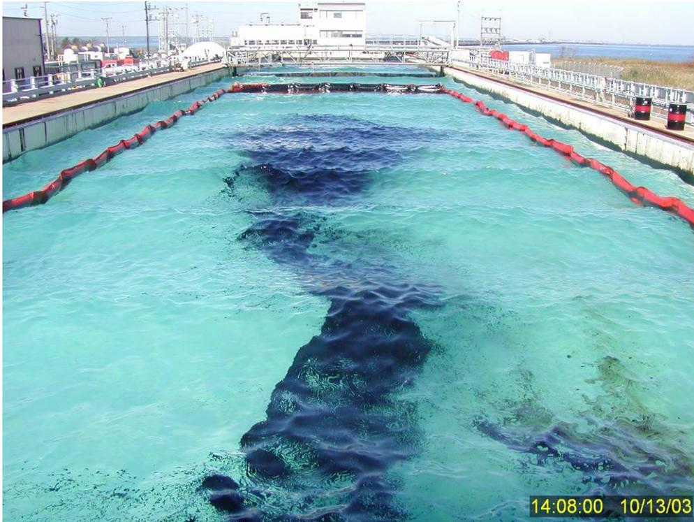
**Figure 43** Test No. 12: IFO 180 four minutes after treatment with Agma dispersant. Note water clarity and lack of significant dispersion/entrainment into the water column.
