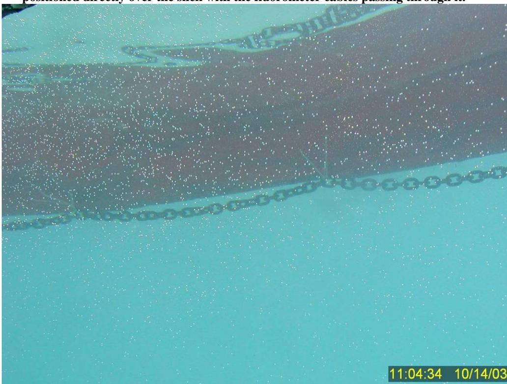
**Figure 70** Underwater view of containment boom and anchor chain showing the water clarity at the end of Test 13.
