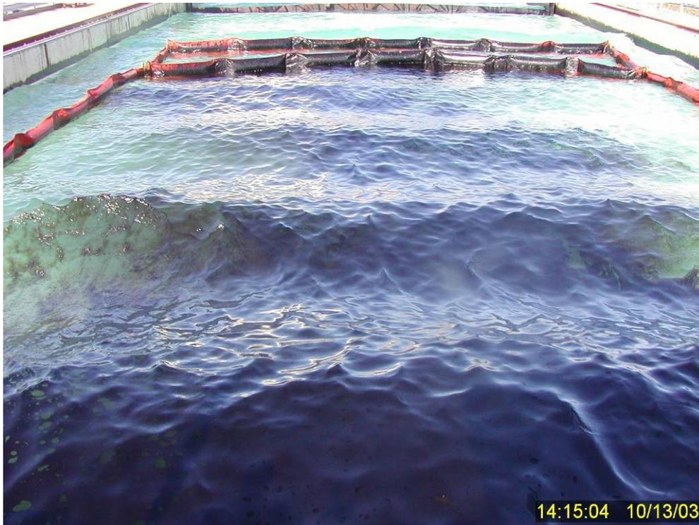
**Figure 47** Gradual breakup of surface oil slick and slow entrainment (dispersion) into water column eleven minutes after dispersant treatment. Note rougher 1-2 inch wave chop on water surface and lateral spread of subsurface dispersed oil plume.
