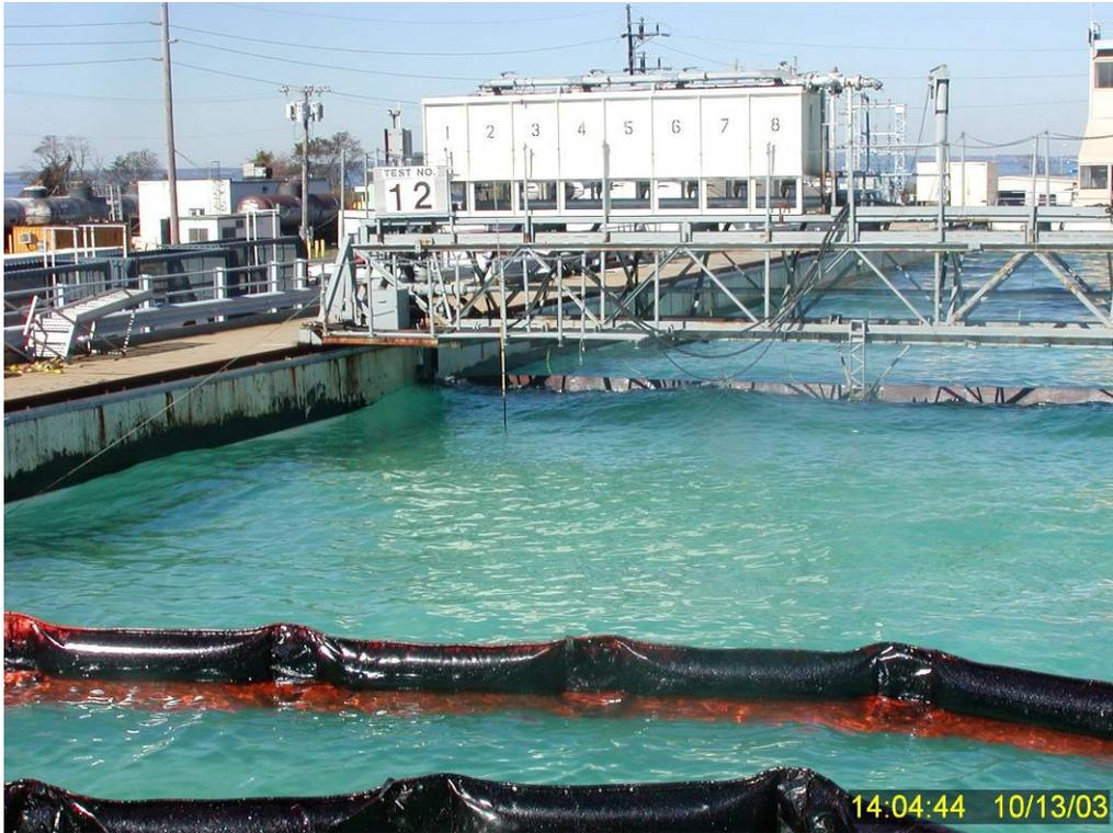
Figure 41 Initiation of Test No. 12: IFO 180 fuel oil treated with Agma at measured DOR of 1:148 and higher-energy waves at 33.3 cpm.
