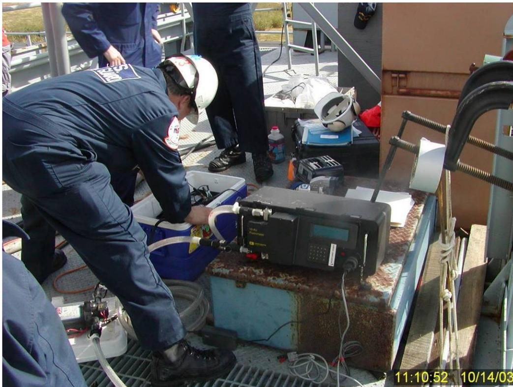
**Figure 74** USCG SMART system fluorometer set up on movable bridge for Visitors Day tests and training.
