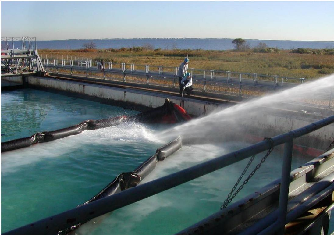
**Figure 10** Removal of remaining surface oil from inside secondary containment boom before test initiation on October 13, 2003.
