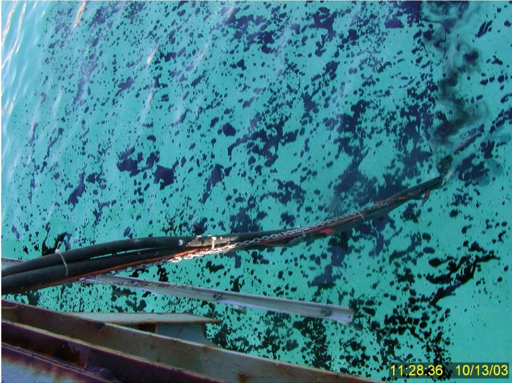
Figure 25 Test No. 11: Dispersant spray boom and in situ fluorometer cable 14 seconds into test.
