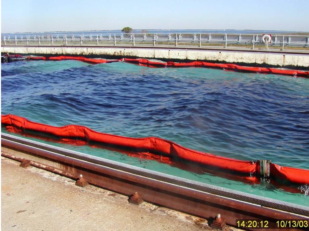
**Figure 49** Poorly dispersed subsurface oil and surface oil residues viewed from the side of the wave tank 16 minutes after initiation of Test Number 12.
