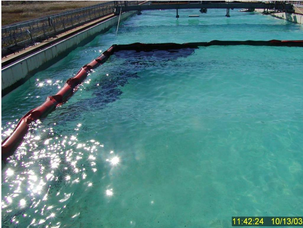
Figure 33 Test No. 11: Non-dispersed IFO 180 fuel oil driven by wind to south-east corner of experimental containment boom. Note the water clarity and the lack of any oil outside the test area.
