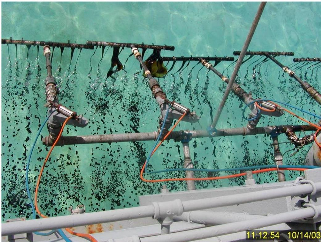
Figure 75 Application of IFO 180 to water surface for Test No. 14 initiation at ~1113 hrs 14 October 2003.
