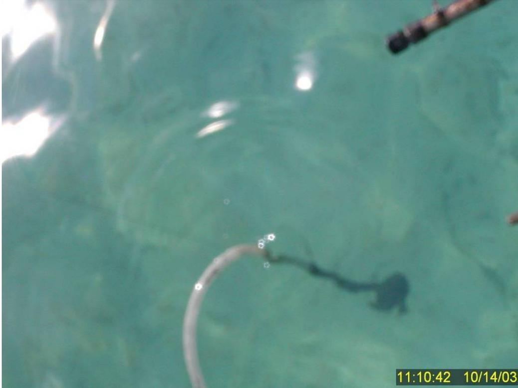
**Figure 73** Submersible pump for USCG SMART fluorometer system deployed from the movable bridge.
