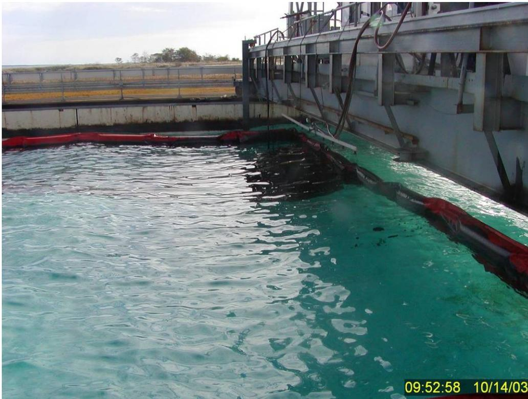
**Figure 69** With very light winds from the north, most of the oil drifted to the southeast corner of the containment boom (against the prevailing wave train). This photo shows the movable bridge positioned directly over the slick with the fluorometer cables passing through it.
