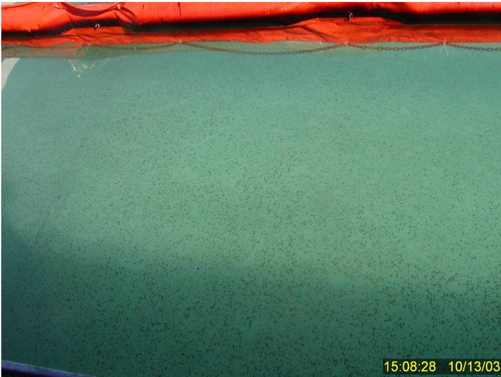
**Figure 58** Resurfacing dispersed oil between the western tank wall and containment boom approximately 35 minutes after termination of wave turbulence at the end of Test No. 12.
