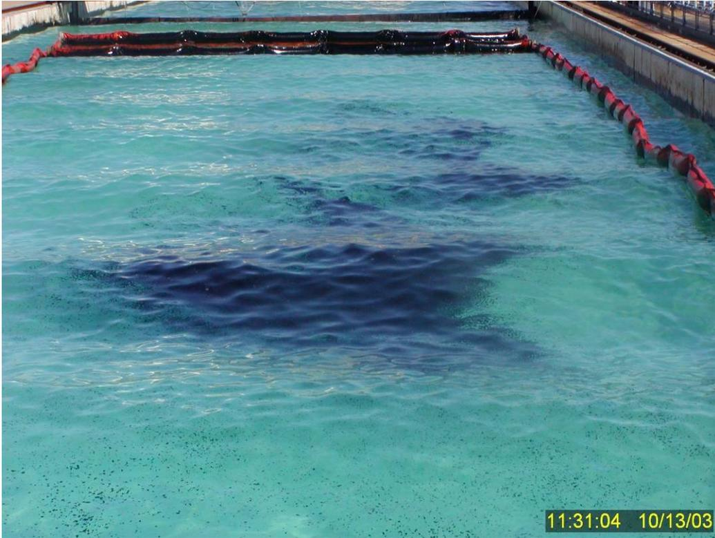
**Figure 29** Test No. 11: Still no dispersion/entrainment ~ 2.5 minutes after dispersant treatment.
