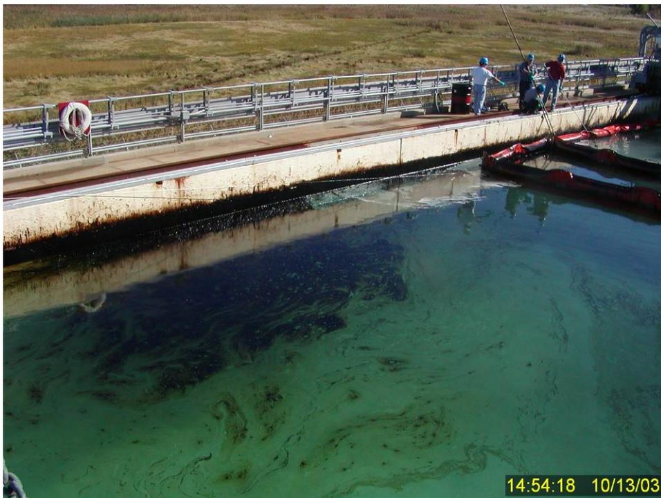
**Figure 56** Residual surface oil outside both the primary and secondary containment booms 20 minutes after the cessation of turbulence at the conclusion of Test No. 12 (see also Figure 55). Presumably this was from partially-dispersed oil that was entrained by increased turbulence around the containment boom during the test, although it may also have been lost due to splash-over.
