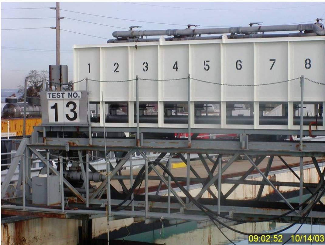
**Figure 62** Preparations for Test 13 on “visitors day” 14 October 2003: IFO 180 fuel oil, Superdispersant 25 (DOR 1:130), and low-energy wave turbulence at 30 cpm.
