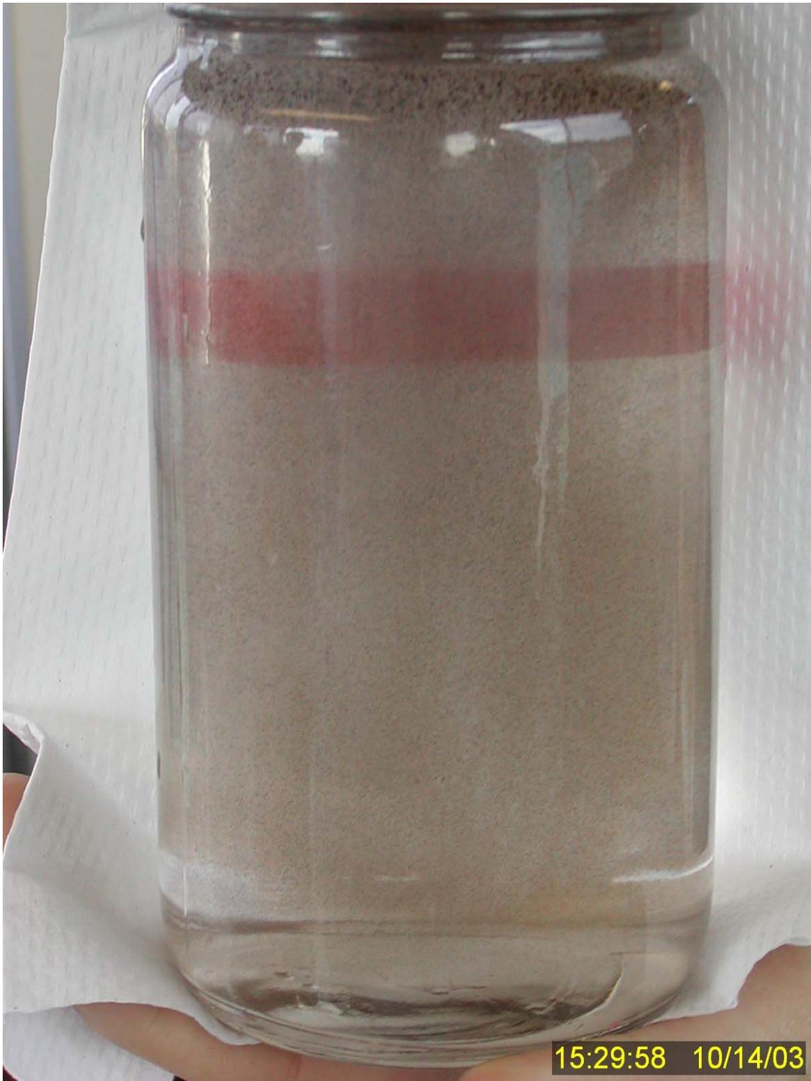
**Figure 142** Grab sample of water tapped from the discharge line of the 1-meter Turner AU-10 fluorometer. This sample was collected after approximately eleven and one-half minutes for detailed chemical analysis of oil content for direct comparison to the fluorometer reading. Note the visible dispersed oil droplets throughout the sample.
