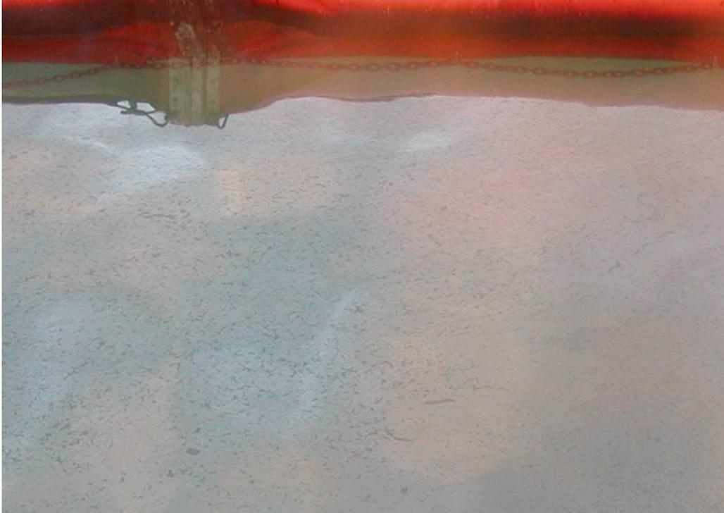
**Figure 170** Close up of silver sheen and 0.5 – 1 cm sized surface oil agglomerates between the containment boom and western tank wall from area outlined by the yellow rectangle in Figure 169. The colors are from the reflections of the clouds at sunrise and not thicker colored oil films.
