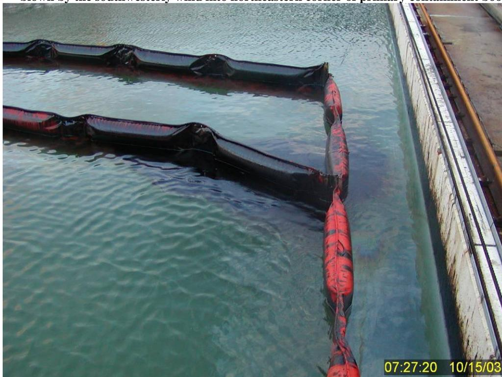
**Figure 173** Close up of the accumulated silver sheen and re-surfaced oil that had been blown overnight into the northeast corner of the primary and secondary containment boom.
