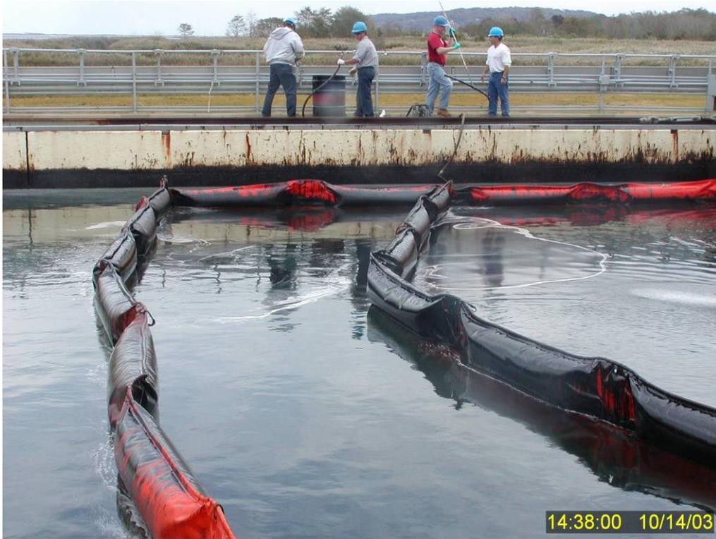
**Figure 119** Residual nondispersed oil within the test area being herded for recovery after Test No. 15.
