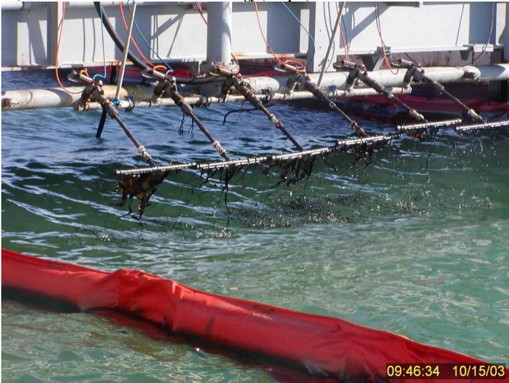
**Figure 179** Application of lower viscosity IFO 120 fuel oil to water surface at beginning of Test No. 17.
