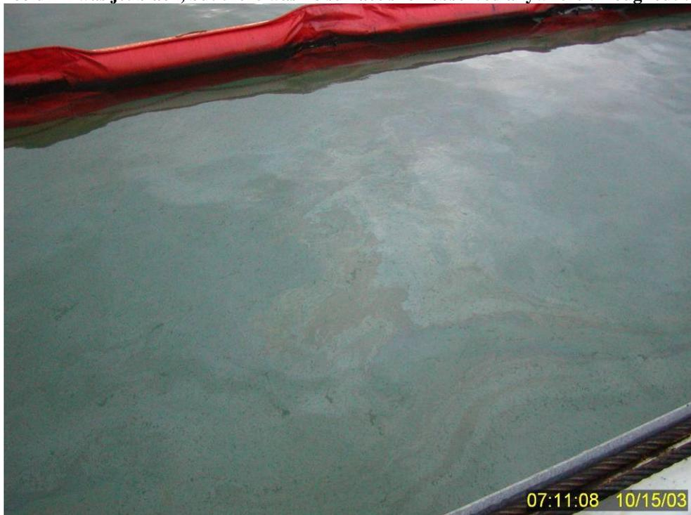
**Figure 161** Resurfaced oil sheen between western tank wall and containment boom 15 hours after cessation of turbulence at the end of Test to. 16. Photo taken early the next morning before any tank cleaning operations had been initiated.
