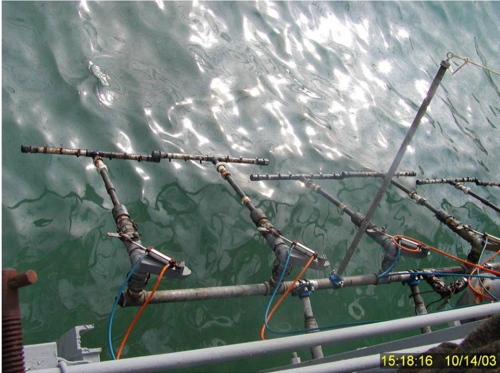
Figure 127 Discolored water and residual surface sheen from previous test (No. 15) terminated an hour earlier.
