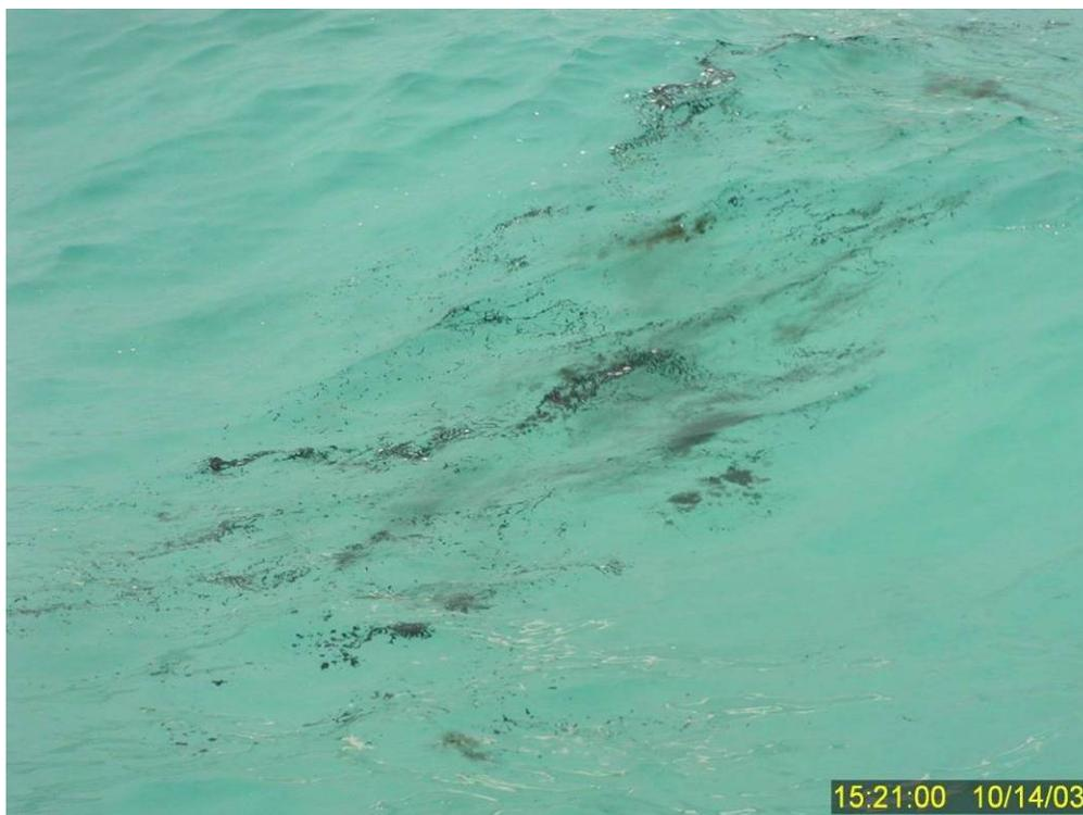
**Figure 135** Close up of the yellow rectangle in Figure 134 as it begins to disperse into the water column two and one-half minutes after dispersant treatment. Note the water color before the majority of the oil begins to disperse.
