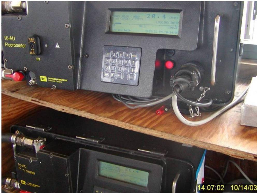
**Figure 115** Real-time readout of measured dispersed oil concentrations from the 1- and 2-meter sampling lines (20.4 and 26.4 ppm, respectively) attached to the Turner 10-AU fluorometers on the movable bridge. In previous tests where no dispersion occurred these instruments both consistently read 0.0 ppm.
