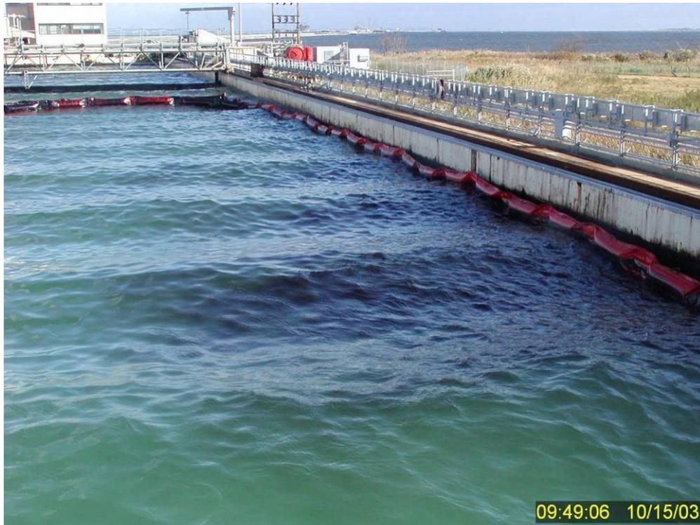
**Figure 182** IFO 120 fuel oil two minutes after dispersant treatment. With the strong westerly winds, the surface oil quickly drifted toward the east (note the containment boom is being pressed hard against the tank wall); however, the dispersed oil remained more in the center of the tank.
