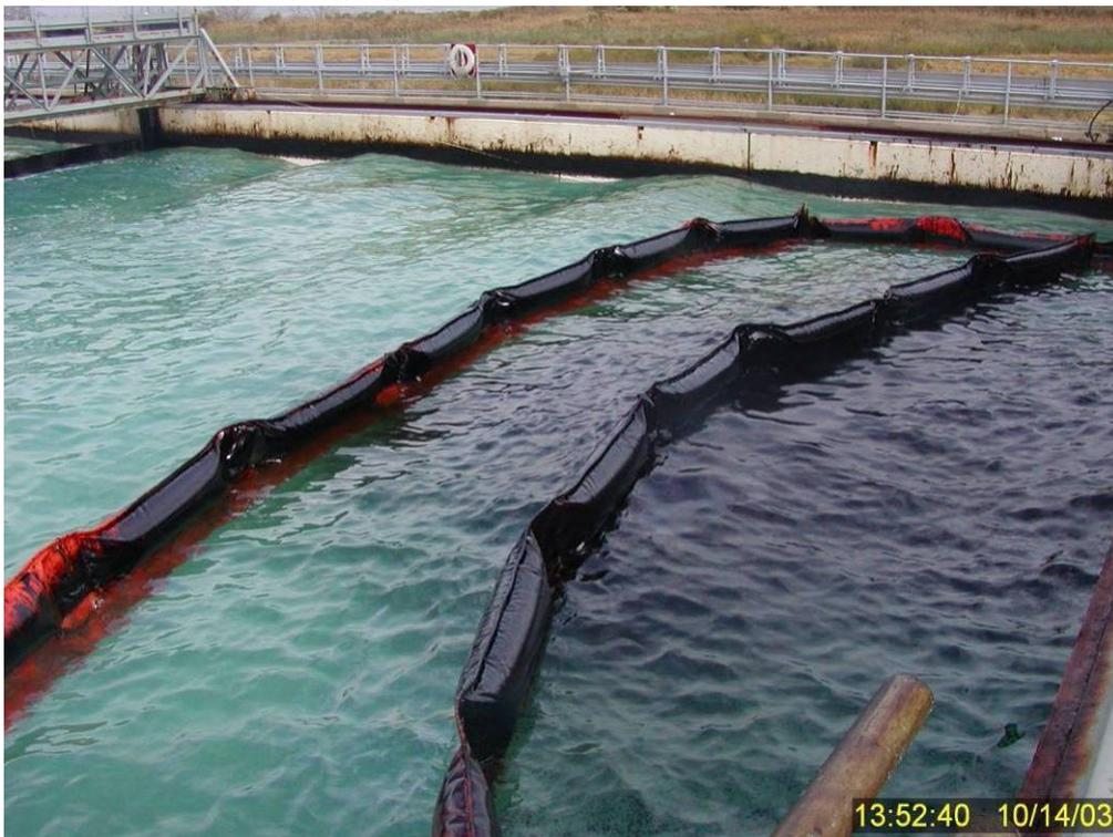
**Figure 110** Residual (nondispersed) surface oil against the northern containment boom and slowly diffusing subsurface dispersed oil within secondary containment area and in water at the bottom of the figure seven minutes into Test No. 15.
