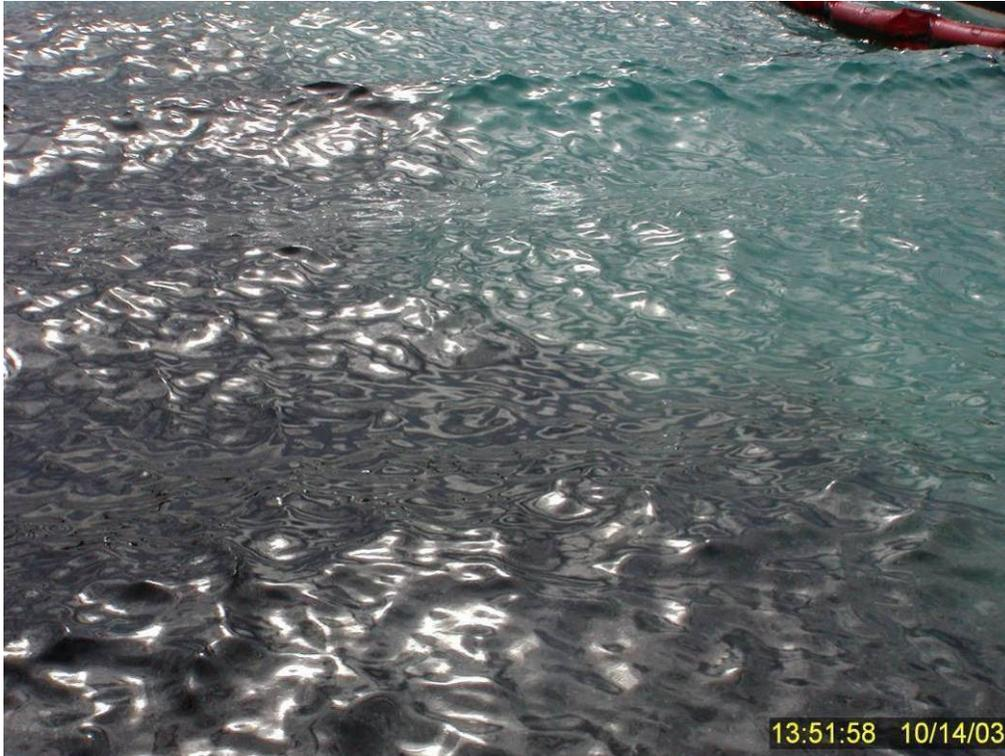
**Figure 109** Dispersed oil plume diffusing toward eastern containment boom in center of test area six and one-half minutes into Test No. 15.
