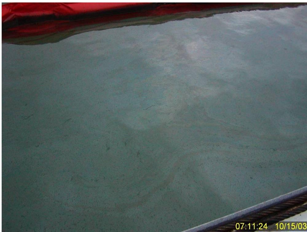
**Figure 162** Resurfaced oil sheen and droplets outside of secondary containment boom 15 hours after Test No. 16. The tank had been allowed to stand undisturbed overnight, and this photograph was taken before any OHMSETT personnel had arrived to initiate additional clean up operations.
