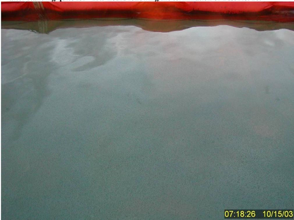
**Figure 167** Oblique photograph of silver oil sheen on water surface from Figure 166 (photographed at a 90 degree angle to the containment boom).
