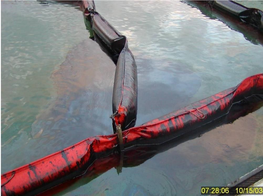
**Figure 174** Resurfaced oil in the northeast corner of the containment boom photographed from the eastern tank wall 15.5 hours after cessation of turbulence at the end of Test No. 16.
