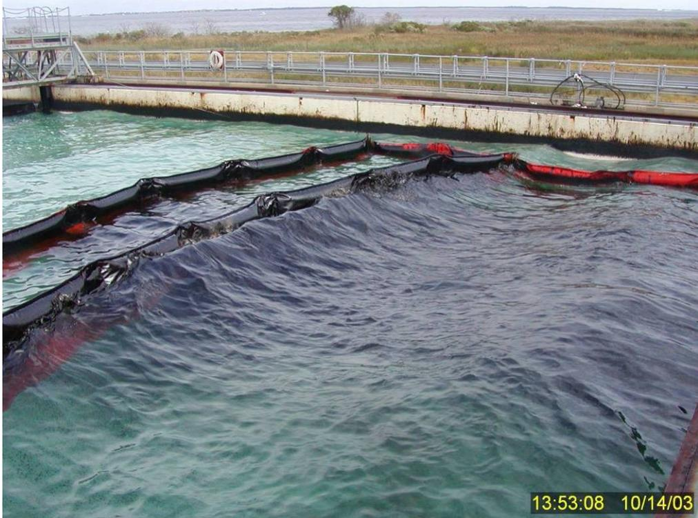
**Figure 111** Laterally spreading subsurface dispersed oil plume near north end of test area eight minutes into Test No. 15.
