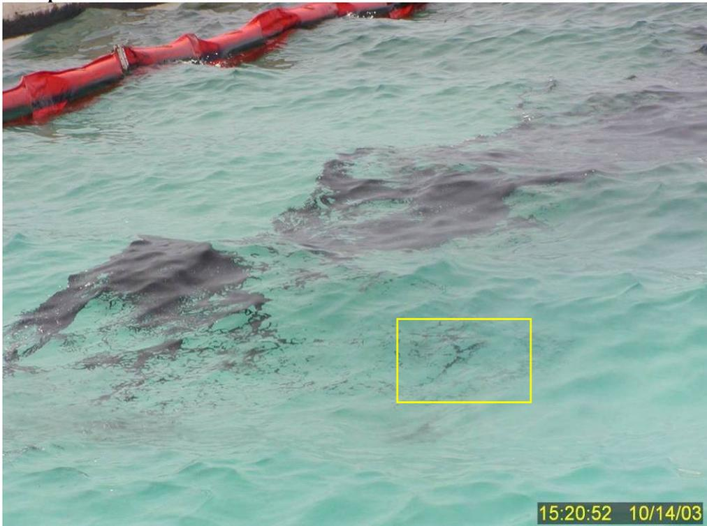
**Figure 134** Overhead view of dispersant-treated surface slick approximately two and one-half minutes after dispersant application. See Figure 135 for a close up of the area in the yellow rectangle as it begins to break up and become dispersed.
