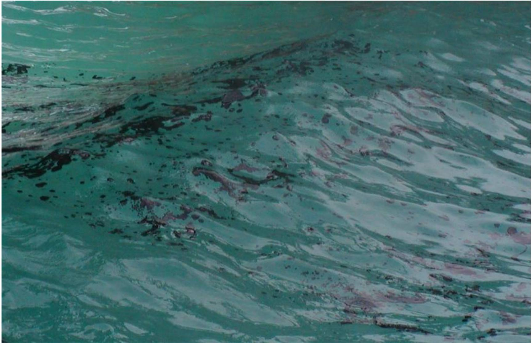
**Figure 100** Close up of water surface and IFO 180 fuel oil directly under the dispersant spray bar in Figure 98. Note the dispersant spray velocity is not sufficient to force the oil into or under the water surface.
