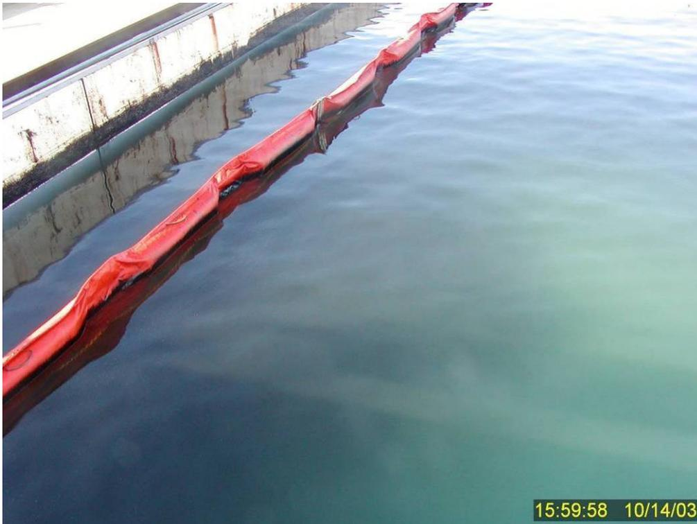
**Figure 152** Subsurface dispersed oil plume along western edge of containment boom and tank wall approximately seven minutes after cessation of wave turbulence for Test No. 16.
