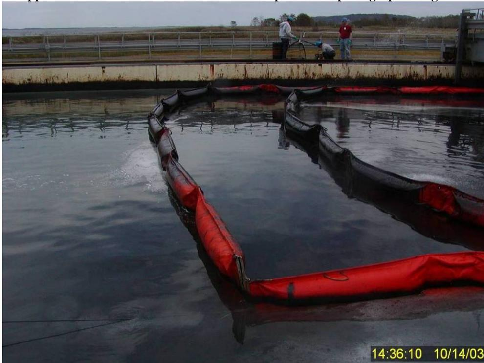
**Figure 118** The water throughout the test tank (both inside and outside the containment booms) was still jet black twenty minutes after the wave turbulence was terminated at the end of Test No. 15. Note there was some silver sheen observed on the water surface, but there was no evidence of massive oil resurfacing like that observed at the end of Test No. 12 with a poorer performing dispersant (see Figures 55 and 56 for comparison).
