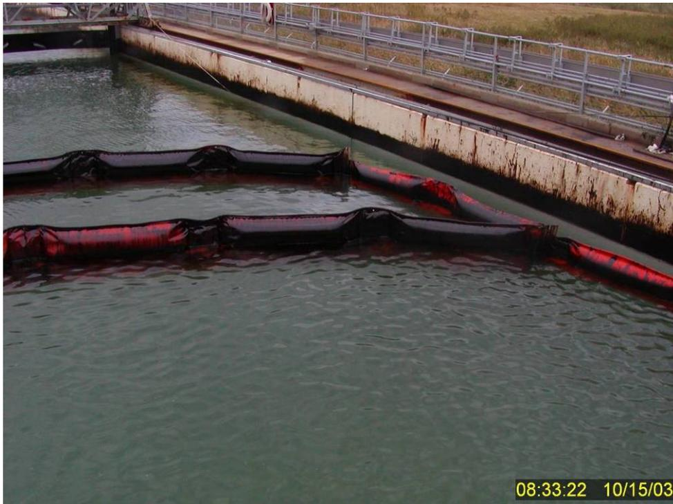
**Figure 176** Subsurface dispersed oil imparting a dark green/black hue to the water column after 16.5 hours of relative calm and removal of the residual surface oil by OHMSETT personnel in preparation for additional tests scheduled for October 15, 2003. Photographed an hour after Figures 174 and 175 from the movable bridge looking north northeast.
