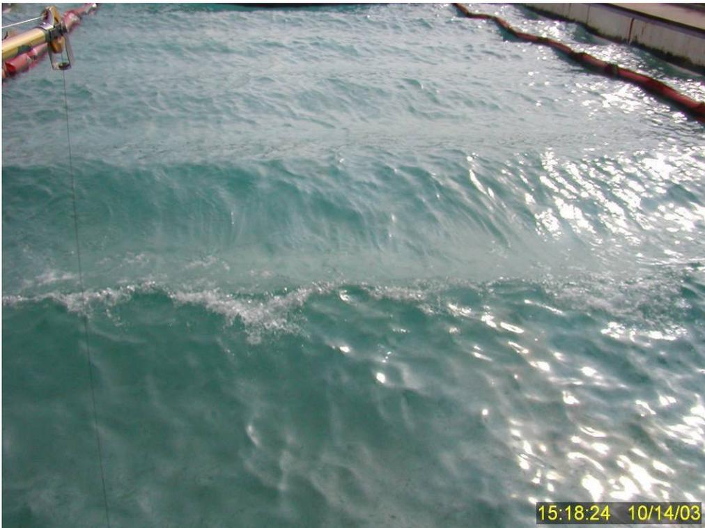
Figure 128 Wave train established for Test No. 16 just before oil addition. Note single cresting wave passing under movable bridge.
