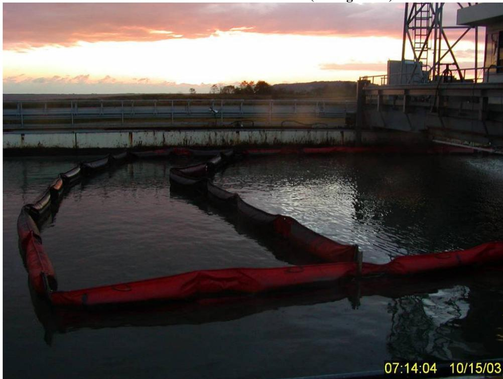
**Figure 165** Undisturbed water surface inside secondary containment boom and north end of test zone 15 hours after termination of Test No. 16.
