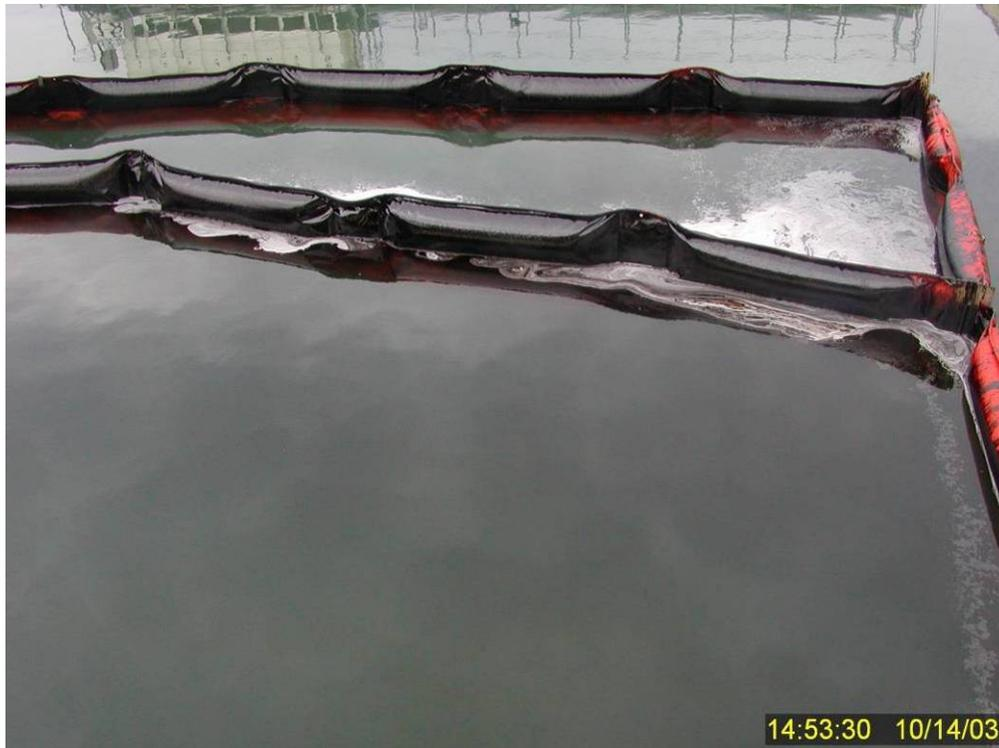
**Figure 125** Subsurface dispersed oil discoloration of the tank water 38 minutes after stopping the wave turbulence and sweeping the tank to remove residual surface oil at the end of Test No. 15. Note there is some minor sheen adjacent to the primary containment boom near the top of the figure, but massive dispersed-oil resurfacing like that observed after Test No. 12 did not occur.
