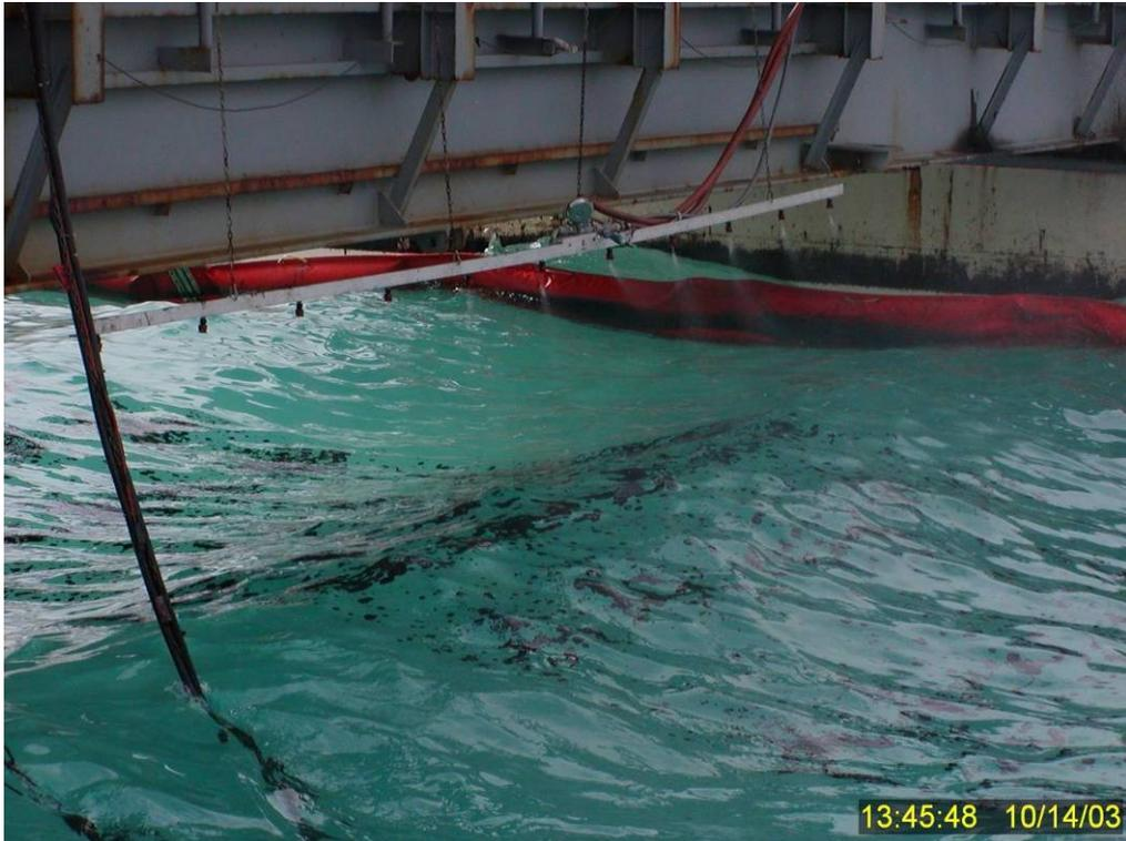
Figure 98 Passing wave moving under the dispersant spray bar 14 seconds after initiation of Test No. 15.
