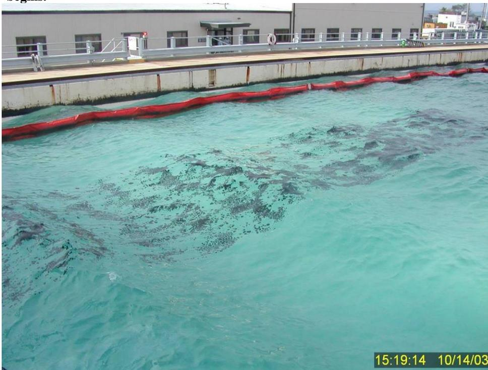
**Figure 132** Appearance of the IFO 180 fuel oil approximately 30-45 seconds after treatment with Corexit 9500. Note the water clarity appears better from this angle (looking north) compared to the view toward the south just before the initiation of the test (Figures 127 and 128).
