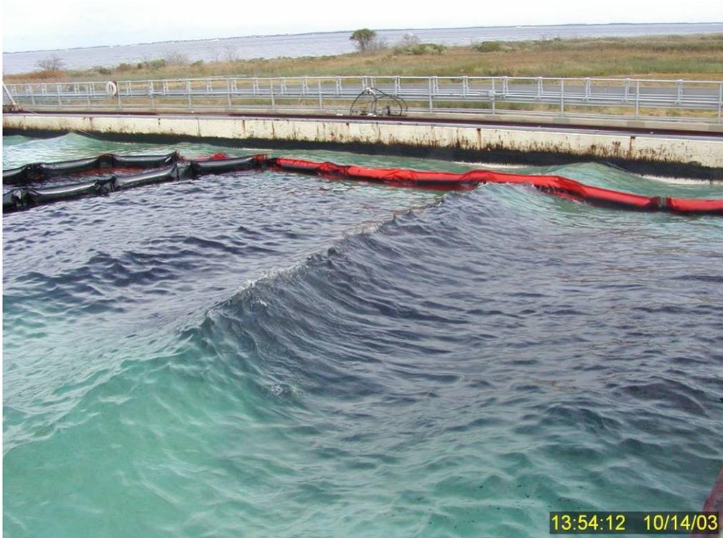
**Figure 112** Subsurface dispersed oil plume throughout center of test tank ~ nine minutes into Test No. 15.
