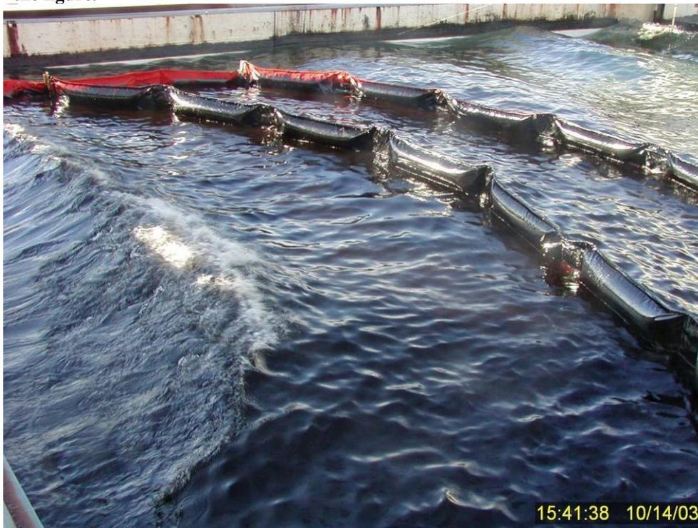
**Figure 147** Primary and secondary containment boom showing little or no surface oil and the distribution of dispersed subsurface oil across the tank 23 minutes after dispersant treatment.
