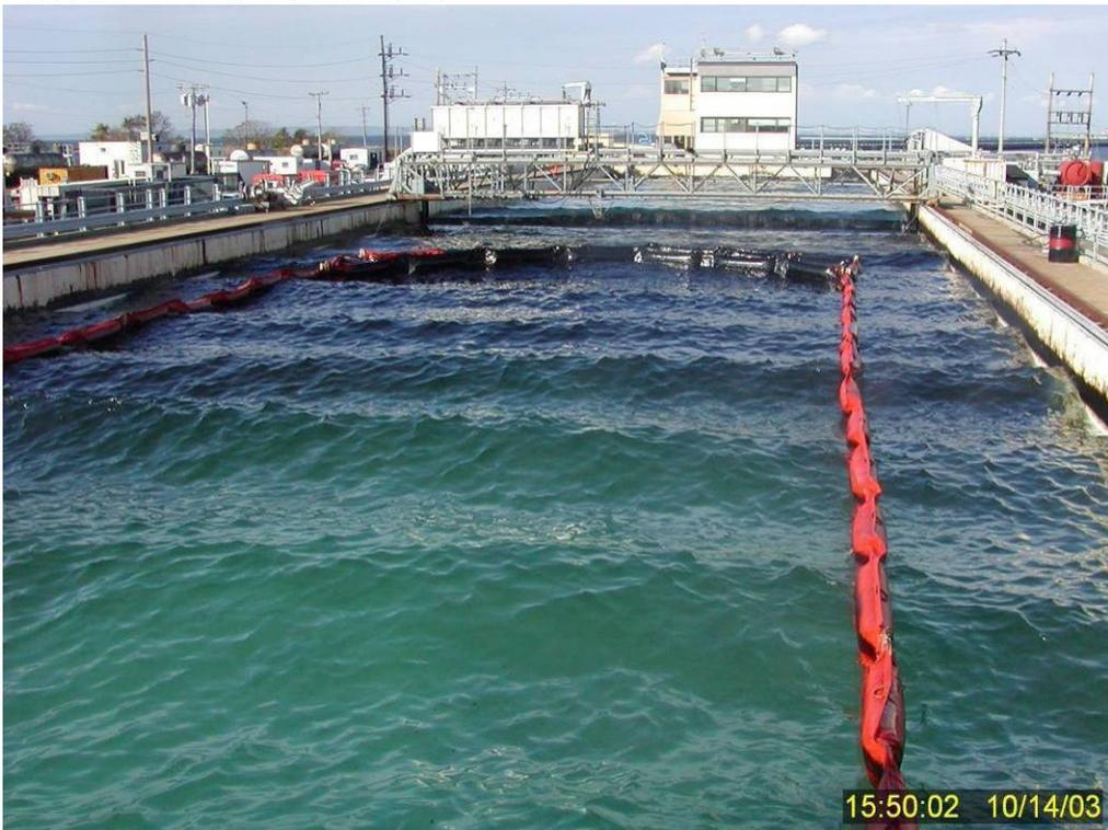
**Figure 149** Overview of test tank 32 minutes into Test No. 16 showing dispersed oil plume diffusing laterally and longitudinally throughout the tank.
