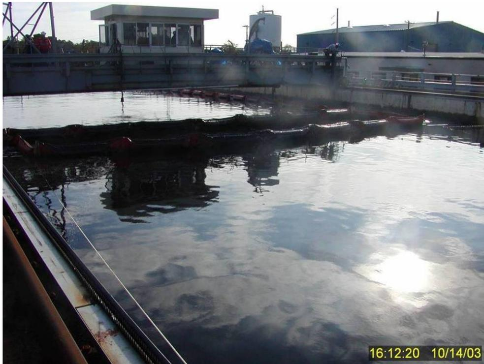
**Figure 160** Surface water and dispersed oil plume to the north of the primary and secondary containment booms 19 minutes after the wave turbulence was stopped at the termination of Test No. 16. No significant resurfacing of dispersed oil was observed after this test like it was with the poorer performing dispersant at the termination of Test No. 12 (see Figure 56). At this time, the water column was jet black, but there was no surface slick observed anywhere throughout the tank.
