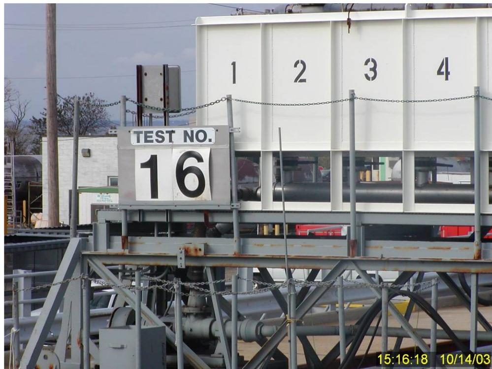
**Figure 126** Set up for Test No. 16: IFO 180 treated with Corexit 9500 (nominal DOR 1:50) at intermediate wave energy (33 cpm).
