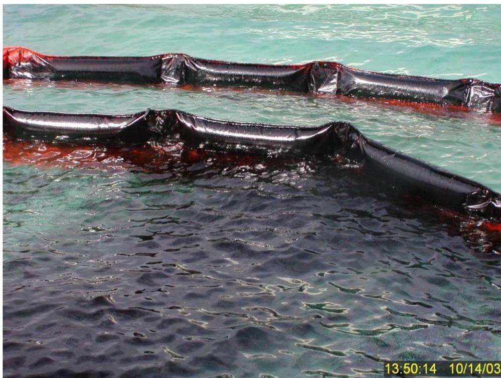
**Figure 105** Surface and slightly entrained subsurface oil in contact with the containment boom at the north end of the test tank four and one-half minutes into Test No. 15.
