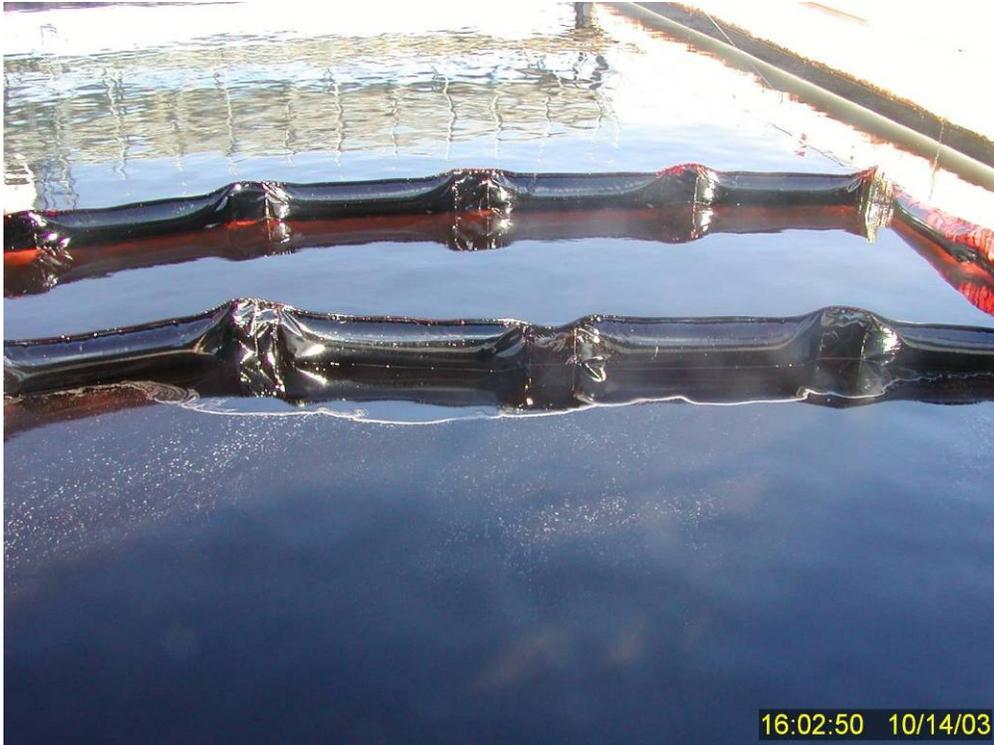
**Figure 154** Close up of minor residual surface oil remaining within the primary containment boom at the termination of Test No. 16.
