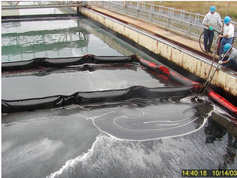
**Figure 121** Vacuum recovery of residual surface oil remaining inside the primary containment boom at the termination of Test No. 15.
