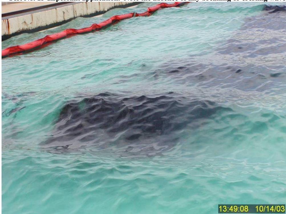
**Figure 102** Closer view of dispersant-treated oil as it continues to spread three and one-half minutes into Test No. 15.
