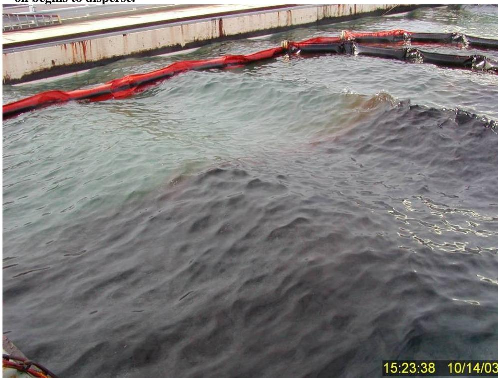
**Figure 136** Bulk oil in center of tank beginning to disperse approximately five minutes after dispersant treatment.
