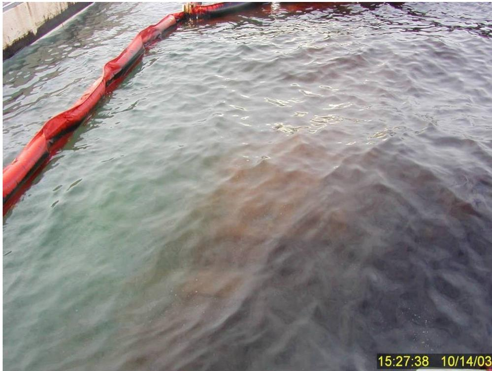
**Figure 139** More traditional lighter brown plume of subsurface dispersed oil plume nine minutes after dispersant treatment in Test No. 16. It is believed that the lighter color may be due to smaller dispersed oil droplets, but droplet size data are not available to confirm this hypothesis.
