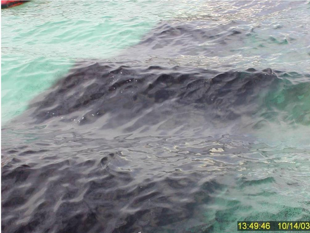
**Figure 103** Overhead view of dispersant treated oil actually beginning to be entrained below the water surface. Note, this is being facilitated by the stretching and pulling of the slick by the passing waves, not by cresting of breaking whitecaps per se.
