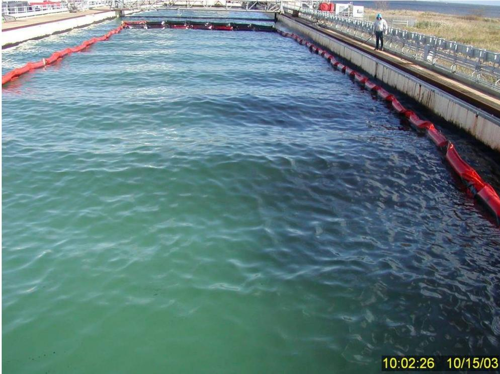
**Figure 187** Dispersed IFO 120 oil plume over eastern half of the tank approximately 15 minutes after initiation of Test No. 17.
