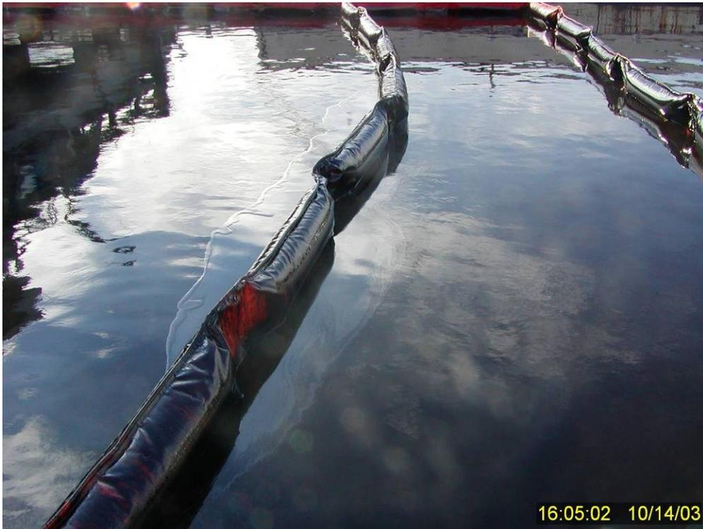
**Figure 155** Residual surface oil and subsurface dispersed oil plume within primary and secondary containment booms at the end of Test No. 16.
