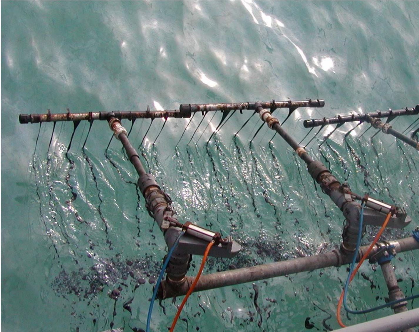
**Figure 130** Close up of IFO 180 fuel oil being dribbled onto water surface at initiation of Test No. 16. Note the lack of oil penetration into the water at this low application rate and the presence of broken silver sheen from Test No. 15 on the water surface at the top of the photograph.
