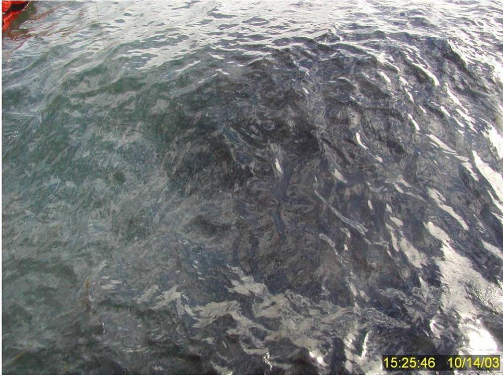
**Figure 137** Subsurface oil plume approximately in the middle of the tank and 6-7 feet from the western containment boom. Photo was taken looking to the north seven minutes after dispersant treatment in Test No. 16.
