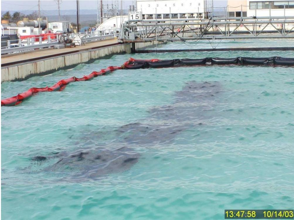
**Figure 101** Appearance of dispersant-treated slick in center of the wave tank two and one-half minutes after Test No. 15 dispersant application. Note the absence of any breaking or cresting waves.
