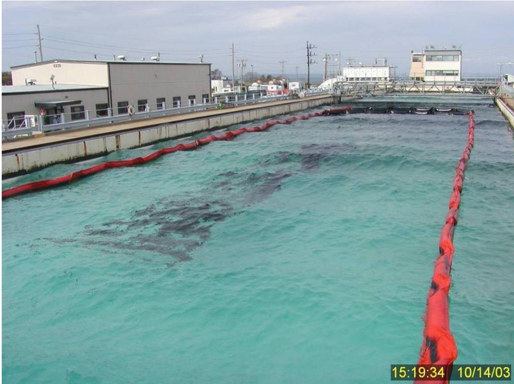
**Figure 133** Dispersant-treated slick in the center of the tank one minute after initiation of Test No. 16.
