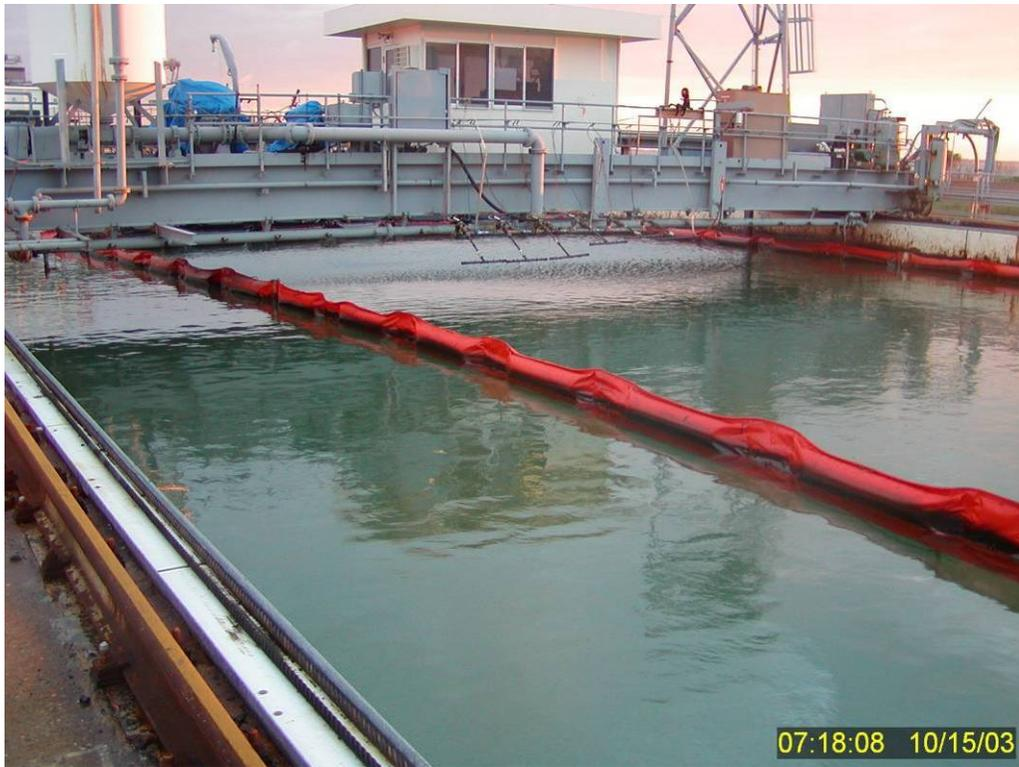
**Figure 166** Undisturbed water surface between western tank wall and containment boom in center of tank after standing quite for ~15.5 hours following the termination of Test No. 16.
