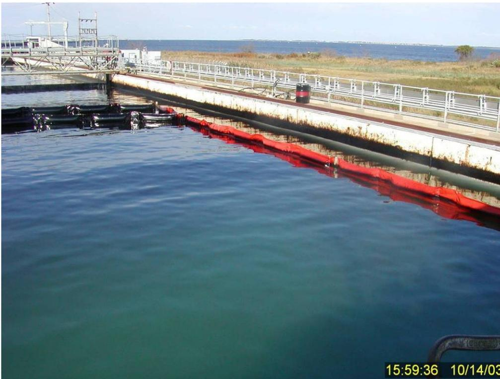
Figure 151 Water surface and green-black subsurface dispersed oil plume approximately six minutes after the wave turbulence for Test No. 16 was stopped (41 minutes after dispersant addition).
