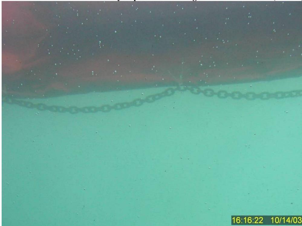
**Figure 157** Water clarity as observed from the southern-most underwater window (closest to the wave generator) where the containment boom and anchor chain 8-10 feet from the window can still be observed 23 minutes after terminating the wave turbulence for Test No. 16.
