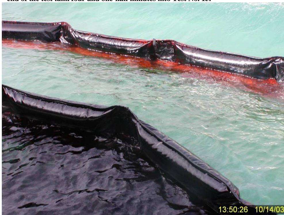
**Figure 106** Surface and slightly entrained oil at north end of containment boom five minutes into Test No. 15. Note the clean water in the secondary containment boom showing the lack of any oil “splash over” and only limited diffusion of subsurface dispersed oil up to this time (compare to Figure 107 taken 22 seconds later).
