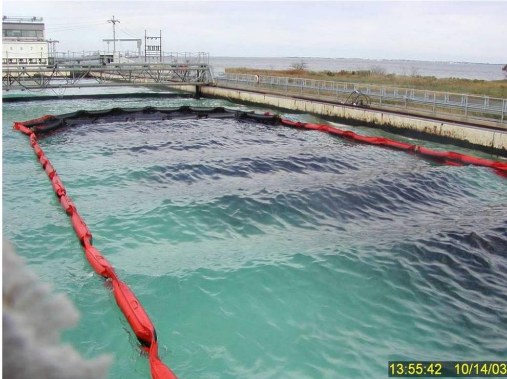
Figure 113 Subsurface dispersed oil plume throughout test tank 10 minutes into Test No. 15. Note the subsurface oil is not subject to wind drift and it is not driven by the waves into the north end of the test enclosure. Compare to surface slick appearance for non-dispersed oil in Figure 66.
