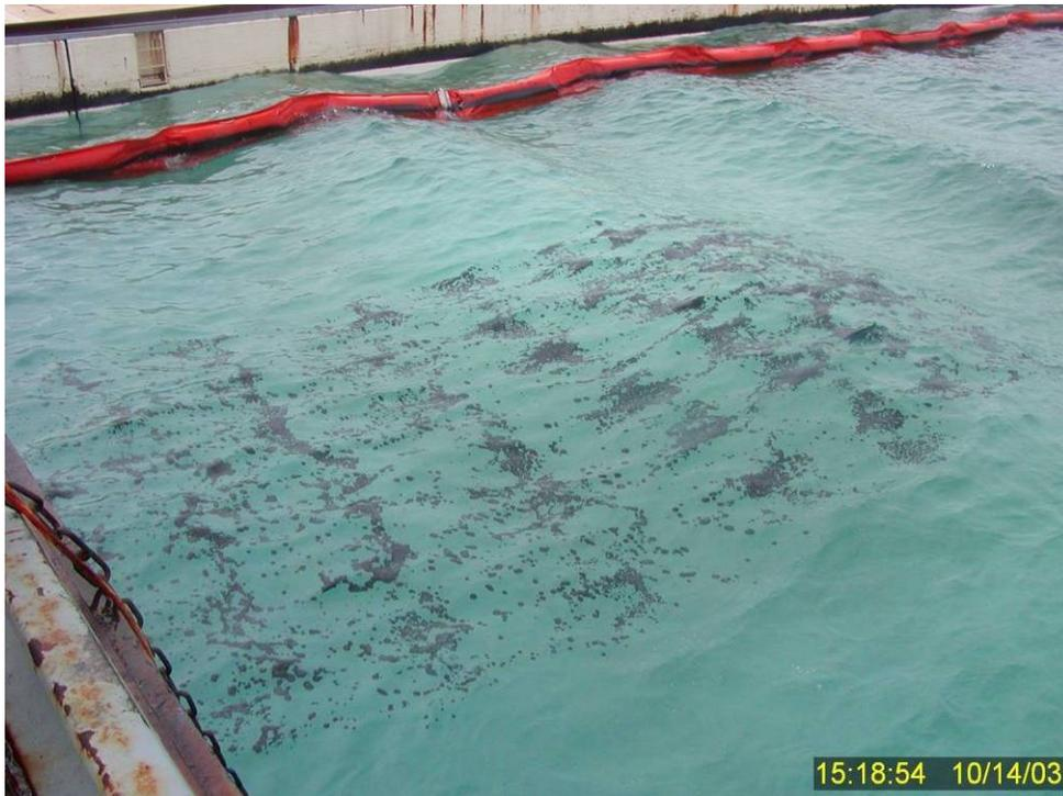
**Figure 131** Appearance of the IFO 180 immediately after passing under the dispersant spray boom 20 seconds into Test No. 16. Note the uneven distribution of the oil on the water surface resulting in under dosing by the dispersant spray. Also note the water color before any significant dispersion begins.
