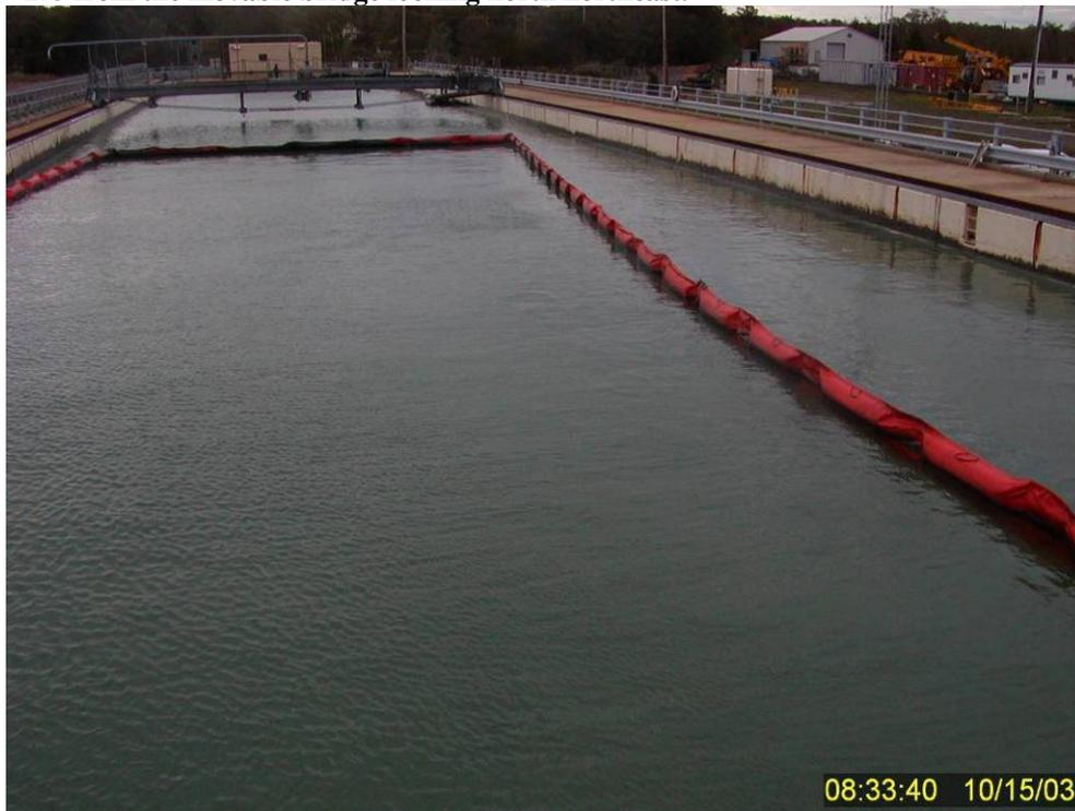
**Figure 177** View of the containment boom (looking towards the south from the movable bridge) after the tank had been cleaned of residual resurfaced oil in preparation for additional tests on October 15, 2003. Although the wind blowing from the west (right to left) has bowed the primary containment boom, it does not impart a lot of wave energy to the tank.
