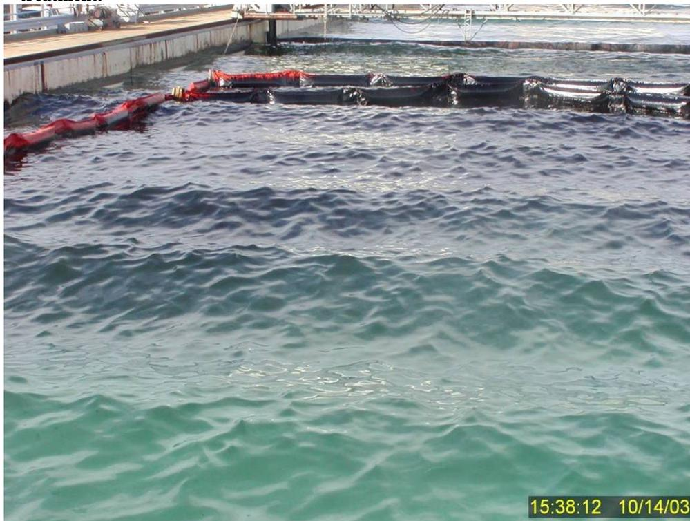
Figure 145 Overview of the water surface and dispersed oil plume 20 minutes into Test No. 16. Note the virtual absence of any surface oil and the lateral diffusion of the dispersed oil plume outside (to the left of) the containment zone.
