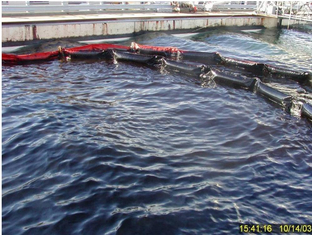
**Figure 146** North end of the experimental test zone 23 minutes into Test No. 16. There is little or no visible surface oil, and the dispersed oil plume can be seen outside the containment boom on the top of the figure.
