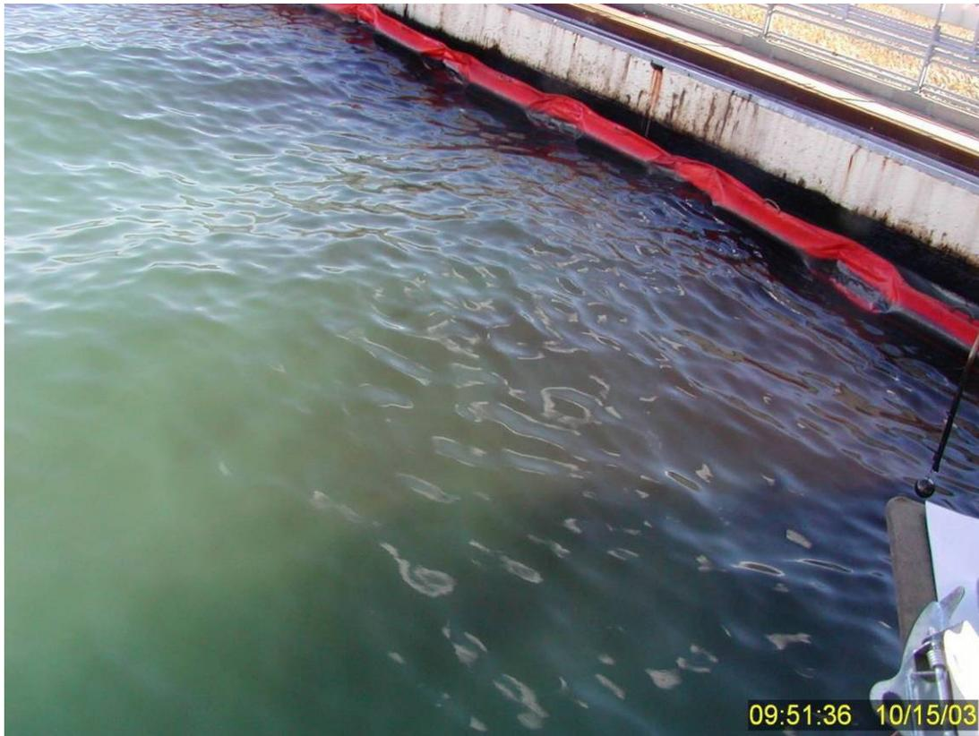
**Figure 184** Subsurface dispersed oil plume approximately four and one-half minutes after dispersant treatment in Test No. 17. Note this lighter IFO 120 oil (viscosity = 1,145 cP @ 16° C) dispersed much more readily than the IFO 180 oil (2,075 cP @ 16° C) treated with the same dispersant, DOR, and wave energy during Test No. 14. See Table 1 and Figures 72 through 91.
