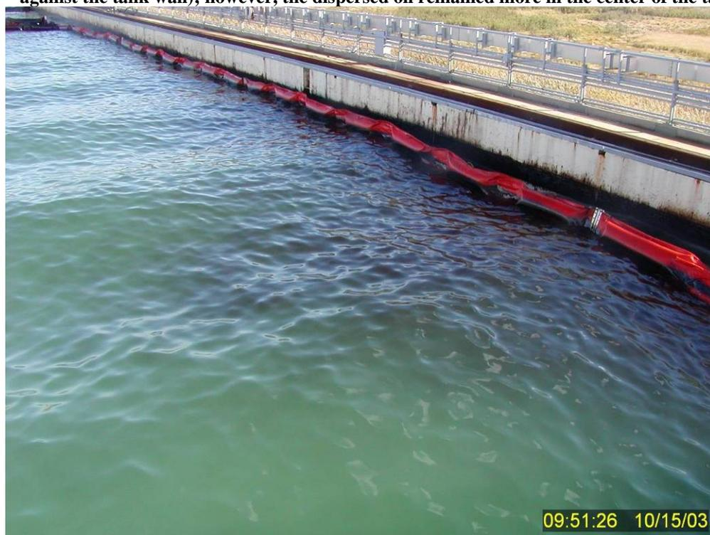
**Figure 183** Dispersed oil plume and residual non-dispersed surface oil (immediately adjacent to the boom) approximately four minutes after dispersant treatment in Test No. 17.
