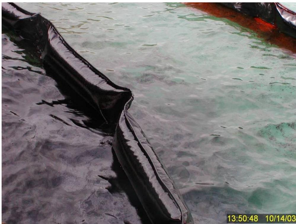
**Figure 107** Initial diffusion of subsurface dispersed oil plume into secondary containment boom five and one-half minutes into Test No. 15 (compare to Figure 106 taken 22 seconds earlier).
