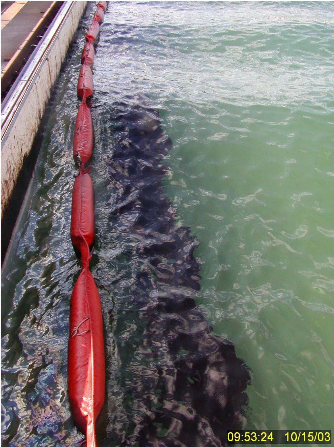
**Figure 185** Residual non-dispersed surface oil blown against the containment boom along the eastern side of the tank approximately 6 minutes after the initiation of Test No. 17.
