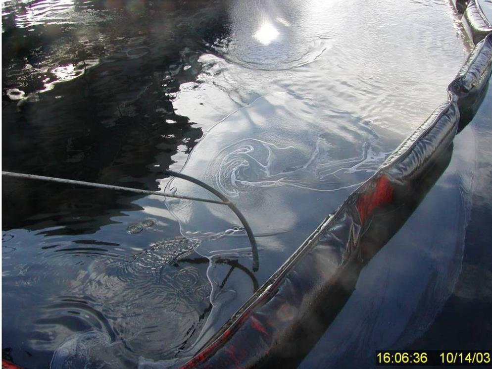
**Figure 156** Squeegee/vacuum recovery of residual surface oil within the primary containment boom at the termination of Test No. 16. Only 16 percent of the original oil was recovered (Table 1).
