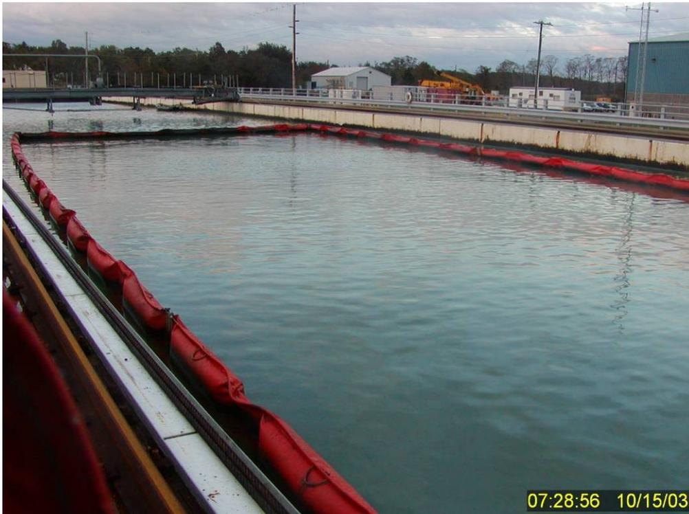
**Figure 175** View of the primary containment zone looking toward the southwest approximately 15.5 hours after the wave generator was turned off at the end of Test No. 16. The water surface was relatively free of oil (it had all been blown into the northeast corner by the prevailing winds), but the subsurface was still very dark due to the dispersed oil that remained in suspension overnight.
