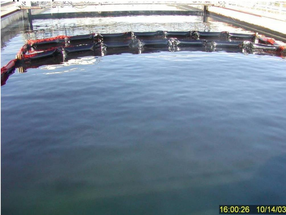
**Figure 153** Center of tank test area showing dispersed oil cloud and absence of any significant surface oil before tank cleaning operations were initiated at the end of Test No. 16.
