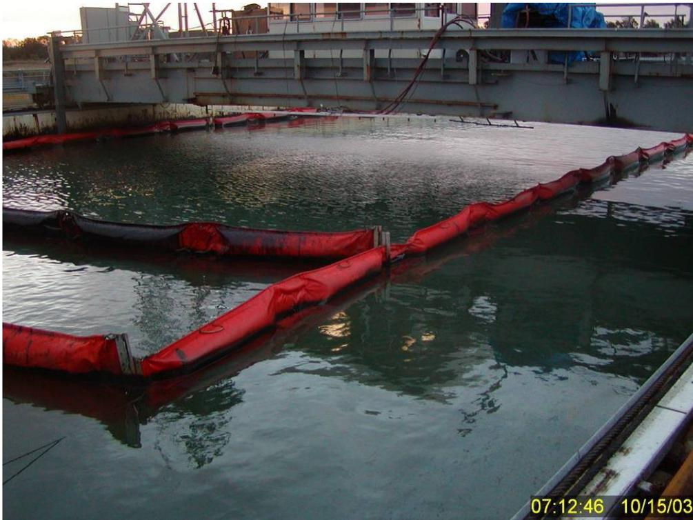
**Figure 164** Undisturbed test tank surface near secondary containment boom and under movable bridge 15 hours after termination of Test No. 16. Note the absence of significant resurfaced oil accumulations like those observed after Test No. 12 (see Figure 56).
