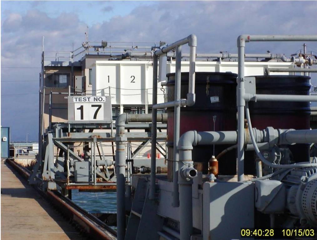
**Figure 178** Completing final preparations for Test No. 17: Lower viscosity IFO 120 fuel oil, Corexit 9500 (nominal DOR 1:50), and low wave energy (30 cpm).
