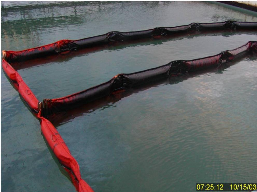
**Figure 171** Northwestern corners of primary and secondary containment booms 15.5 hours after the termination of wave turbulence at the end of Test No. 16.
