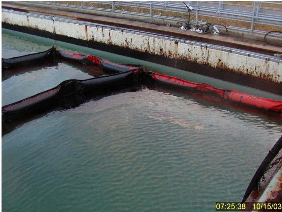
**Figure 172** Residual oil from within the experimental test area that had resurfaced overnight and been blown by the southwesterly wind into northeastern corner of primary containment boom.
