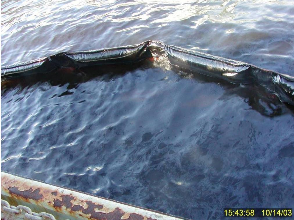
**Figure 148** Silver oil sheen and small patch of residual surface oil adjacent to the primary containment boom 25 minutes into Test No. 16.
