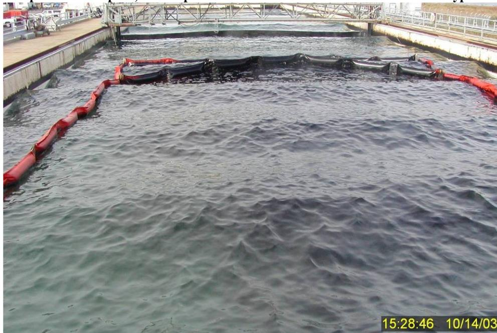
**Figure 140** Overview of subsurface dispersed oil plume in center of the tank ten minutes after treatment in Test No. 16. Note the lack of any whitecaps at this wave frequency setting and the gradual lateral spread (diffusion) of the black subsurface oil outside the containment boom on the western (left) side of the tank. Compare the water color to Figures 132 and 133.
