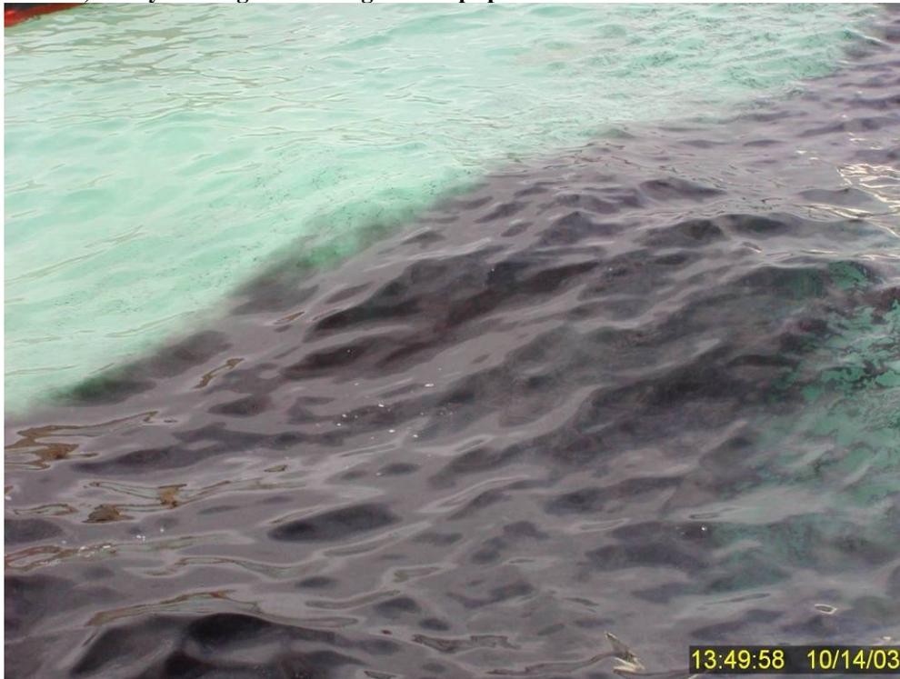
**Figure 104** Close up of oil and water surface four and one-half minutes into Test No. 15 showing the beginning evidence of a fringing subsurface dispersed oil cloud along the upper edge of the slick. Compare the appearance of the oil to that from Figure 80 where no dispersion occurred following a similar time interval after dispersant application but lower wave energy.
