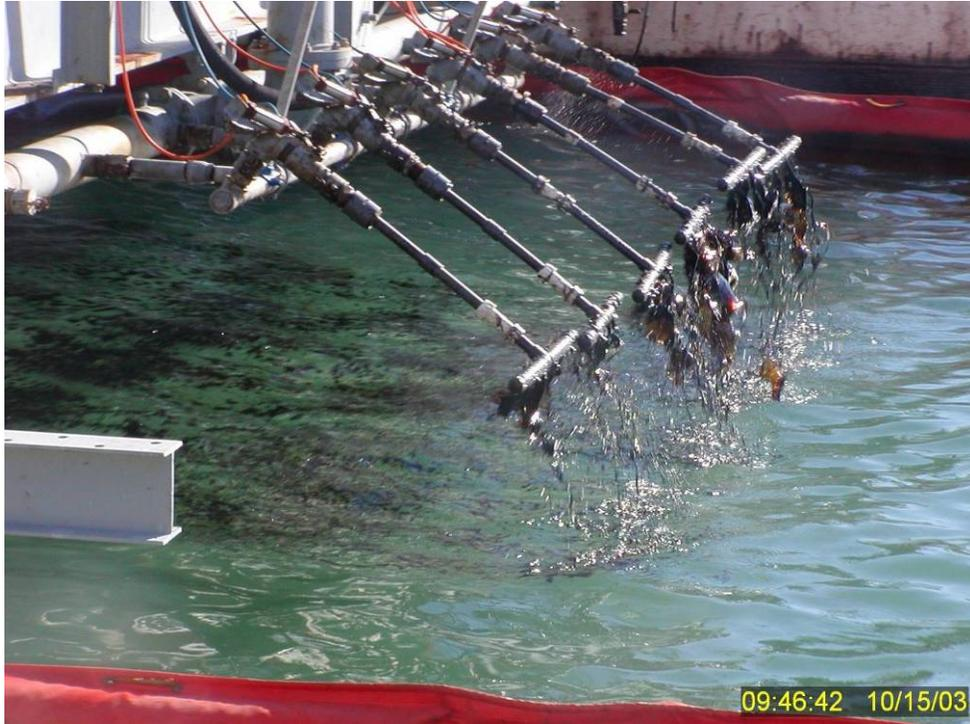
**Figure 180** IFO 120 fuel oil application to water surface at initiation of Test No. 17. Note the lighter, less viscous oil spreads more rapidly than the heavier IFO 180 fuel oil used in earlier tests.
