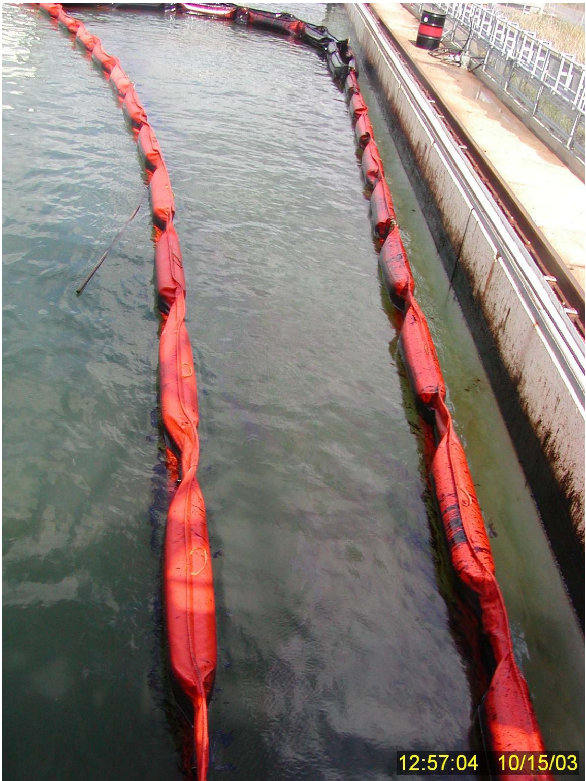
Figure 230 Nondispersed surface oil within newly reopened containment boom along eastern edge of wave tank 17 minutes after the tether line parted and the boom was stabilized for an attempt at oil recovery.
