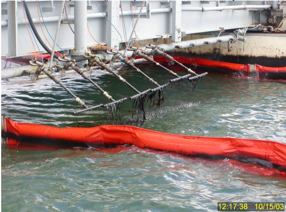
Figure 199 Application of IFO 120 fuel oil to water surface at the initiation of Test No. 18. Note how close the wind has pushed the western edge of the containment boom to the oil application manifold. As noted in the text, these wind conditions were clearly at the edge if not outside the normal operating range for the OHMSETT facility.
