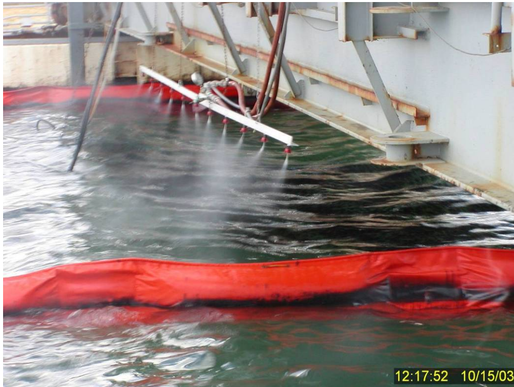
Figure 200 Application of Corexit 9500 to the IFO 120 fuel oil at the initiation of Test No. 18. Note that this lighter, less viscous oil spreads out to make a more uniform target for the dispersant spray, but much of the dispersant was carried away by the wind.
