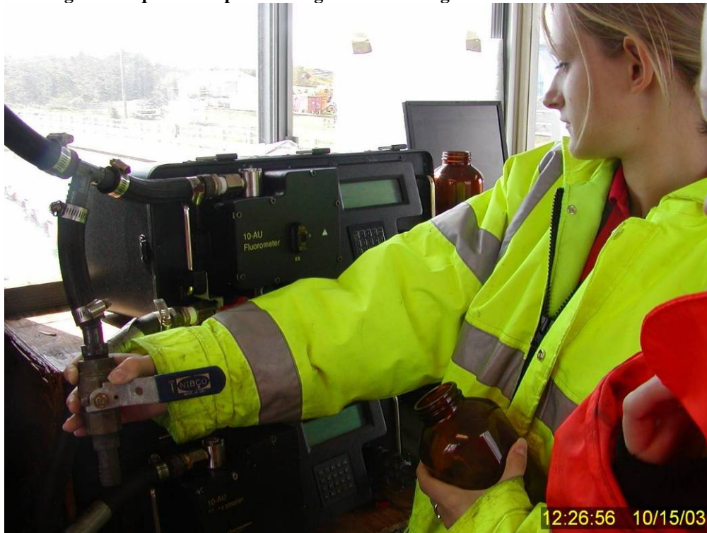
Figure 208 Preparing to collect a discrete water sample from the 1-meter Turner AU-10 fluorometer effluent during a fluorescence peak.
