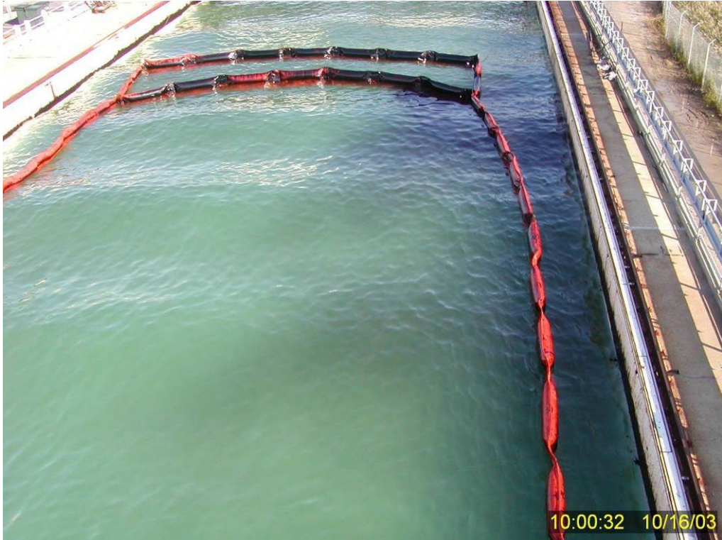
Figure 264 Slightly enhanced dispersion of IFO 180 fuel oil caused by localized turbulence adjacent to the primary and secondary containment booms ~22 minutes into Test No. 19.
