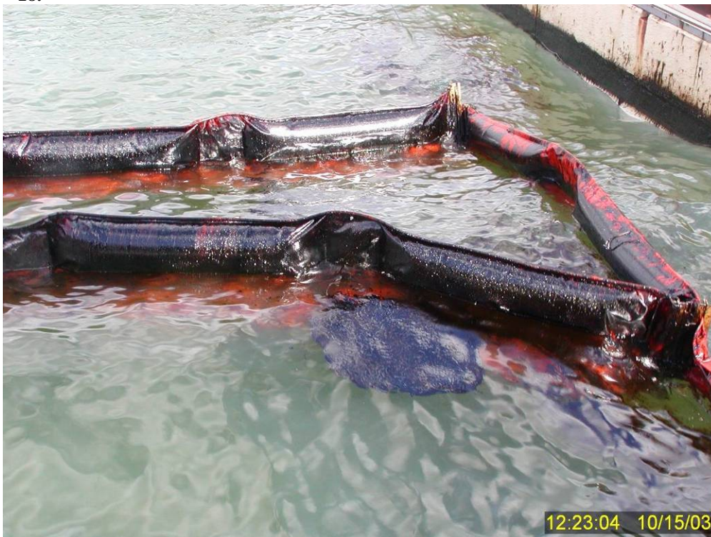
Figure 206 Minor amount of non-dispersed surface oil observed in the northeast corner of the primary containment boom approximately 5 minutes into Test No. 18.
