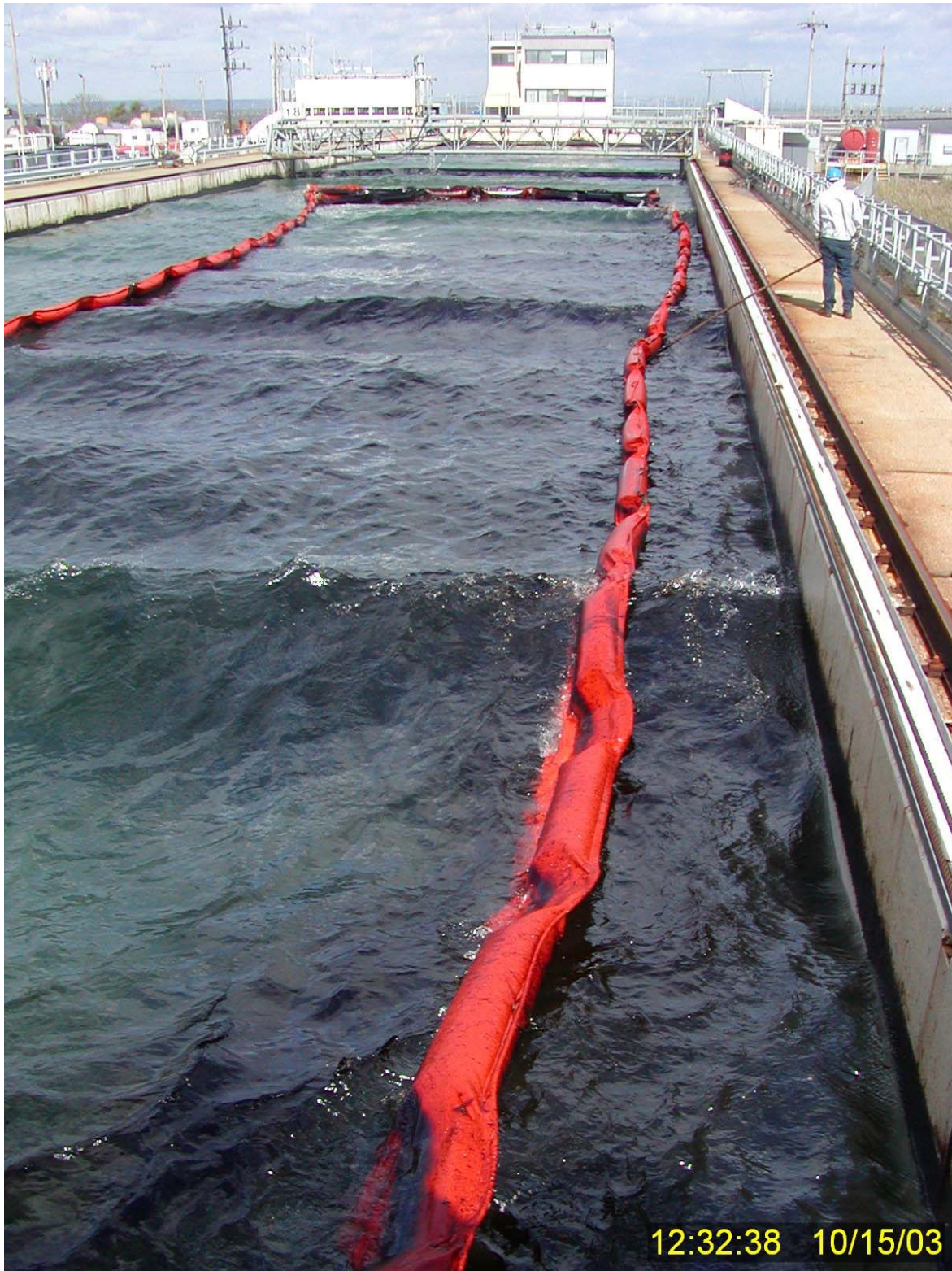
Figure 212 Dispersed oil plume in the center of the tank and along the eastern containment boom 15 minutes into Test No. 18. Note there is very little undispersed surface oil visible in this section of the test tank.
