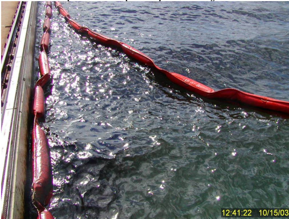
Figure 220 Collapsing containment boom passing over dispersed oil plume and possibly sweeping some residual nondispersed surface oil before it ~ 25 minutes into Test No. 18.
