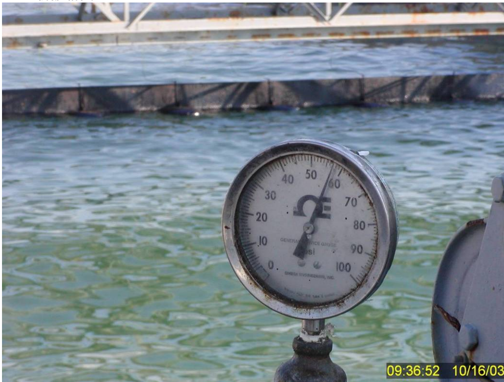
Figure 255 Dispersant control unit pressure guage (reading 57-58 psi on the recirculating plumbing shown in Figure 251) just before initiation of Test No. 19 where a nominal DOR of 1:25 was desired.
