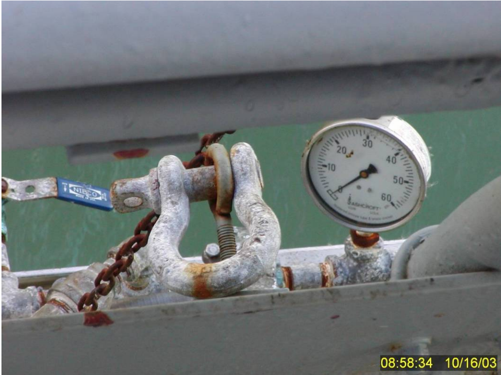
Figure 246 Pressure gauge mounted on the dispersant spray bar to measure dispersant pressure immediately before application.
