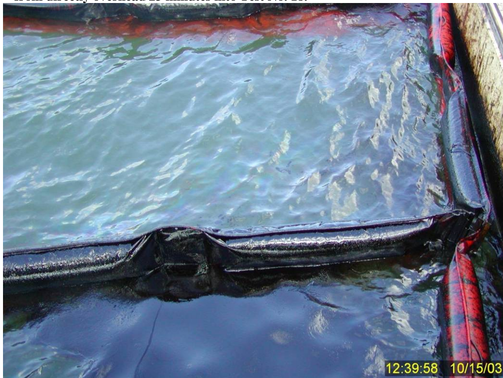
Figure 218 Undispersed surface oil in northeast corner of primary containment boom and relatively oil-free water in secondary containment boom showing little or no splash-over (top of the photograph) 23 minutes into Test No. 18.
