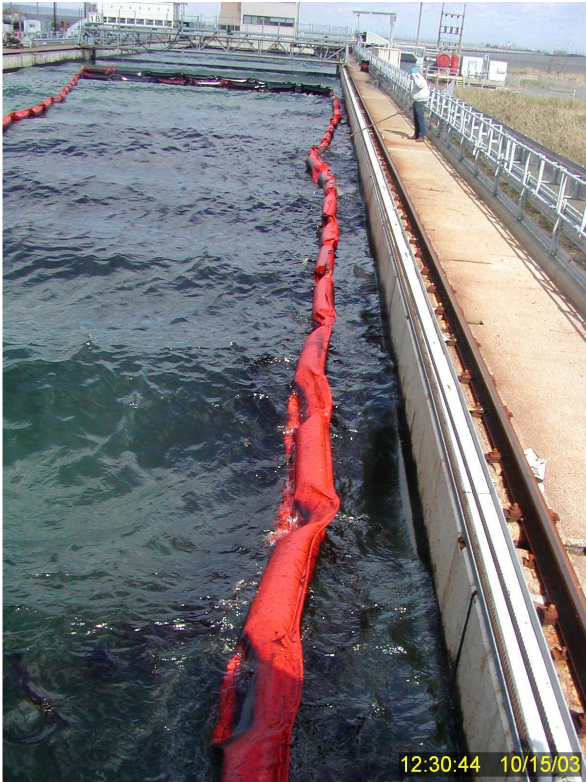
Figure 211 Dispersed oil plume in the center of the tank and along the eastern containment boom 13 minutes into Test No. 18.
