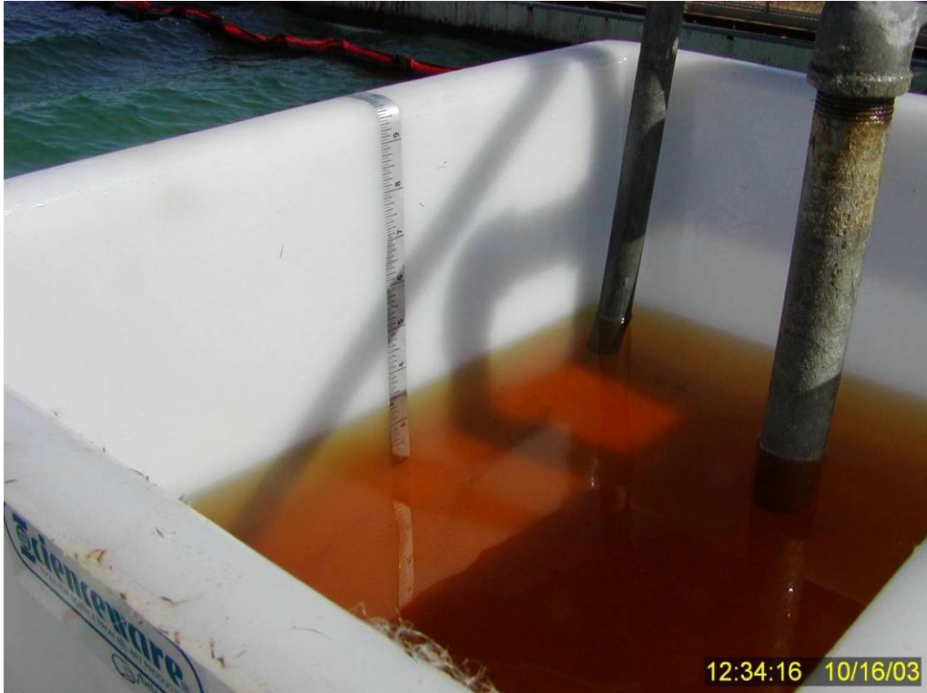
Figure 252 Tape measure used for dispersant volume measurements before and after each test.
