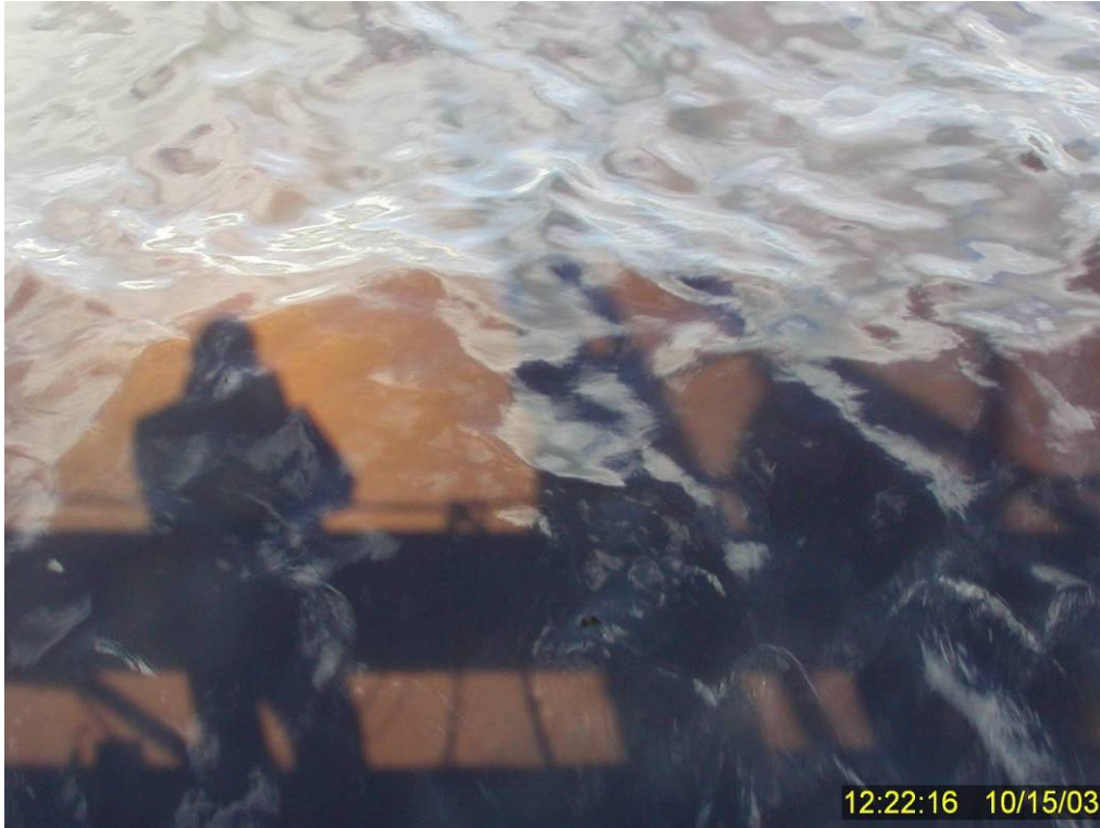
Figure 205 Overhead photograph of classic light-brown dispersed oil plume directly under the movable bridge in the center of the tank approximately 5 minutes after dispersant application in Test No. 18.
