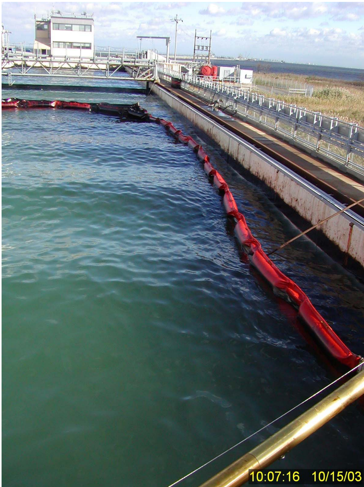
Figure 189 Subsurface dispersed oil plume along eastern containment boom 20 minutes into Test No. 17.
