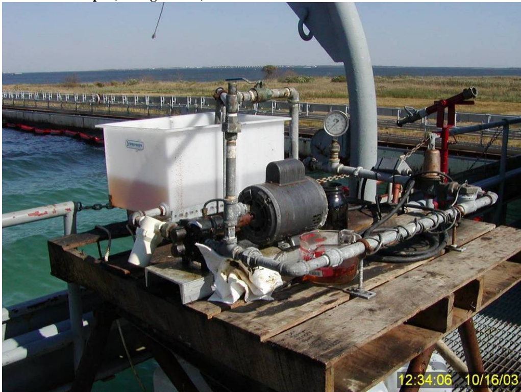
Figure 251 Dispersant spray control unit with Superdispersant SD 25 in the Nalgene reservoir.
