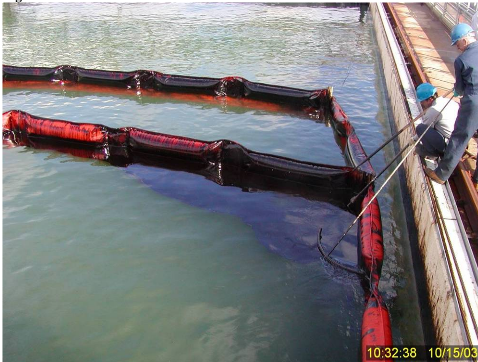
Figure 195 Additional oil collected after sweeping the test area with the fire monitors in preparation for quantitative recovery at the end of Test No. 17.
