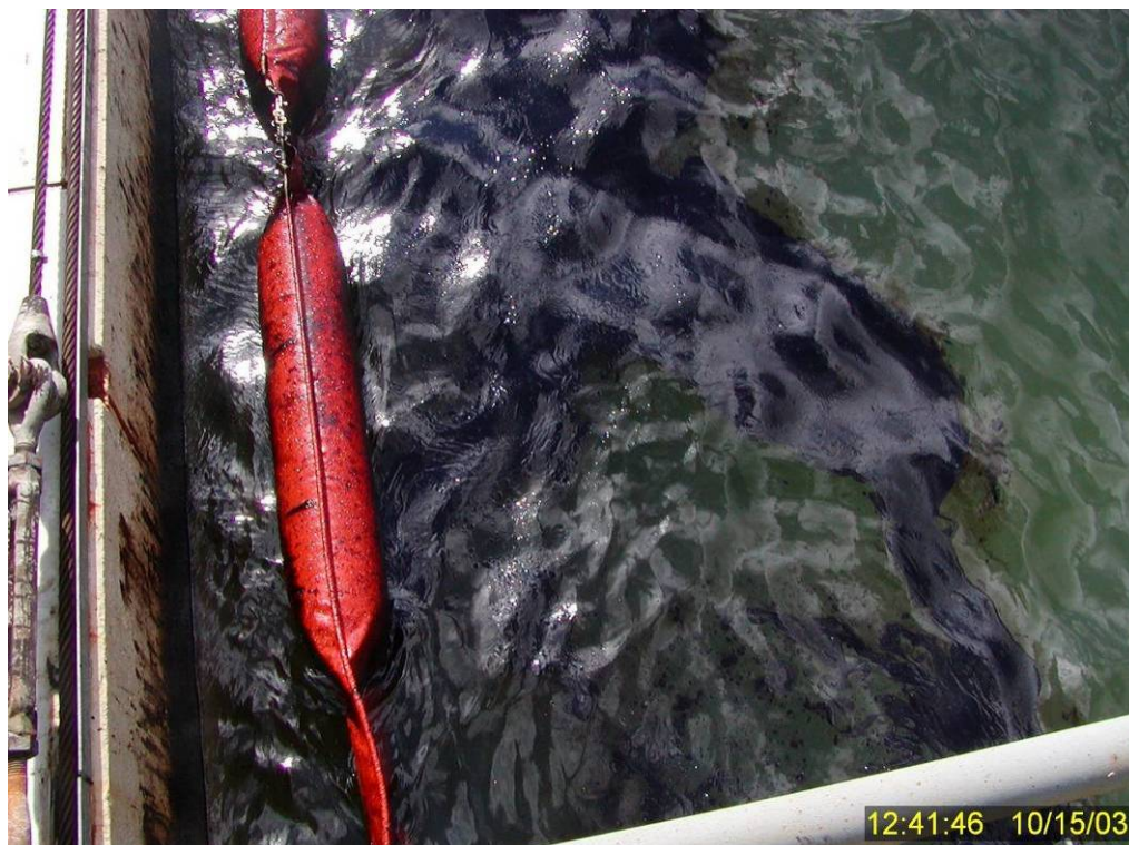
Figure 221 Residual nondispersed surface oil adjacent to the containment boom against the eastern tank wall 25 minutes into Test No. 18.
