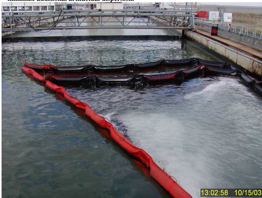
Figure 232 Residual nondispersed surface oil being herded into the northern end of the primary and secondary containment zones 22 minutes after the test was aborted due to the boom failure towards the end of Test No. 18.
