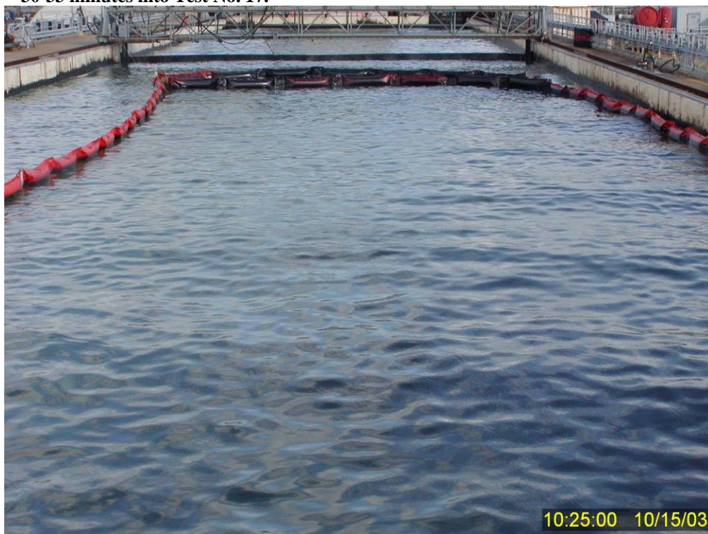
Figure 193 Tank surface photographed at the termination of Test No. 17 before using the fire monitors to sweep any remaining non-dispersed surface oil into the northeast corner (top of figure) for collection.
