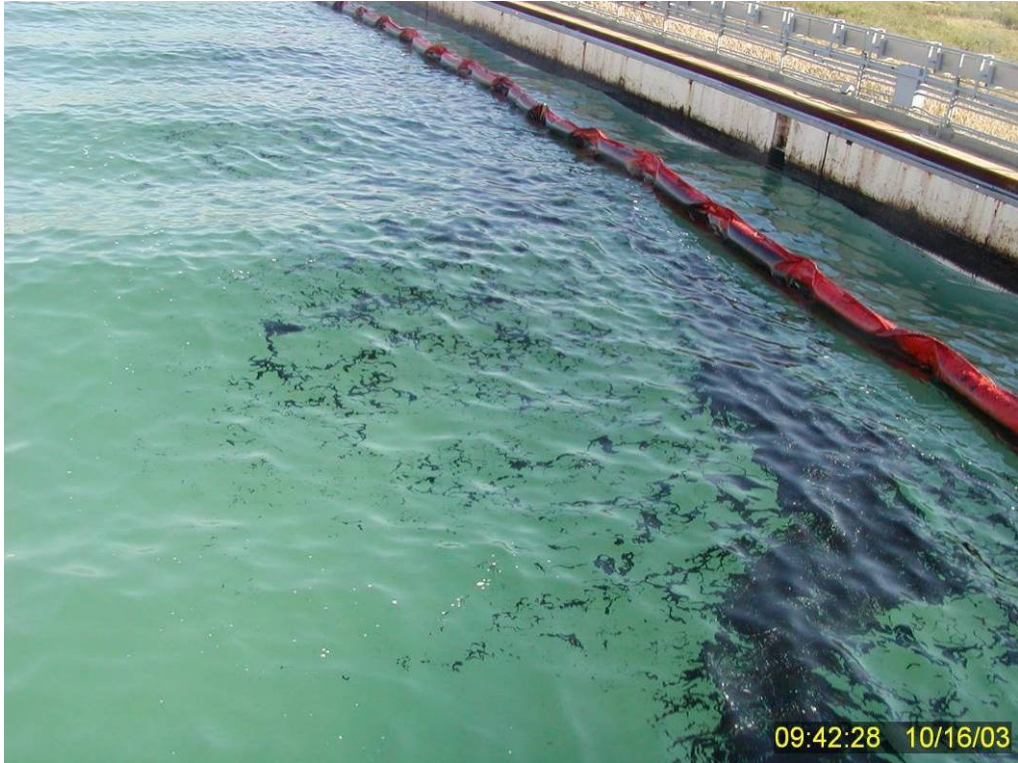
Figure 258 Appearance of the surface IFO 180 fuel oil four minutes after dispersant application in Test No. 19. Note the complete lack of any dispersion under these low-energy conditions despite the higher nominal DOR of 1:25.
