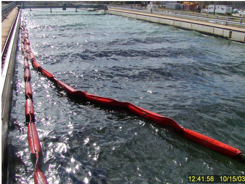
Figure 223 Western containment boom slowly drifting to the eastern tank wall (from right to left) approximately 25 minutes into Test No. 18 (about two minutes after the tether line separated). Note the two sides of the boom converging at the top of the figure (compare to Figure No. 219).
