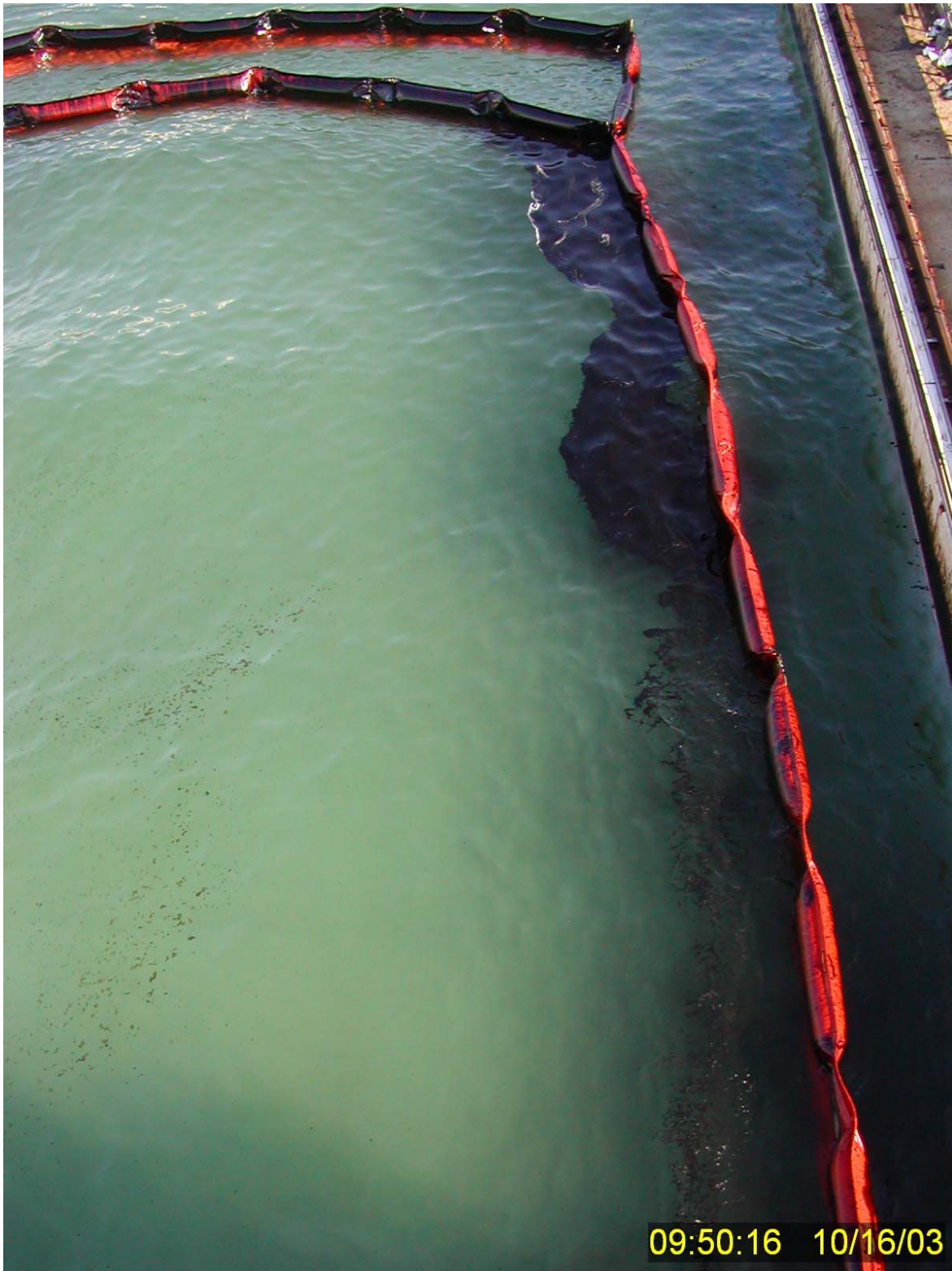
Figure 262 Nondispersed surface oil accumulating along the eastern containment boom ~12 minutes after dispersant application in Test No. 19. Photographed from the observation platform 15 feet above the movable bridge looking from the south to the north (toward the secondary containment boom). Note there is still little or no evidence of any significant chemically-enhanced dispersion.
