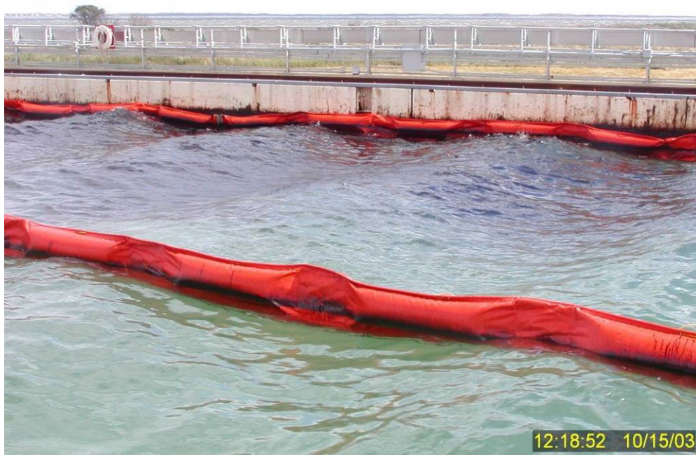
Figure 201 Appearance of treated IFO 120 fuel oil as photographed from the side of the wave tank one minute after Test No. 18 dispersant application. Despite the lack of any white caps or cresting waves, much of the oil has already been dispersed into the water column.
