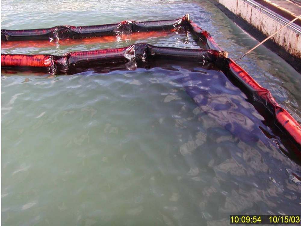
Figure 190 Residual non-dispersed surface oil that had collected in the northeast corner of the containment boom 22 minutes into Test No. 17.
