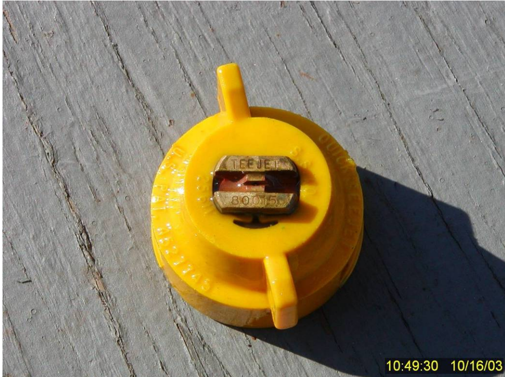
Figure 250 Close up of one of eleven UniJet Model 80015 flat spray nozzles used to deliver a nominal DOR of 1:25 at 60 psi (see Figure 247).
