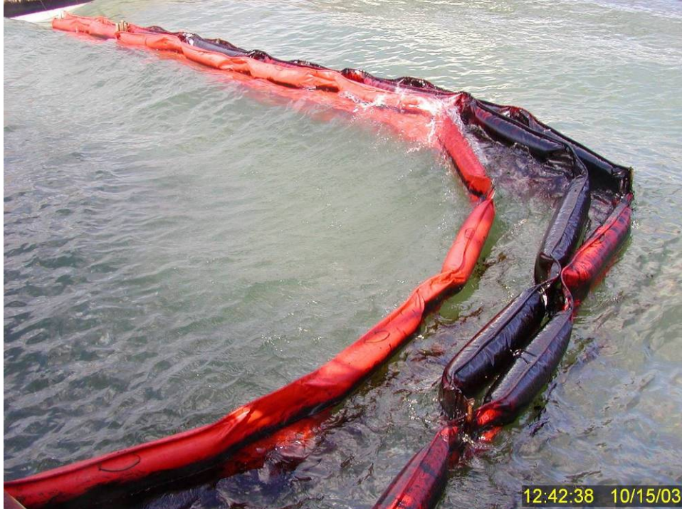
Figure 224 Primary and secondary containment boom collapsing near north end of wave tank two and one-half minutes after the tether line broke at approximately 12:40 hrs. By this time, the wave generator had been turned off, but it took several minutes for the waves to dampen within the tank.
