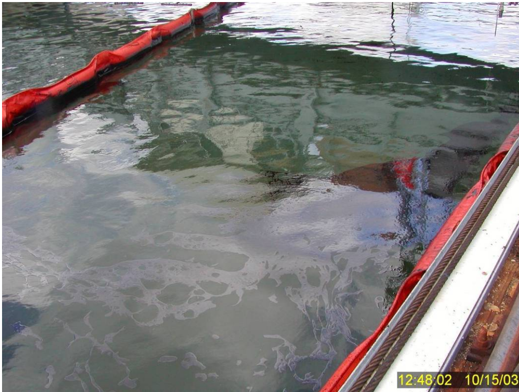
Figure 228 Nondispersed surface oil between reopened containment boom segments under the movable bridge eight minutes after the tether line had separated.
