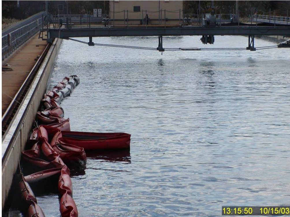
Figure 237 Close up of collapsed boom that no doubt trapped additional nondispersed surface oil that could not be collected and quantified at the end of Test No. 18.
