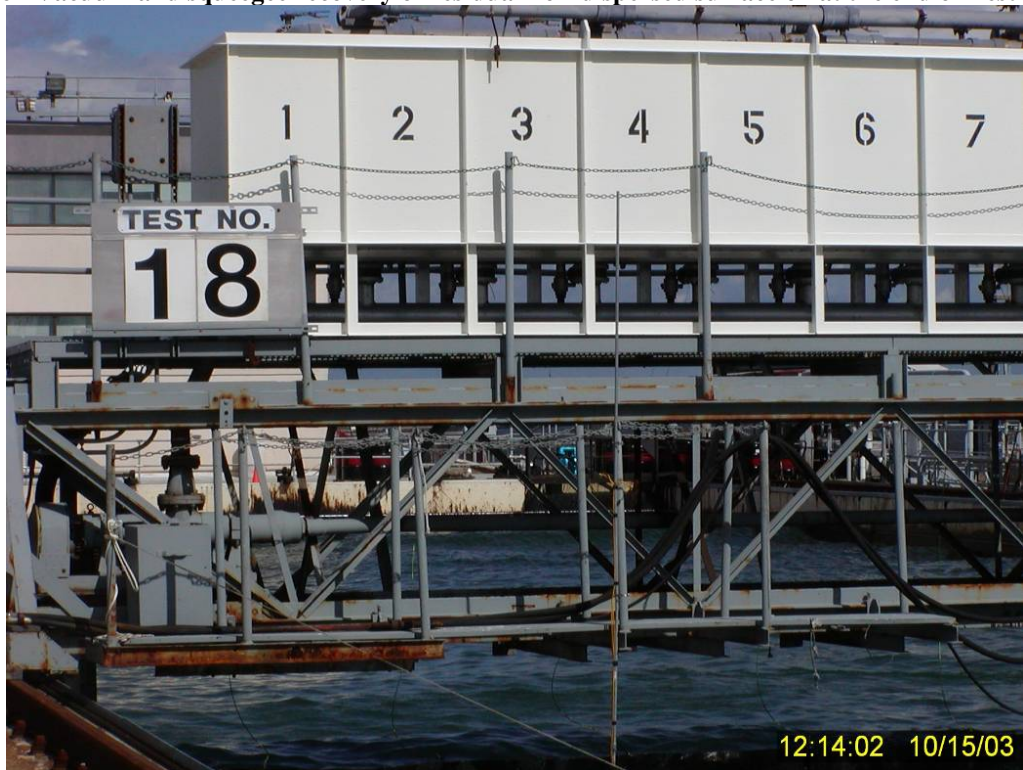
Figure 197 Completing final preparations for Test No. 18: IFO 120 fuel oil, Corexit 9500 (nominal DOR 1:50), and intermediate wave energy (33.3 cpm).
