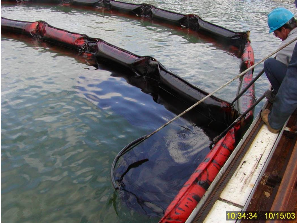
Figure 196 Vacuum and squeegee recovery of residual non-dispersed surface oil at the end of Test No. 17.
