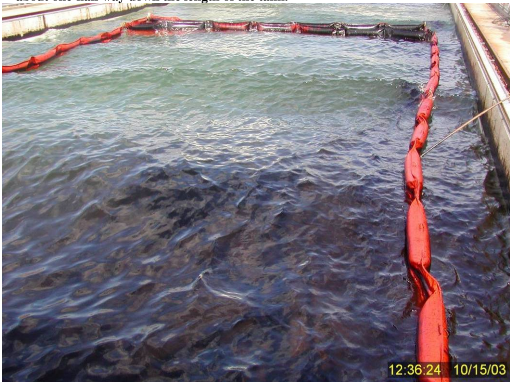
Figure 214 Dispersed oil plume in the center of the tank and along the eastern containment boom approximately 20 minutes after dispersant treatment in Test No. 18.
