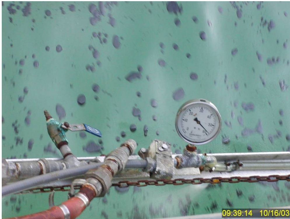
Figure 256 Dispersant pressure measured on the spray bar (57-58 psi) during dispersant application at the initiation of Test No. 19. Note the uneven distribution of oil on the water surface passing beneath the spray resulting in significant under dosing of the slick.
