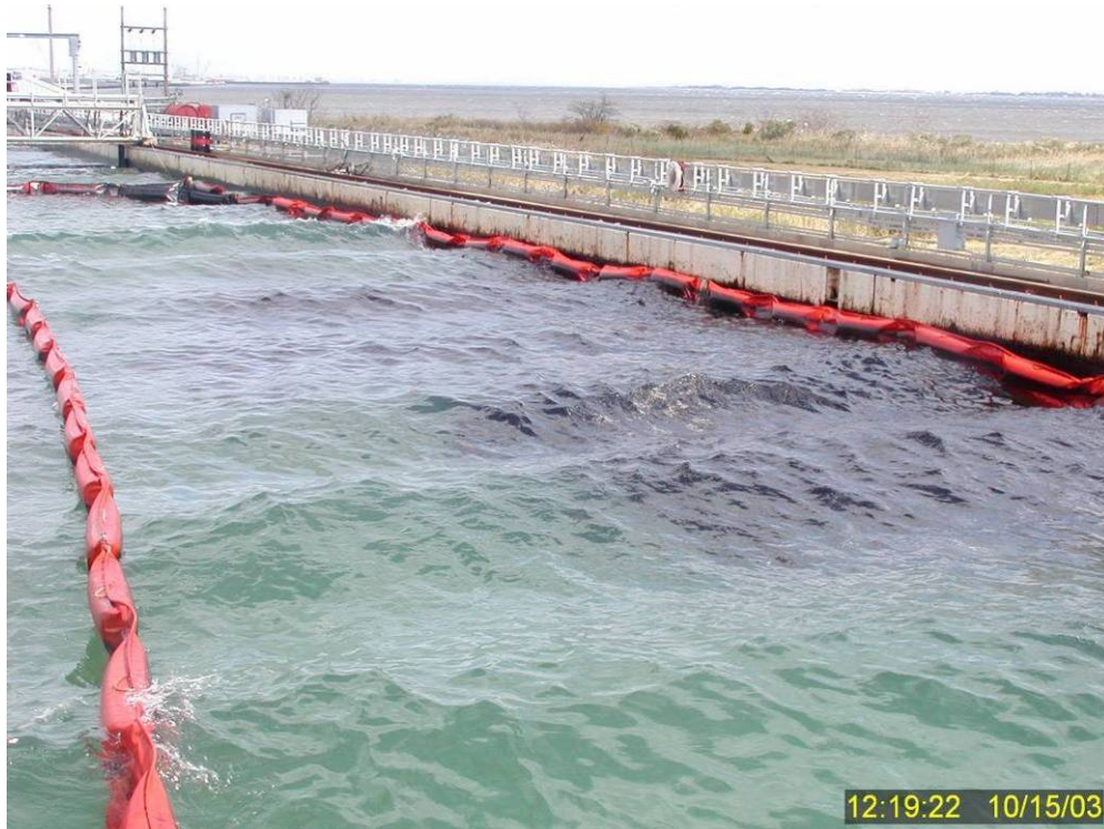
Figure 202 Appearance of the treated IFO 120 approximately two minutes after Test No. 18 dispersant application. Much of the oil has actually been dispersed into the water column where it is no longer subject to the strong cross wind pushing it towards the eastern containment boom along the top of the figure.
