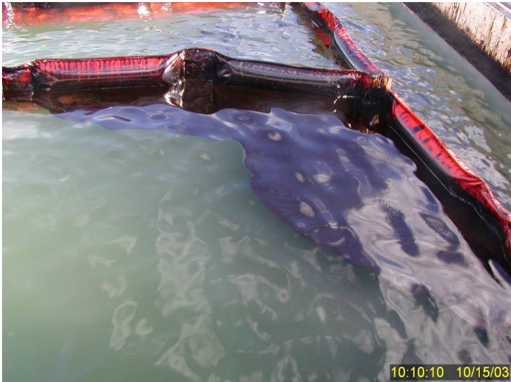
Figure 191 Close up of residual non-dispersed oil in northeast corner of test area showing little or no splash over into the secondary containment boom 23 minutes into Test No. 17.
