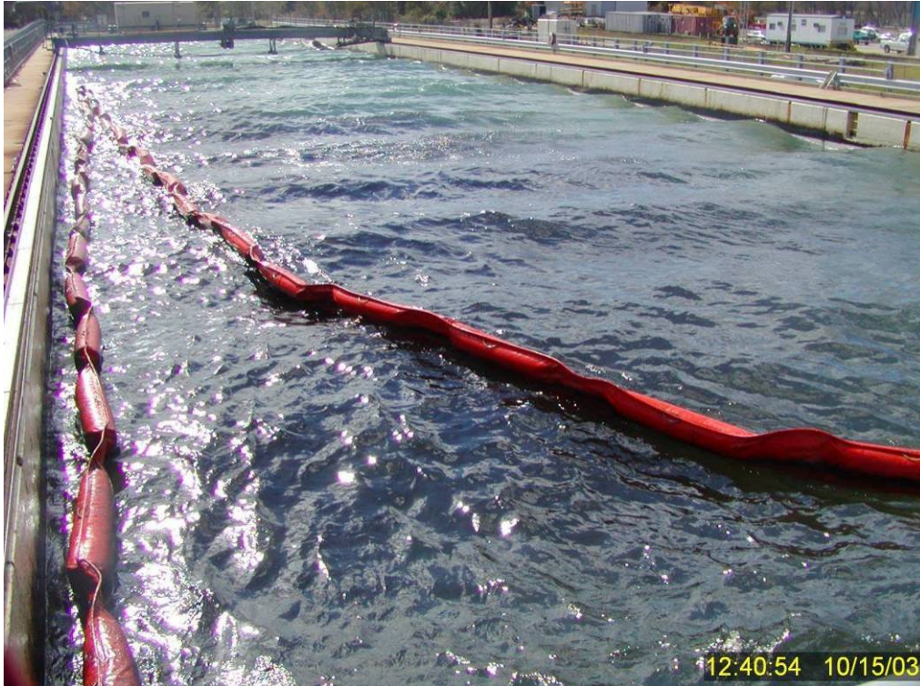
Figure 219 Containment boom after tearing away from the tether in the south west corner of the wave tank 24 minutes into Test No. 18. The boom had been anchored to the bridge shown at the top of the photograph, but the steady 30-35 knot winds from the west (right side of the figure) eventually caused the line to part. Note the dispersed oil plume remaining in the center of the tank.
