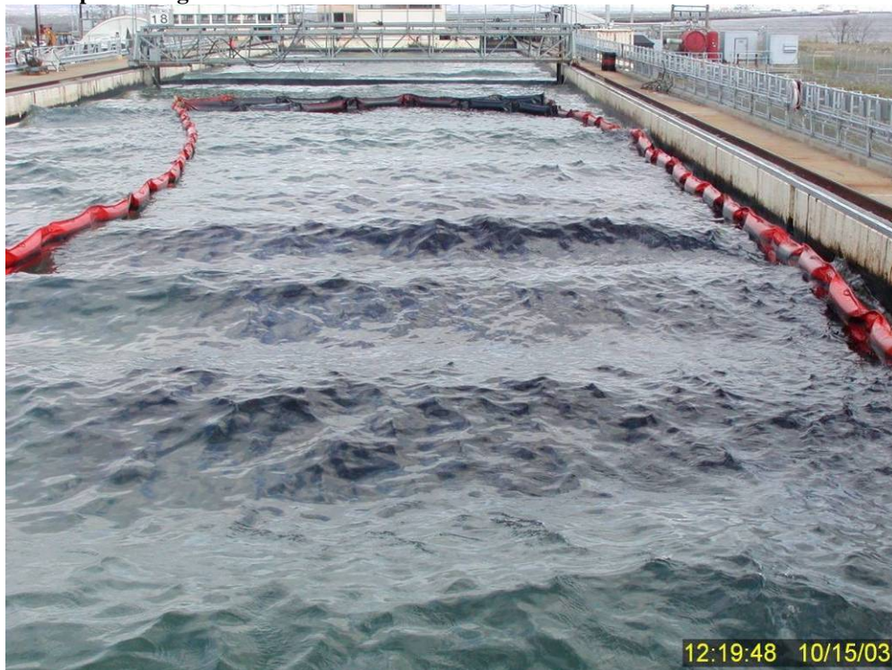
Figure 203 Overhead view of dispersed oil plume in the water column approximately two minutes after dispersant treatment in Test No. 18.
