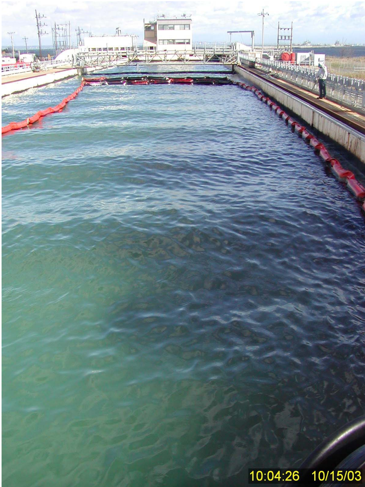
Figure 188 Subsurface dispersed oil plume and almost complete absence of surface oil approximately 17 minutes into Test No. 17 (IFO 120 fuel oil, Corexit 9500 (DOR 1:50), and low energy (30 cpm) waves).
