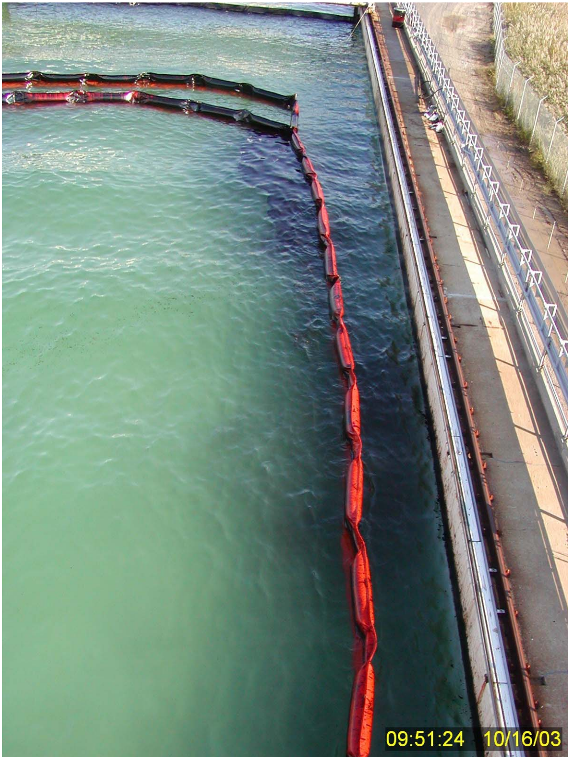
Figure 263 Accumulation of nondispersed surface oil in the northeast corner of the primary containment boom approximately 13 minutes after dispersant application in Test No. 19. At this time, there is just the slightest indication of minor (and anomalous) dispersion due to enhanced turbulence caused by the waves interacting with the containment boom. This is more fully developed after another 10 minutes (as shown in Figures 264 and 265).
