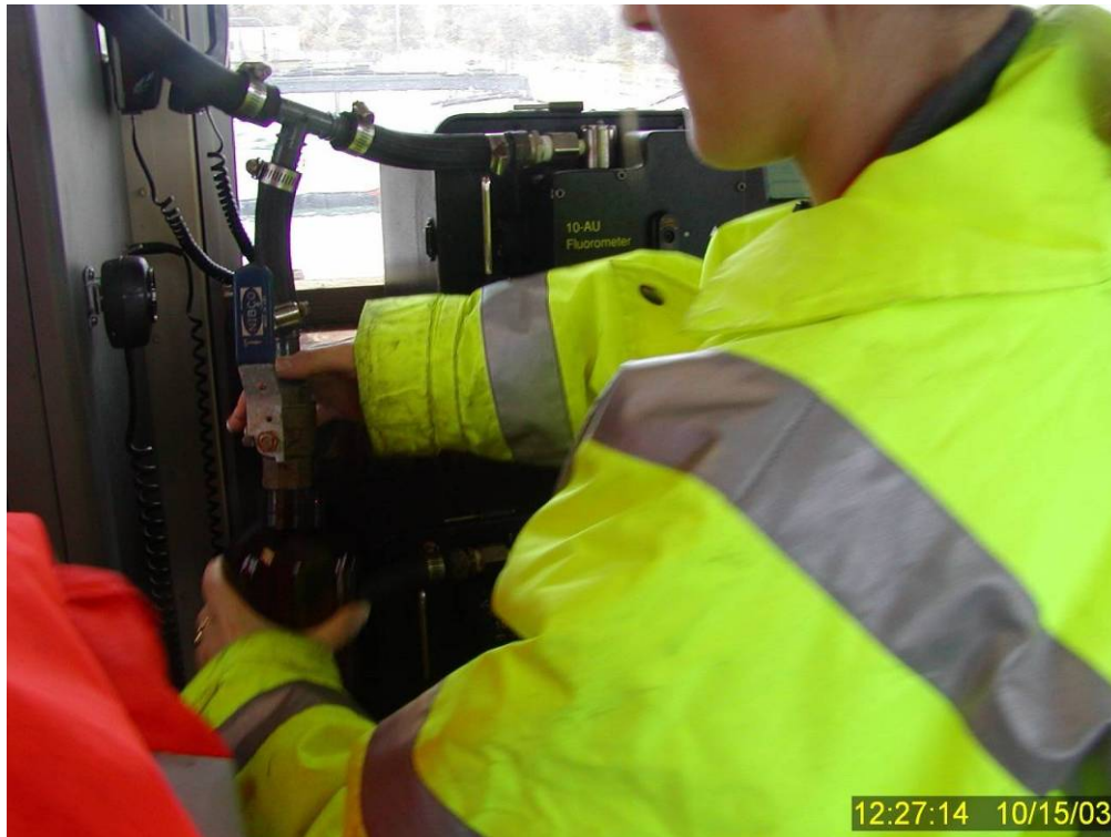
Figure 209 Collecting a discrete grab sample of water from the 1-meter fluorometer effluent during a fluorescence peak maxima.
