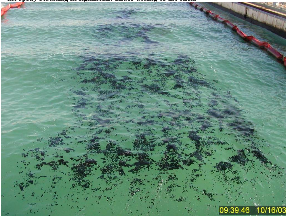
Figure 257 Appearance of the treated IFO 180 fuel oil approximately one minute after dispersant application in Test No. 19.
