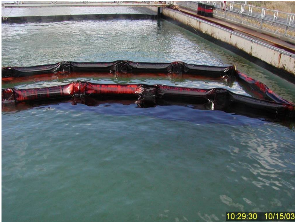
Figure 194 Remaining nondispersed surface oil that had naturally accumulated in the northeast corner of the test enclosure during Test No. 17. From the lack of any surface oil along the eastern containment boom at this time, it is believed that this oil was probably swept along the boom by the wave train during the test, and that it represented the non-dispersed oil photographed in Figures 185 and 186.
