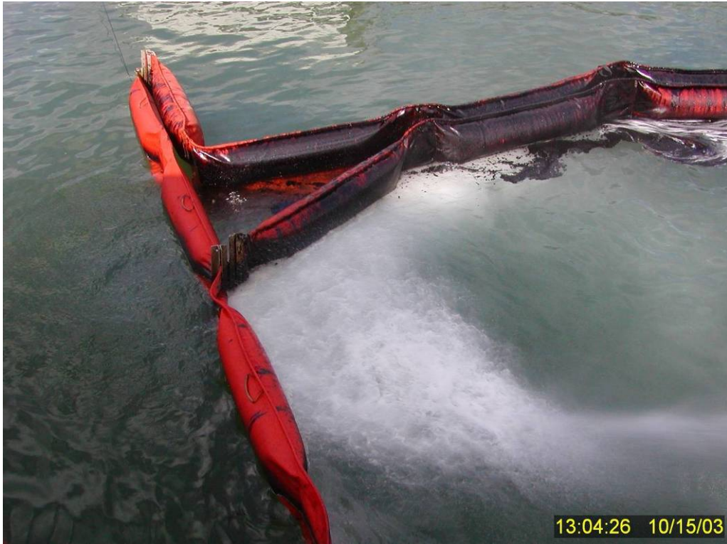
Figure 233 Example of fire monitor spray direction to herd residual surface oil with capillary waves and rising air bubbles in preparation for oil collection effort at the end of aborted Test No. 18.
