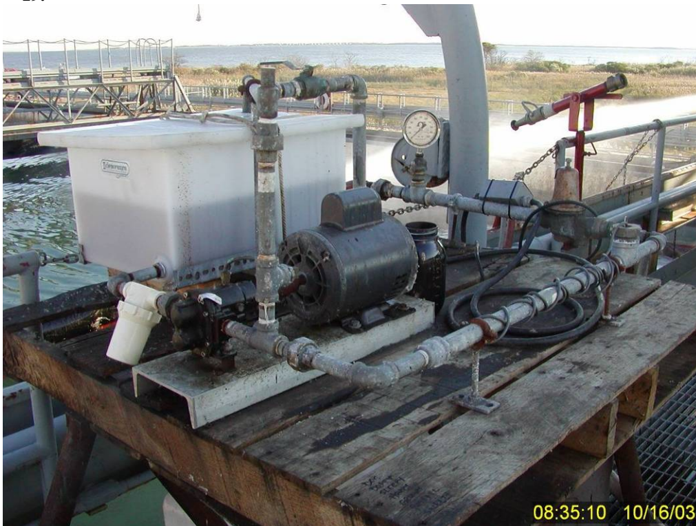
Figure 243 Dispersant control/pumping apparatus. The white Nalgene reservoir holds the dispersant, which is pumped under a specified pressure to the dispersant spray bar mounted beneath the bridge.
