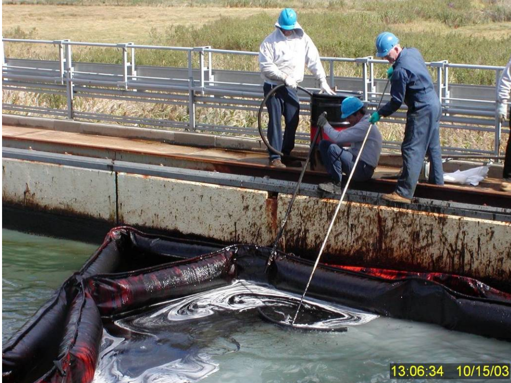
Figure 235 Squeegee and vacuum recovery of residual nondispersed surface oil at the end of aborted Test No. 18.
