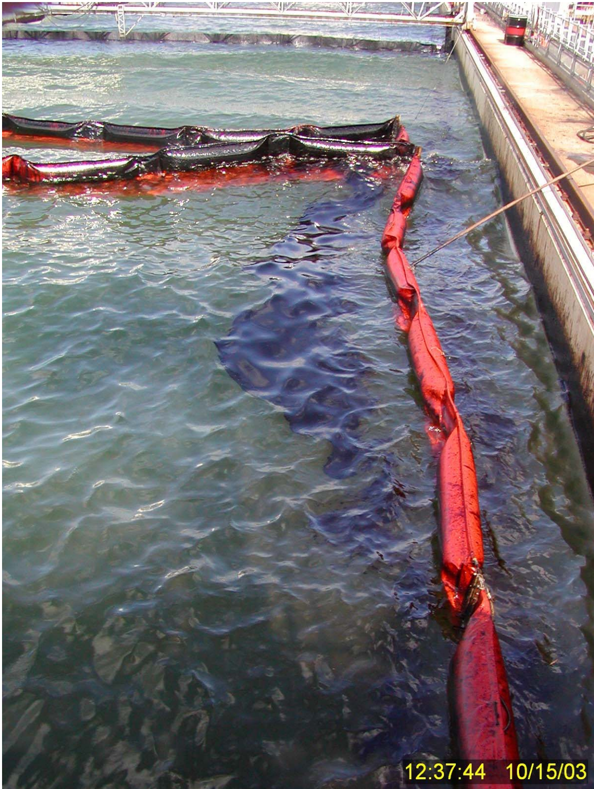
Figure 216 Close up of undispersed surface oil in northeast corner of primary containment boom approximately 20-21 minutes into Test No. 18.
