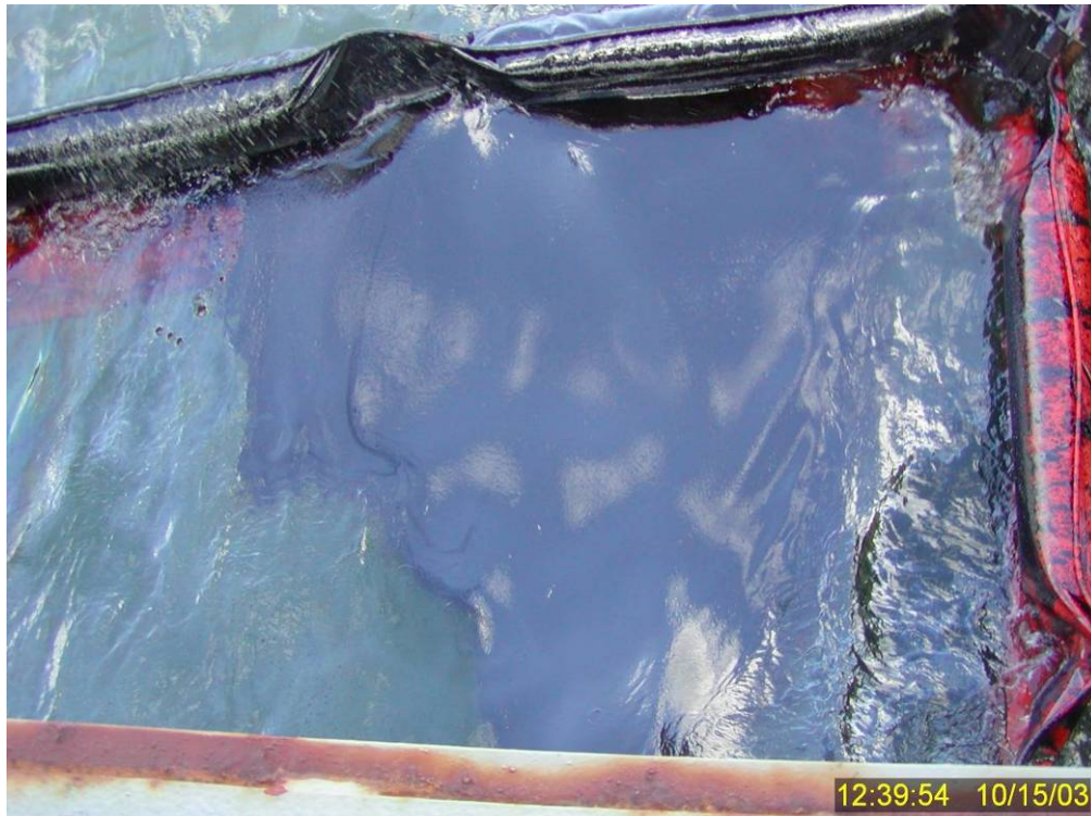
Figure 217 Undispersed surface oil in northeast corner of the primary containment boom photographed from directly overhead 23 minutes into Test No. 18.
