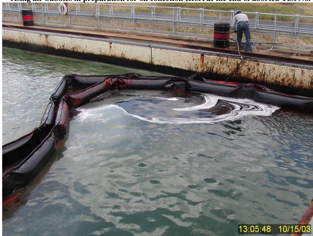
Figure 234 Nondispersed surface oil after being herded into the northeastern corner of the containment boom at the end of aborted Test No. 18.
