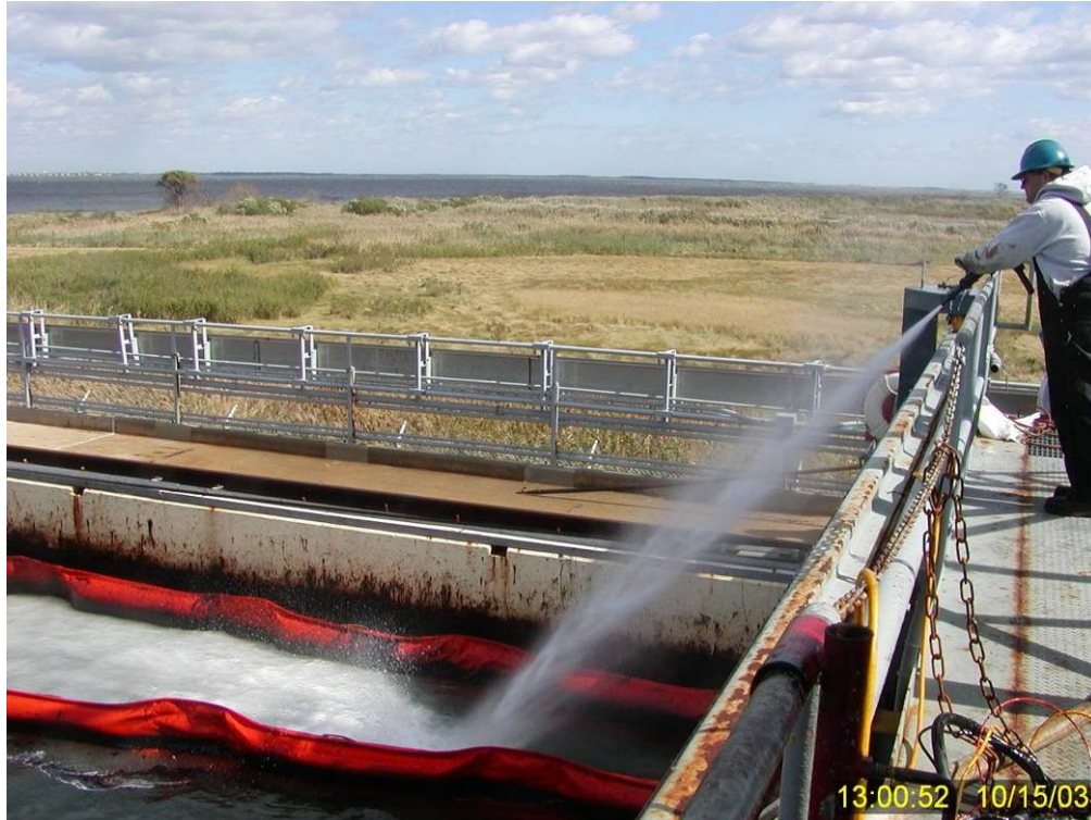
Figure 231 Use of fire monitor to herd residual surface oil to north end of tank for oil recovery. As in previous tests, the water spray was carefully directed to the water surface and not the oil to minimize additional artifactual dispersion.
