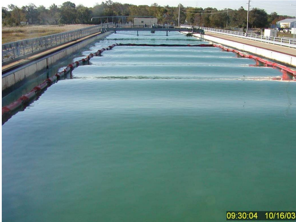
Figure 254 Initiation of wave train just before Test No. 19. These are the first waves coming down the tank at a 30 cpm wave paddle frequency before the desired sea-state was obtained approximately 6-7 minutes later.
