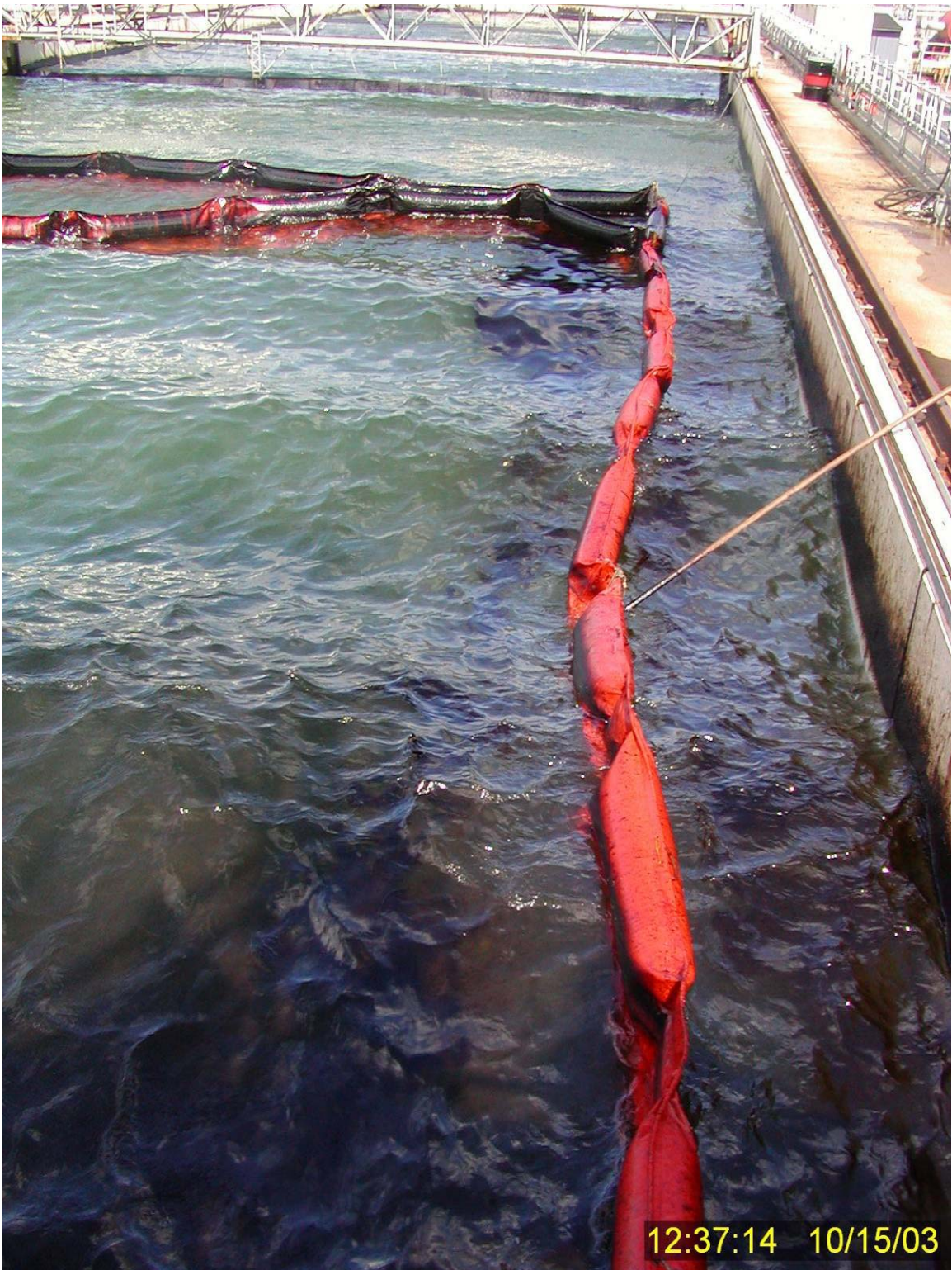
Figure 215 Residual undispersed surface oil accumulating along the north eastern edge of the primary containment boom approximately 21 minutes into Test No. 18.
