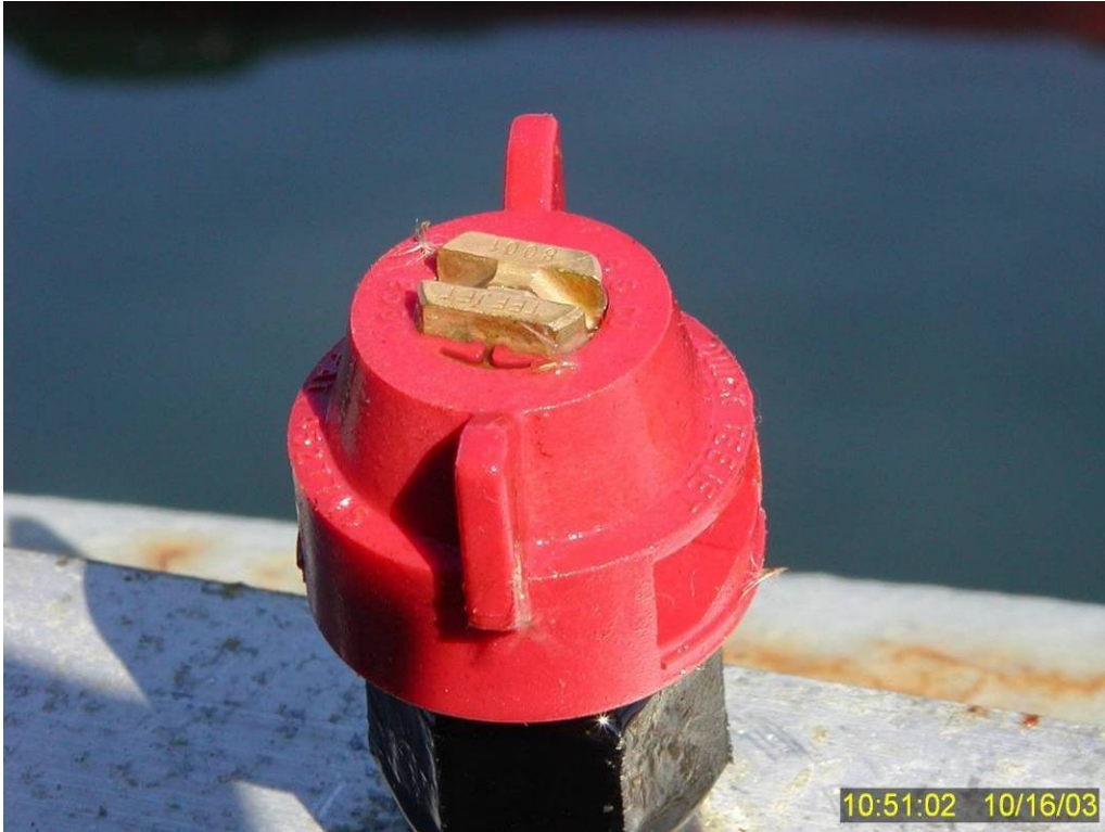
Figure 248 Close up of UniJet Model No. 8001 flat spray nozzle used for the dispersant tests when a nominal DOR of 1:50 was desired.
