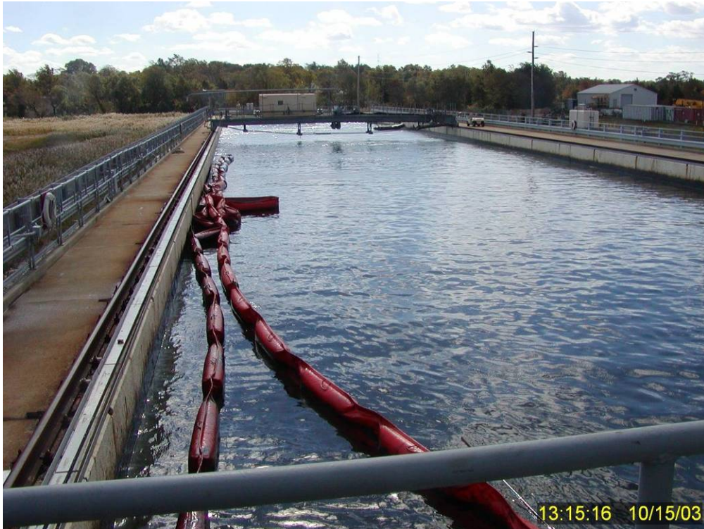
Figure 236 Collapsed containment boom at the southern end of the test tank at the end of aborted Test No. 18. Note, I have no doubt that there was additional nondispersed surface oil trapped within the folds of the boom, so the recovered oil values are probably lower for this test than they otherwise would have been without the boom failure.
