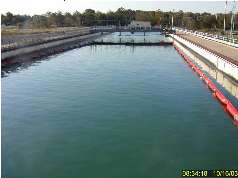
Figure 238 Appearance of the test tank (looking south) after repairing the containment boom that had collapsed the previous afternoon during Test No. 18. Note the dark green color from residual dispersed oil still suspended in the water column 19 hours after the previous test was ended.
