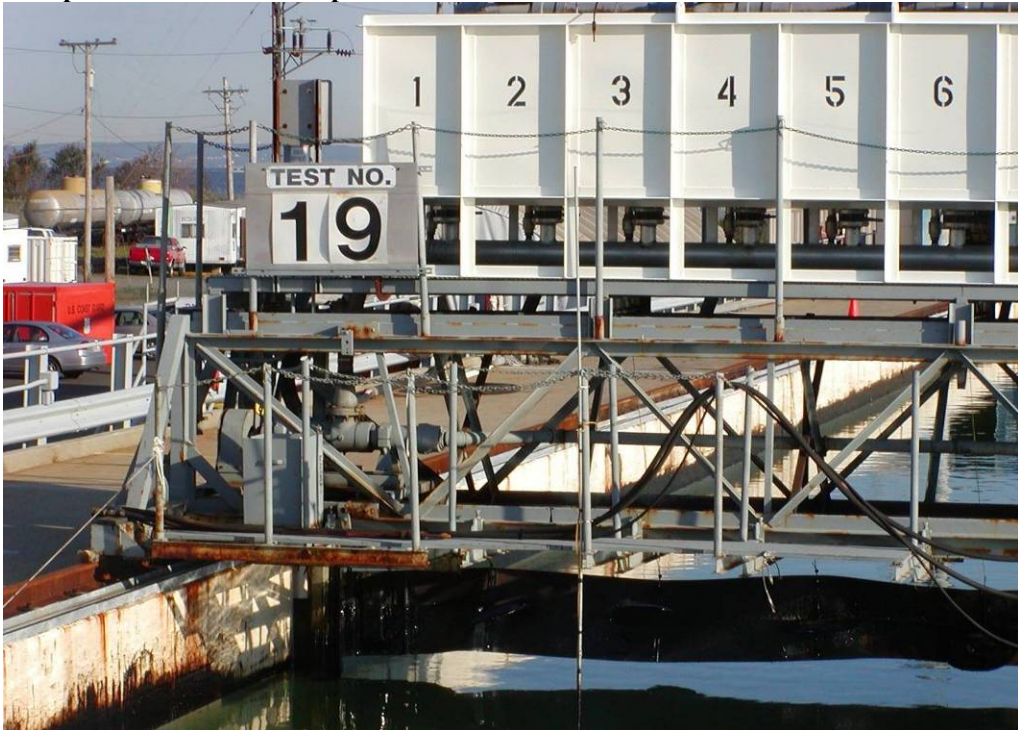
Figure 253 Completion of tank preparations just before Test No. 19: IFO 180 fuel oil plus Corexit 9500 at a nominal DOR of 1:25 and low (30 cpm) energy waves.
