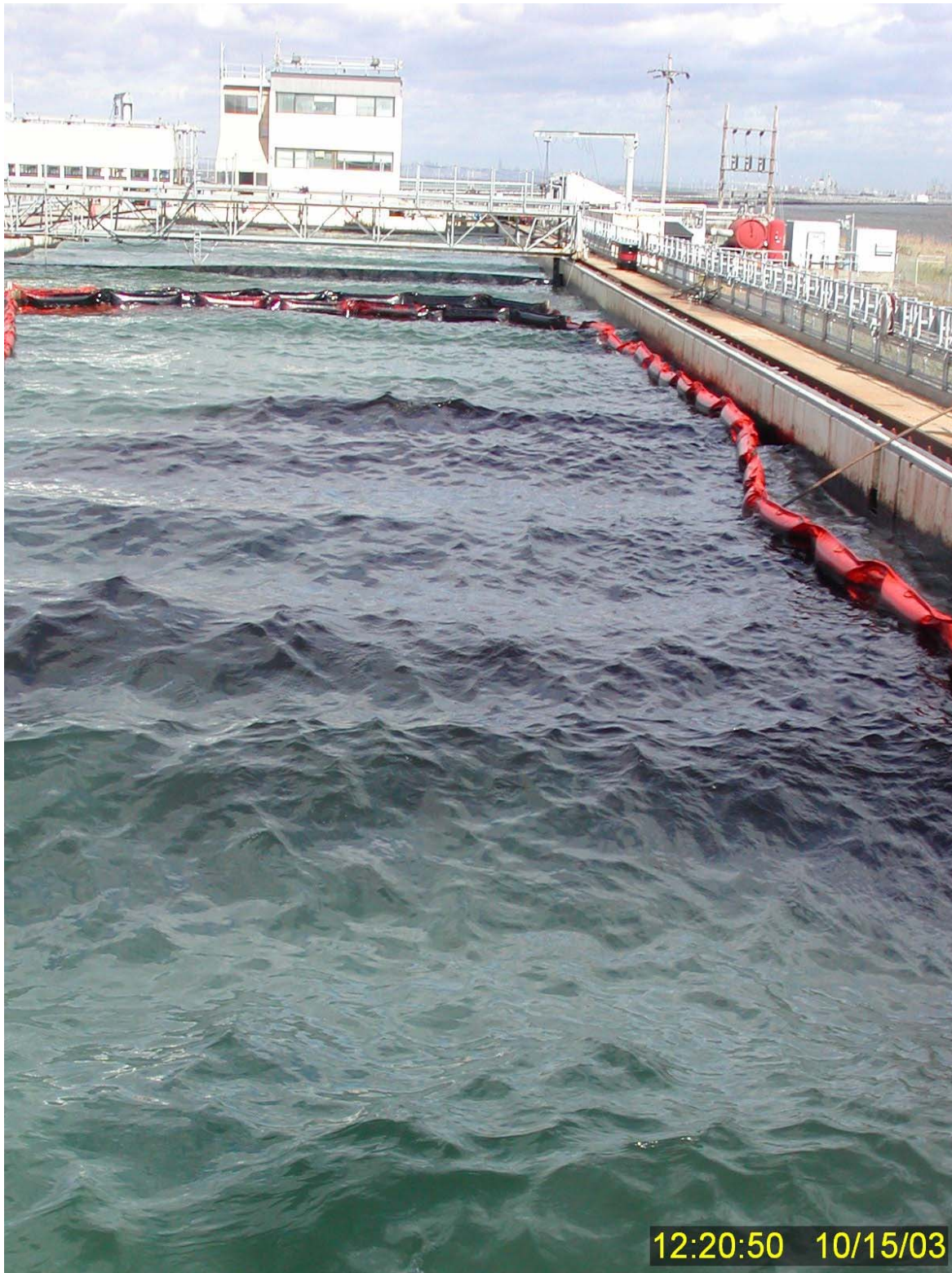
Figure 204 Dispersed oil plume in center of the wave tank approximately three minutes after dispersant treatment in Test No. 18. Note the use of a pole to fend the boom away from the tank wall under these windy conditions.
