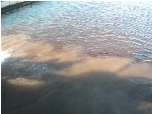
Figure 7 Sweeping Operation. Note that Extensive Re-dispersion is Occurring and Only a Small Amount of Oil is Being Swept in Front of the Water Spray from the Fire Hoses
