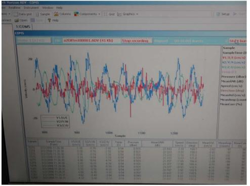
Figure 22 A View of the Screen of the Computer Logging the Acoustic Doppler Velocimeter Output
