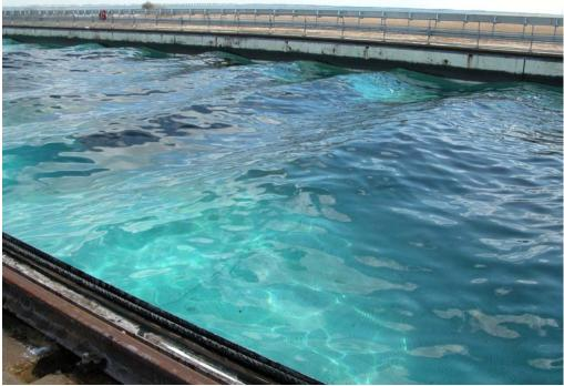
Figure 8 A View of the Second Test Involving Fresh ANS Oil. Note that this Oil Spread Readily Over much of the Tank. Significant Natural Dispersion Was Also Noted.
