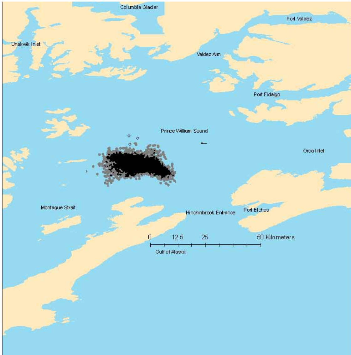
Figure A5: Central Prince William Sound instantaneous release scenario, slick area at 72 hours (GNOME Trajectory)
